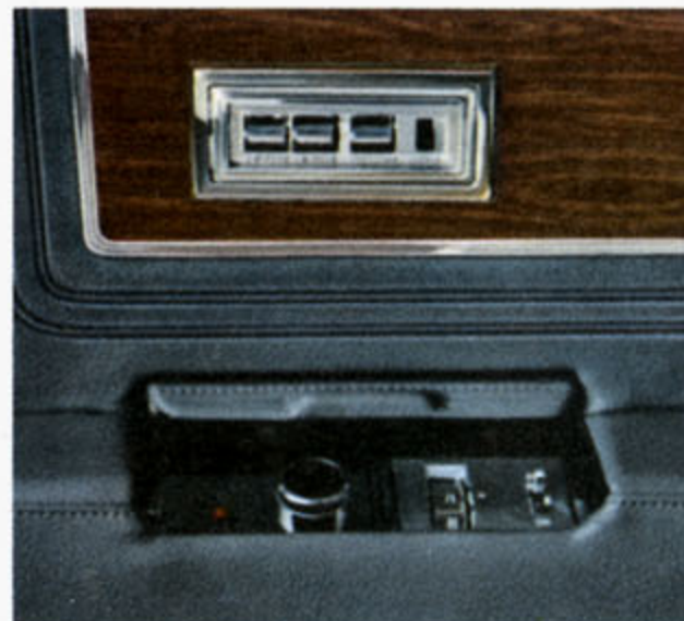
Rear controls in the Limousine, above, permit the occupant to raise or lower the windows, turn on the reading lamps, tune the radio, activate the automatic climate control and raise or lower the glass partition.
