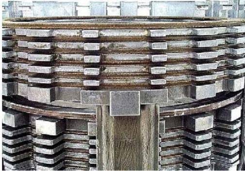
If your drum has the three-piece apply plate assembly, use thin steel clutch plates which measure 0.070" thick, keeping in mind that this version uses an early thin steel with wide teeth at the bottom of the clutch pack.
