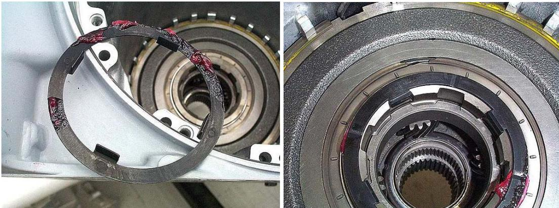
**Step 15:** Install the rear sun gear into the rear planetary carrier.
