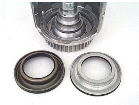
**Step 14:** Remove the forward piston housing inner o-ring from the input drum. All input drum parts are now ready for cleaning and inspection.
