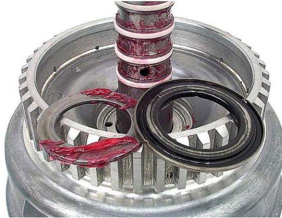
The input drum is now ready for unit assembly. You may want to reinstall the seal ring sizer to keep the seal rings compressed until unit assembly.
