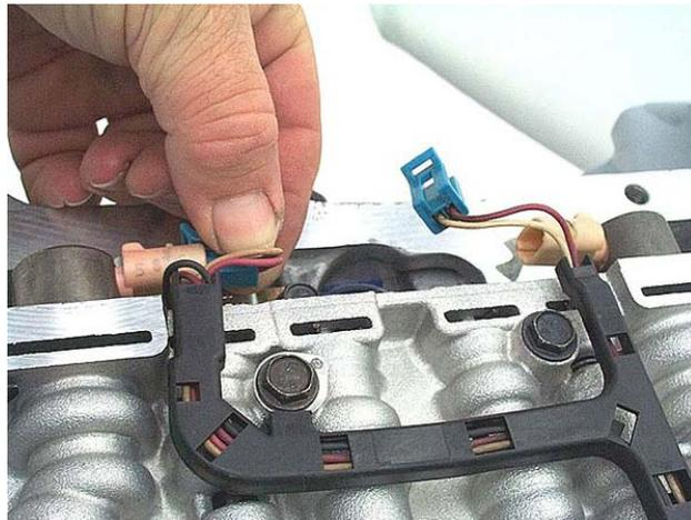
**Step 10:** Remove the manual lever detent spring.
