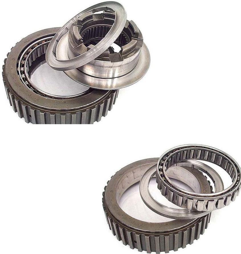
**Step 18:** Use #240 grit emery cloth to break through the glaze on both inner and outer sprag races. Finish both surfaces with #320 grit emery cloth. Thoroughly clean all sprag components.
