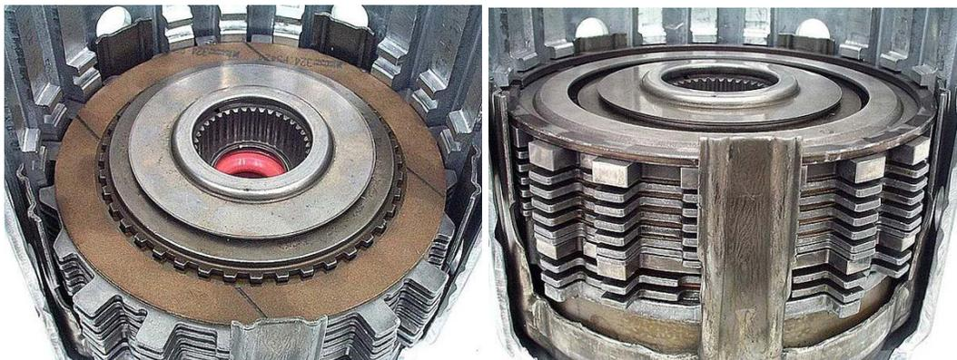
**Step 20:** Install the 3-4 clutch apply plate next. There are two possible types of apply plate setup, and the clutch stack-up is different for each. You will find either a thick one-piece apply plate with built-in feet for the apply ring fingers, or a thin stamped steel plate with feet for the apply ring fingers, with a stamped steel stepped plate on top of it, followed by an early 4L60-style 3-4 clutch steel plate with wide teeth to engage the drum slots.
