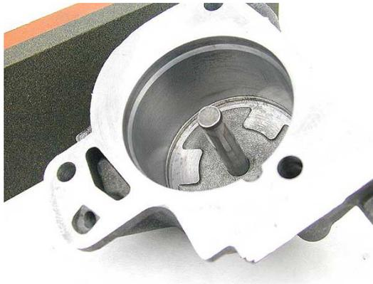
**Step 16:** Place a new seal on the piston. Coat the housing and pin with assembly lube. Install the piston and spring into the housing.
