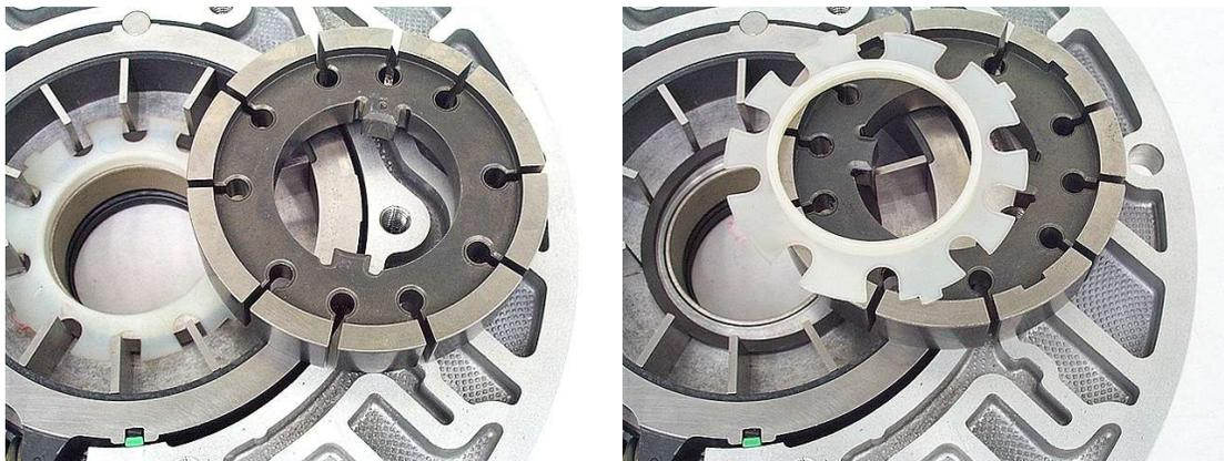
**Step 8:** Remove the pump rotor vanes and bottom vane guide ring.
