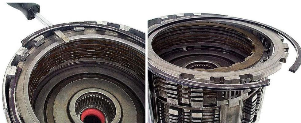
**Step 6:** Remove the 3-4 clutch friction and steel plates. Remove the five boost spring assemblies from the drum if equipped.
