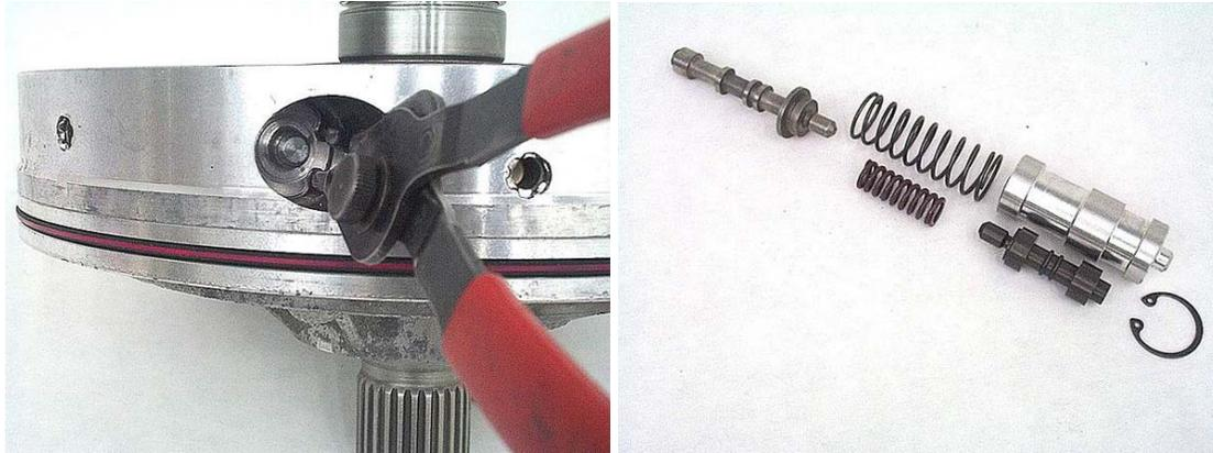
**Step 3:** Remove the TCC apply valve retaining snap ring from the valve bore. The retaining plate, valve and springs should fall out of the bore.
