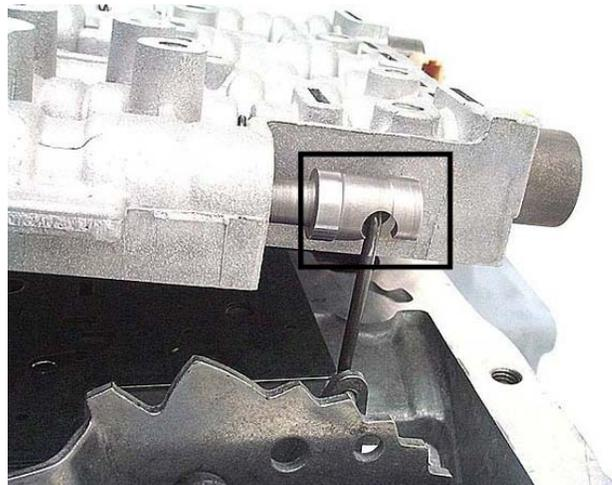
**Step 13:** Remove the seven checkballs from the separator plate.
