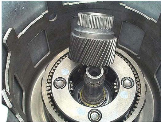
**Step 29:** Hold the output shaft up into the case with one hand while using a pair of small thin snap ring pliers to remove the output shaft snap ring from above the front planet. It may seem a bit like a juggling act, but you don't want the output shaft to hit your toe when you remove the snap ring. It hurts. Once the snap ring is off, slide the output shaft out of the case.
