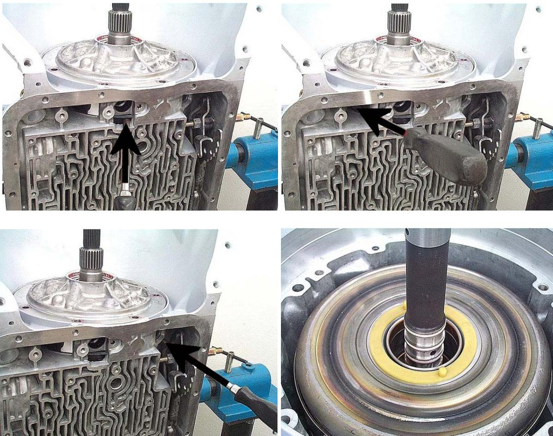
Locate and save the plastic pump-to-reverse input drum thrust washer.
