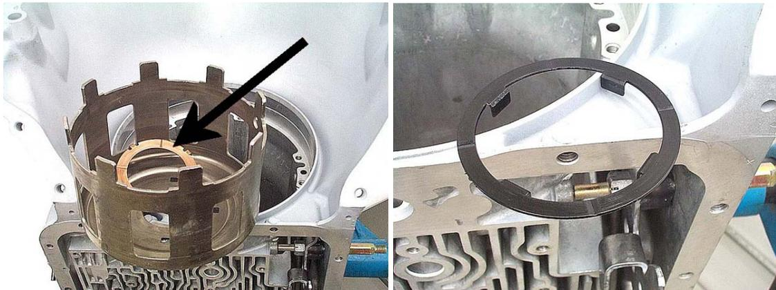
**Step 32:** Remove the rear sun gear from the rear planet.
