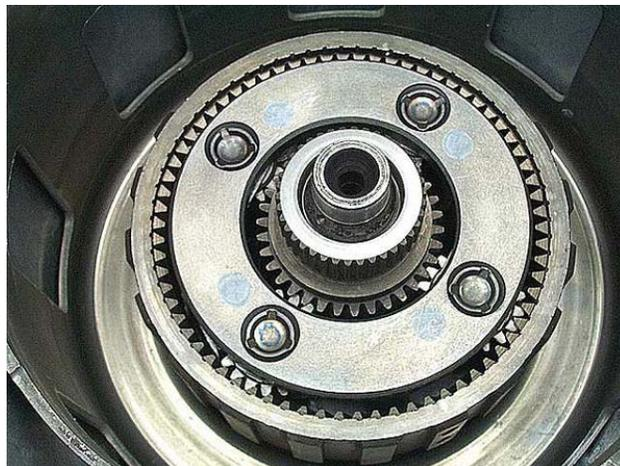
**IMPORTANT-** The following step concerns main unit endplay, which is arguably the most important adjustment to be made in a 4L60E. If this was checked and adjusted during disassembly, and no parts were changed that might change endplay, skip ahead to **Step #25**. Otherwise, proceed to the next step.
