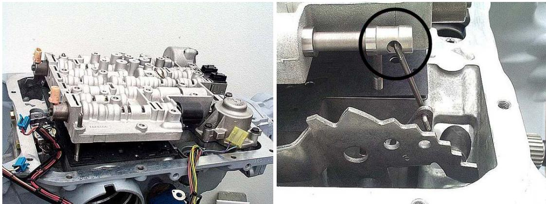
**Step 49:** Place the pressure switch assembly on top of the valve body and install the correct bolts through it as shown in the Bolt Location and Pattern chart link below, but don't tighten them yet. Lay the wiring harness over the valve body in the correct position. Hook up all solenoid and pressure switch assembly connections, making certain that all connector latches engage like they should.
