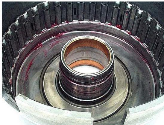
**Step 7:** Install new lip seals on the reverse input piston, then install the piston into the drum. Use a feeler blade or other suitable tool to guide the seal lips into the bores. Be very careful not to cut the seals.
