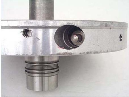
**Step 47:** Place the stator support in a vice between two blocks of wood. This is just to hold the support still, so don't apply a lot of pressure with the vice. Insert the t.v. boost valve assembly into the bore, open end down toward the pressure regulator valve. Gently push the sleeve into the bore while wiggling it around. The spring will push it back out, but this will get it into the correct position.
