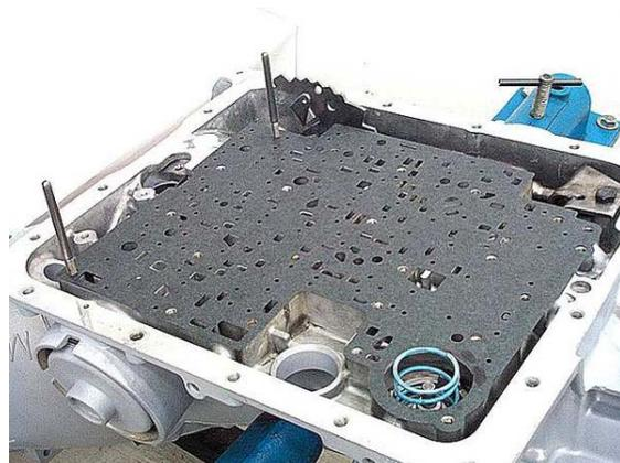
**Step 41:** Make sure that the separator plate screens are in place (4L60E), then lay the separator plate on top of the case gasket.
