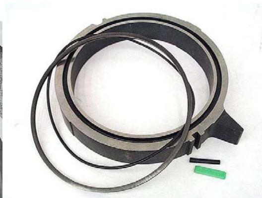
**Step 11:** Remove the slide swivel pin and pin spring, if equipped. This pin is not only a swivel point for the slide, it also acts as a seal. Inspect the pin closely for any wear from the slide.
