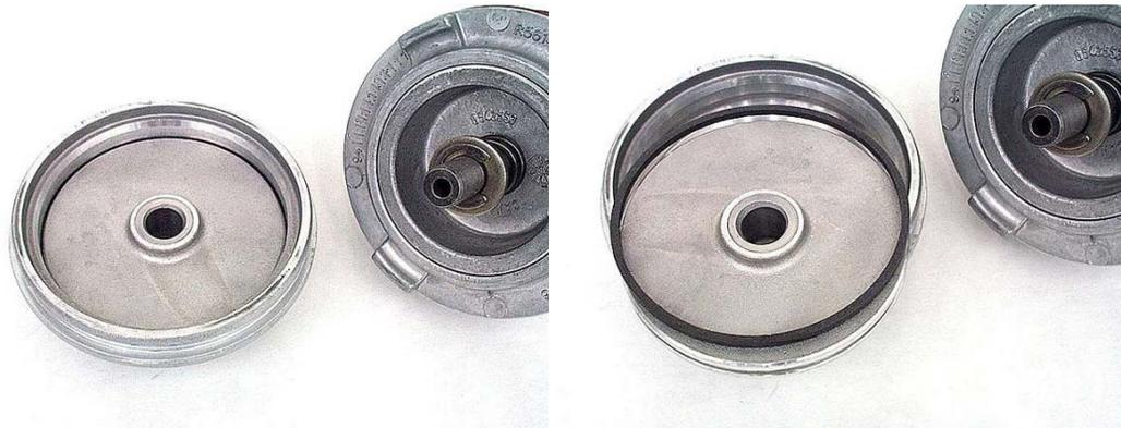
**Step 15:** Remove the guide ring from the servo. Remove the rubber o-ring from the guide ring.
