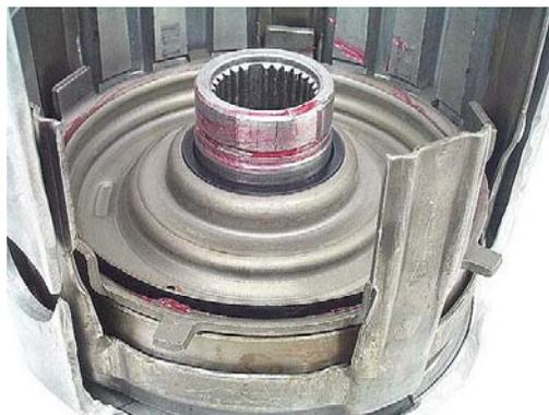
**Step 10:** Place the overrun piston return spring assembly onto the piston, making certain that the proper spring assembly is used for the piston you installed, according to the Updated Input Drum Pistons section listed above. Start the return spring assembly snap ring into position over the drum.
