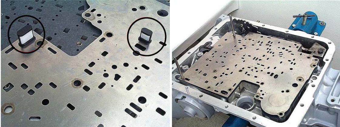
**Step 42:** Place the valve body gasket (identified by a 'V' cut into the gasket) on top of the separator plate.
