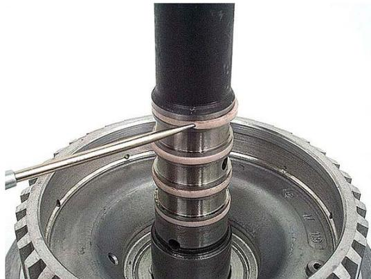
**Step 4:** Flip the drum over. To hold the drum upright while you work on it you can use a 4T60 input drum or other suitable device.
