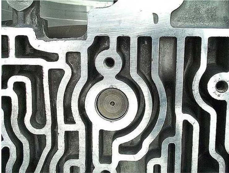
**Step 29:** Place the pump gasket into position on the case. Thread a pair of pump alignment pins into two pump bolt holes across from each other. You can make alignment pins out of two long 8mm bolts that fit the pump bolt holes in the case that you have cut the heads off of, rounded the cut end, then cut a screwdriver slot into.
