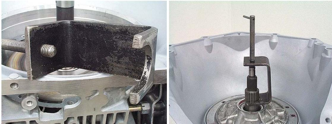
If you are going to pry the pump out rather than using a puller, be careful. Gently pry in several places, including the area between the reverse input drum and the pump.
