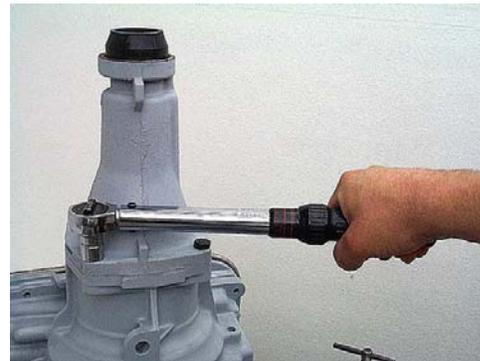
**Step 69:** Put a new o-ring on the output speed sensor, then slide the sensor into the extension housing and tighten the sensor bolt to 8 ft-lbs.
