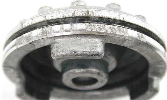
**Step 7:** Resurface the piston bore and pin with ScotchBrite™. Make sure that there is no wear on the pin.
