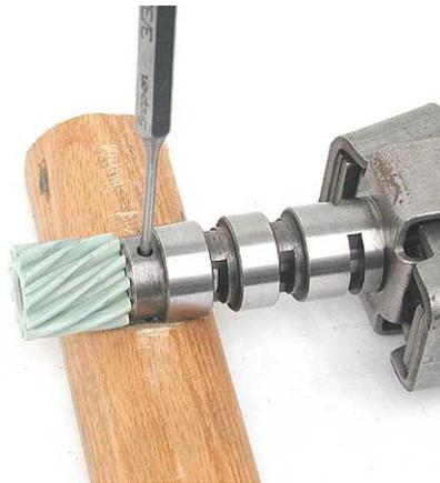
**Step 20:** Pull the gear out of the shaft. Use a small screwdriver to also pry the valve out of the governor shaft. Thoroughly clean the governor parts.
