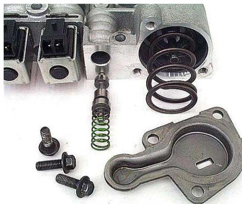
**Step 4:** Remove the accumulator spring, piston pin and piston. Remove the seal from the piston.
