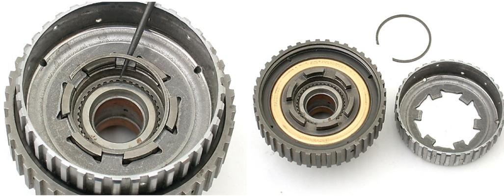
**Step 10:** Lift the sprag outer race from the assembly. Separate the sprag element and end plates from the inner race. Inspect both sprag races for wear or scoring. Inspect clutch hub teeth for wear.
