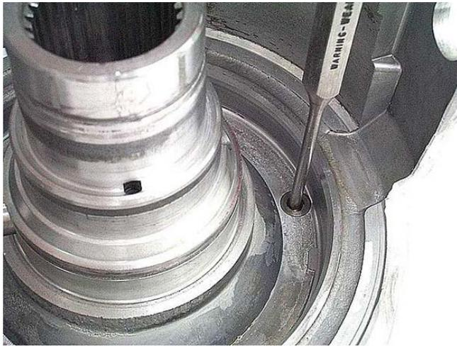
**Step 2:** Install the forward piston housing inner o-ring into the input drum groove as shown. This is usually a green o-ring in most kits. Coat the ring with assembly lube. Coat the drum center tower and 3-4 piston bore with assembly lube.
