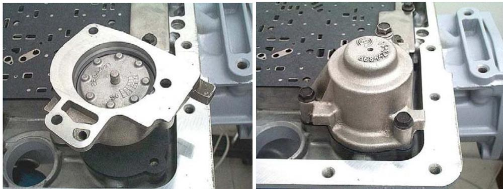
**Step 45 (4L60E):** Place the seven valve body checkballs into the correct positions on the separator plate as shown. A small dab of assembly lube on each of the holes before you put the checkballs on them will help keep the balls in place.
