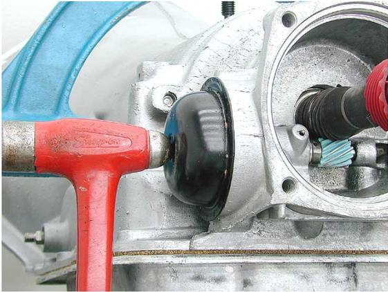
**Step 67:** If you remove the speedometer drive gear from a 4L60, install it at this time. Then install a new o-ring into the output shaft sleeve (if equipped). Slide the output shaft sleeve into place on the output shaft.
