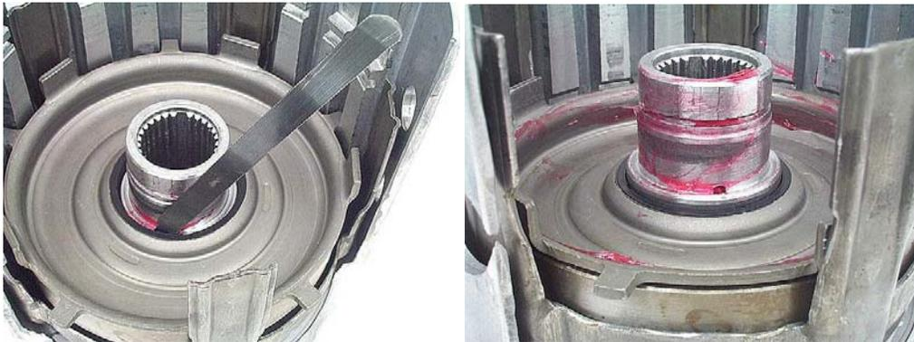
**Step 9:** Install the overrun piston into the forward piston, using a feeler blade to guide the inner piston seal over the snap ring groove in the drum tower. When fully installed, the piston should appear in the position shown.
