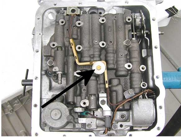
**Step 59:** Install the auxiliary valve body tube and the two tube hold-down brackets.
