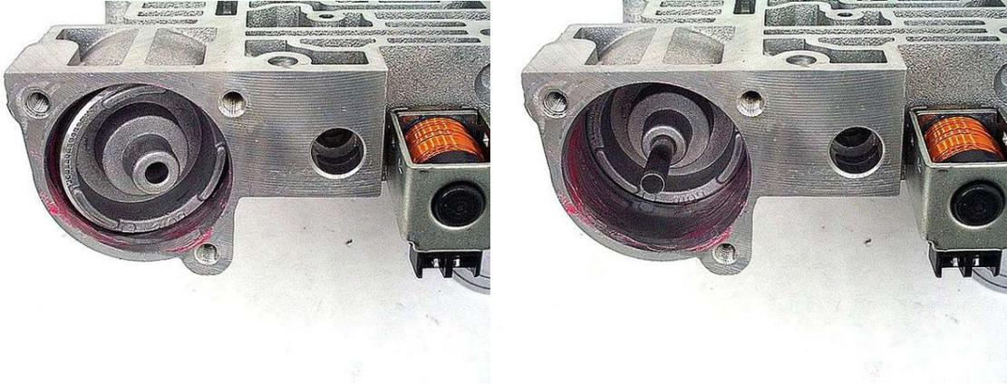
**Step 10:** Install the low overrun valve into its bore.
