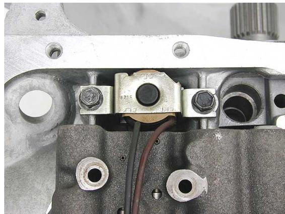
**NOTE:** Some model valve bodies have a TCC switch that may interfere with tightening the solenoid bolts. Lift the valve body a little bit to gain access to the bolts with a wrench.
