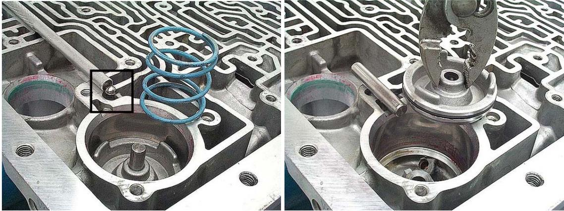
**Step 18:** Use a magnet to remove the 2-4 band anchor plug from the case.
