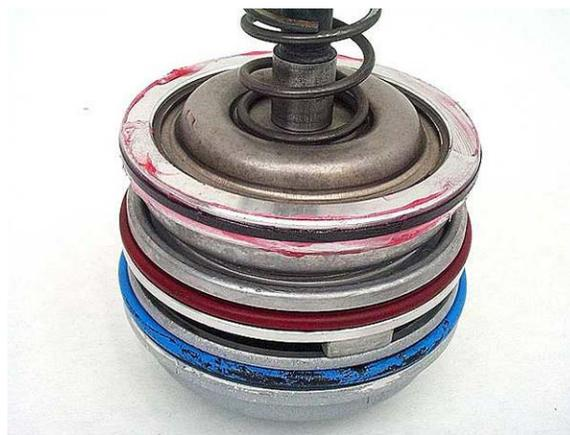
**IMPORTANT-** If the servo teflon ring sticks too far out of its groove, it's sure to get cut to pieces during servo installation. This is one of the most common rebuild errors made on this unit.
