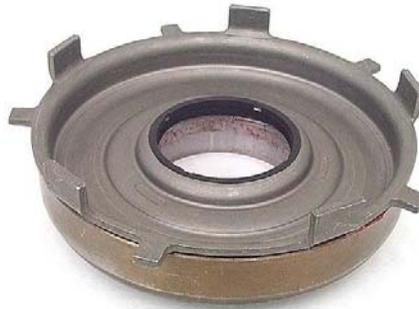
**Step 6:** Place the 3-4 clutch apply ring on the bench. Set the 3-4 clutch return spring assembly inside the apply ring. Place the forward piston and housing assembly on top of the 3-4 clutch return spring assembly, lining up the wide lugs on top of the forward piston with the fingers of the 3-4 clutch apply ring.
