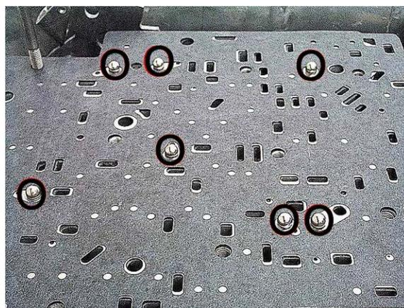
**4L60:** Place the two or three valve body checkballs, depending on the separator plate as shown, into the correct positions on the separator plate as shown. A small dab of assembly lube on each of the holes before you put the checkballs on them will help keep the balls in place.
