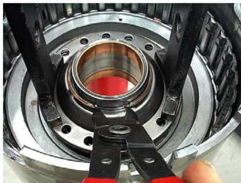
**Step 4:** Remove the return spring assembly from the drum. Remove the piston, and take the lip seals off of the piston.
