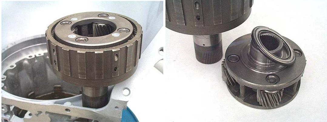
**Step 31:** Lift the sun gear shell out of the case and remove the metal thrust washer from the inside of the sun gear shell. Locate and retrieve the plastic thrust washer that was *under* the shell. It may have stuck to the backside of the shell or may be sitting on the low roller clutch inner race.
