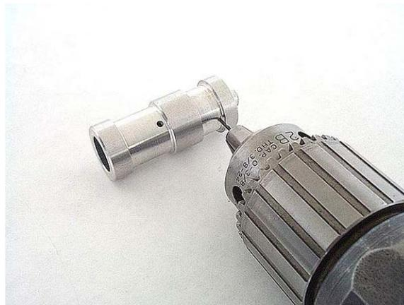
**Step 40:** Smear some assembly lube on the inner end of the boost valve, then slide the pressure regulator boost valve into the sleeve.
