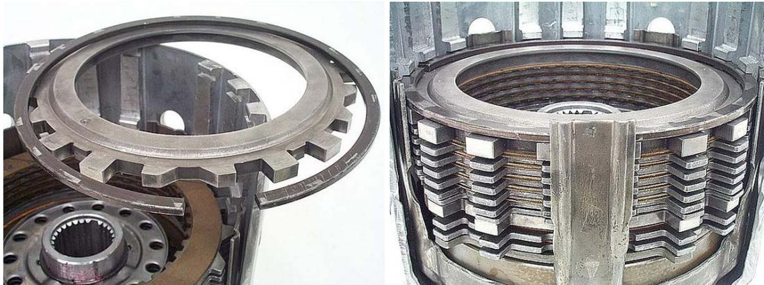
**Step 17:** Measure the forward clutch clearance between the pressure plate and the snap ring. The clearance should be 0.030"-0.063" (0.75mm-1.60mm). Adjust the clearance by changing the forward clutch pressure plate, which comes in the following sizes:
