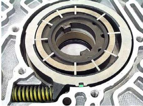
**Step 32:** Check the front stator bushing clearance between the bushing and the turbine shaft center journal. If it's not over 0.002", it can be re-used as long as the journal is in good shape.
