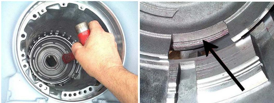
**Step 4:** Place the low-reverse piston return spring assembly on the piston. Set the proper snap ring on top of the return spring retainer. Install the appropriate spring compressing tool (the tabs on the ends of the cross-bar engage with the low roller clutch race snap ring groove in the case), and compress the return spring assembly.
