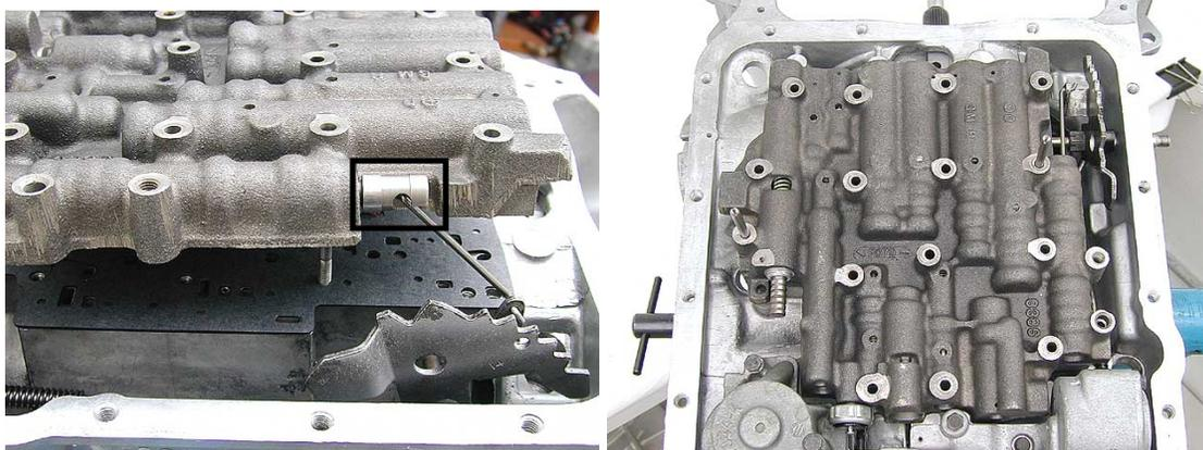
**Step 55:** Remove the alignment pins, replacing them with regular valve body bolts, but leave the bolts loose for now.
