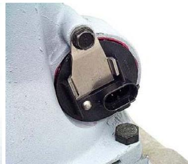
If the unit came to you with a range sensor and/or an external shift lever bolted to the manual shaft, install them now. Transmission assembly is now complete.
