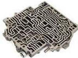
**Step 1:** The valve body must be completely disassembled and cleaned. Use the accompanying illustrations to identify the locations and names of the components as necessary.
