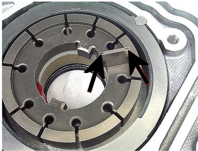
**Step 30:** Using a pick in a vane slot, push the bottom vane ring against the installed vanes. This should provide enough clearance to install the rest of the vanes.
