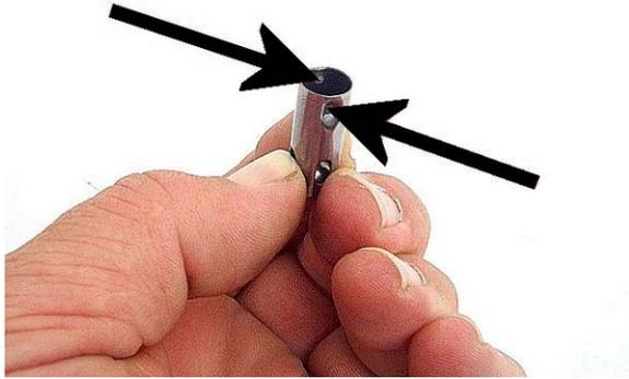
**Step 9:** blow any metal chips out of the capsule hole. Place a new checkball capsule into the hole, *open end up*. Use a 3/8" driver or a long 3/8" bolt with the threads cut off to drive the capsule into position.
