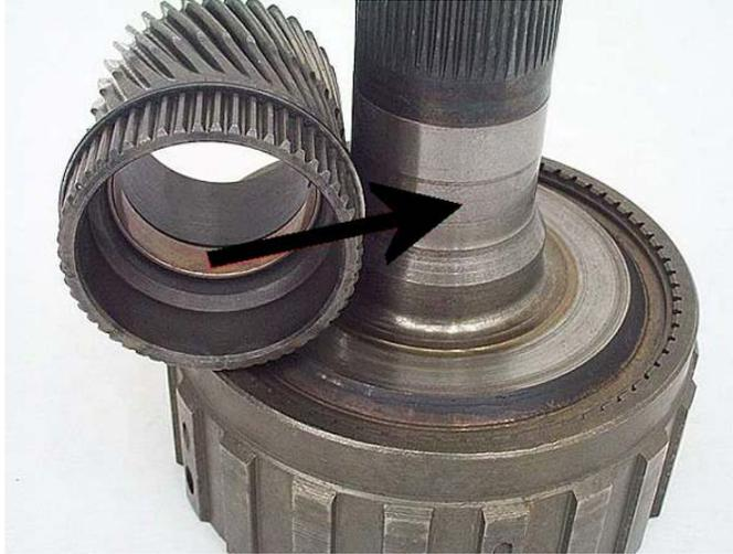
**Step 4:** Inspect all thrust surfaces for wear or scoring. Thrust surface discoloring is usually normal, and is not cause for replacement of the part. However, just like the bushing journals, if you can feel the wear there's too much there. These surfaces can also be reconditioned using ScotchBrite™ or #400 grit emery cloth.
