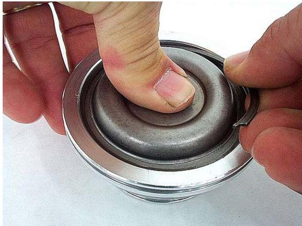
**Step 22:** Slide the servo pin into the 2<sup>nd</sup> gear piston. Place the spring and washer over the flat end of the servo pin. Install the clip into the servo pin groove to retain the spring and washer.
