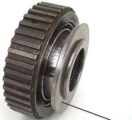
Rotate inner race counter-clockwise to install
