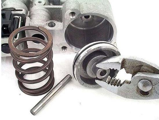
**Step 5:** Resurface the accumulator bore with ScotchBrite™.
