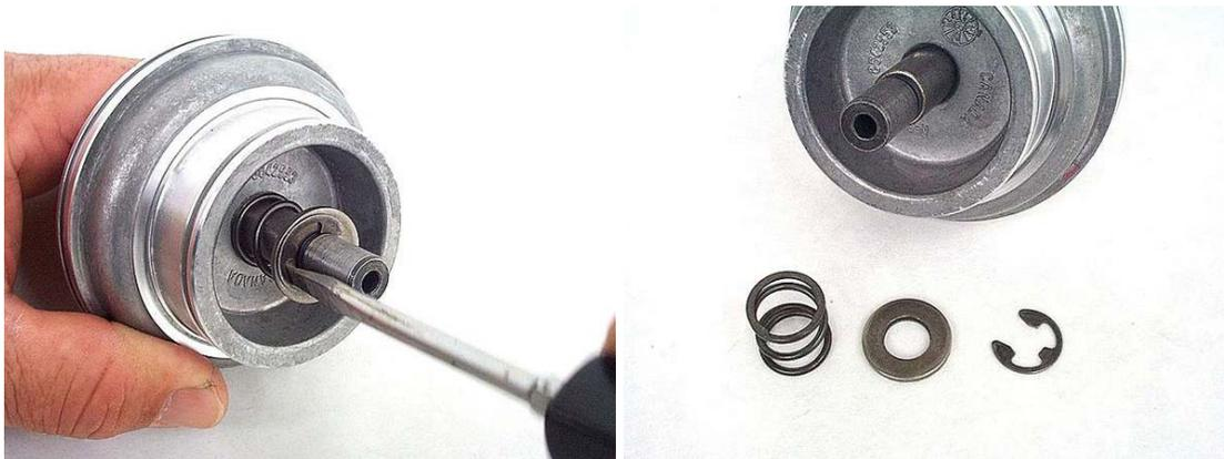
**Step 17:** Use a file to remove any ridge from the servo pin area shown. This will keep from scratching up the inside of the piston pin bore, causing apply circuit leaks. Slide the servo pin out of the piston.
