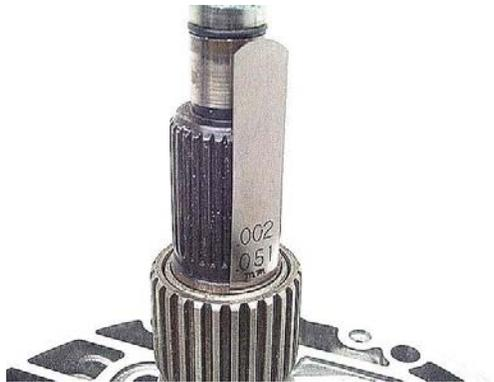
**Step 33:** Always replace the rear stator bushing. This bushing is responsible for maintaining centerline throughout the transmission more than any other bushing, and is subject to rather high loads.
