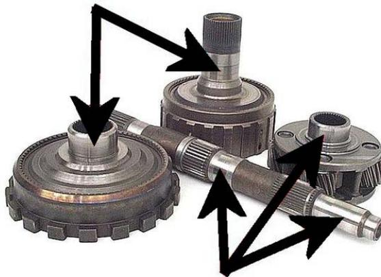
**Step 3:** Although all bushings and bushing journals must be checked for wear and clearance, there is only one geartrain bushing that should be replaced during any internal service, the rear sun gear internal bushing. This is a critical alignment bushing and is also under substantial load. This bushing also bears most of the load caused by any imbalance of the front planet and input sprag assemblies.
