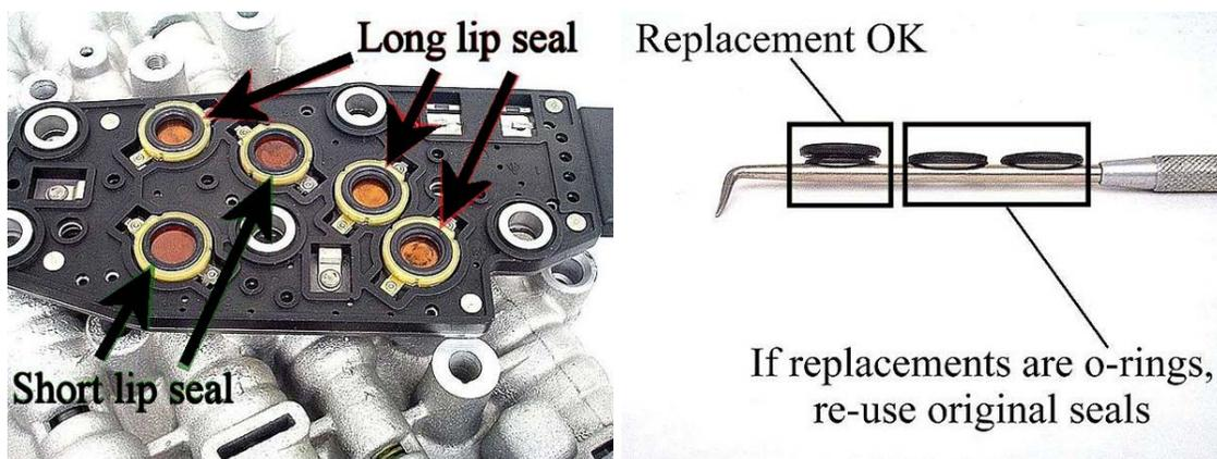
When installing the large lip seals, make sure that the entire lip is under the diaphragm pocket's plastic inner ledge. You can help by pushing on the ID of the seal with the corner of your pick. The small lip seals go in with the sharper edge first, against the diaphragm.
