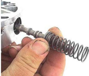
**Step 42:** Place the pressure regulator valve snap ring onto the snap ring pliers. Use the pliers to push the boost sleeve assembly into the bore. If you can't get the snap ring all the way into the groove this way, release the snap ring to hold the sleeve in the bore. Press the snap ring the rest of the way in with a pair of needle nose pliers or a small screwdriver until the snap ring is firmly locked into its groove.
