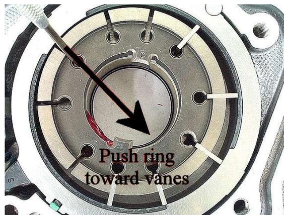
**Step 31:** Once all vanes are installed, check to make sure that all vanes are below flush with the top of the pump pocket. Install the top vane ring inside of the pump vanes. Squirt ATF all over the rotor and slide assembly. The pump body is done for now, so let's move on to the stator support.
