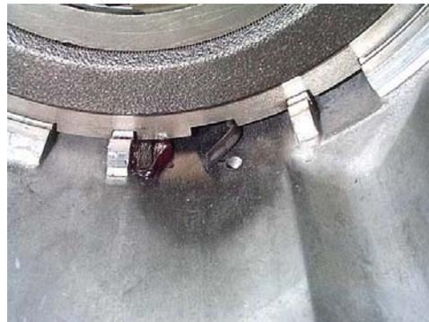
**Step 13:** Install the low roller clutch assembly snap ring, making sure that the anti-clunk spring tip goes between the snap ring ends.
