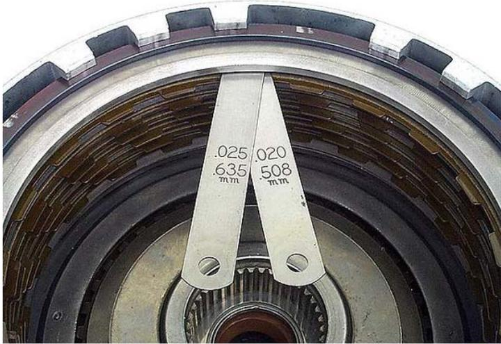
**Step 24:** Flip the drum over and air check all three clutch apply circuits through the turbine shaft. While checking the 3-4 clutch apply circuit, make sure that the checkball capsule is sealing properly. You should not be able to see, hear or feel any appreciable flow of air from this capsule.
