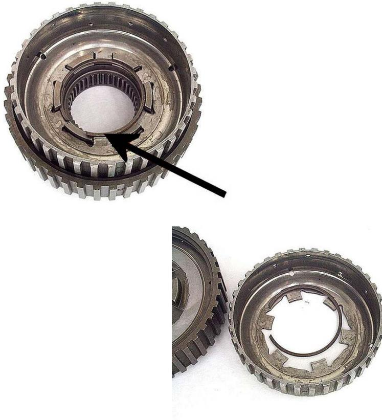
**Step 17:** Remove the sprag inner race from the assembly. Separate the sprag element and end plates from the components. Inspect both sprag races for wear or scoring. Inspect clutch hub teeth for wear.
