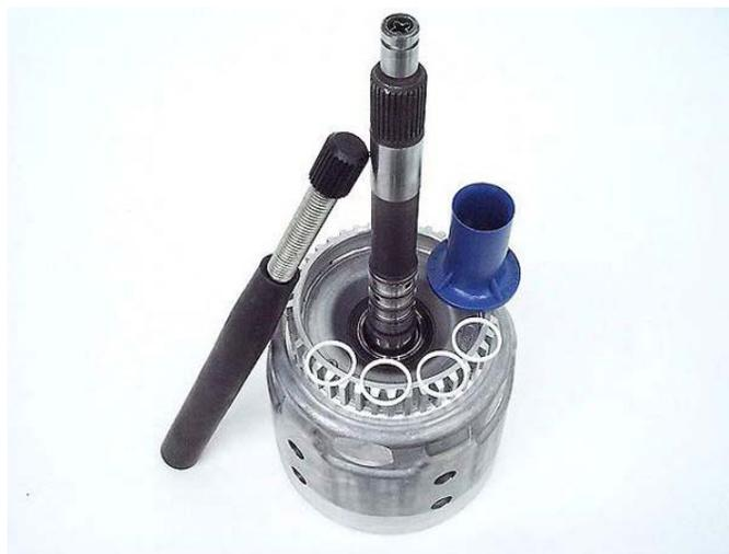
**Step 25:** Using the special tools shown, install the turbine shaft seal rings in the following manner:
