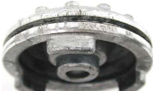
**Step 15:** Make sure that there is no wear on the pin. If wear is found, the housing must be replaced. Resurface the piston bore and pin with ScotchBrite™, then flat sand the mounting surface of the housing. Thoroughly clean the housing and piston.
