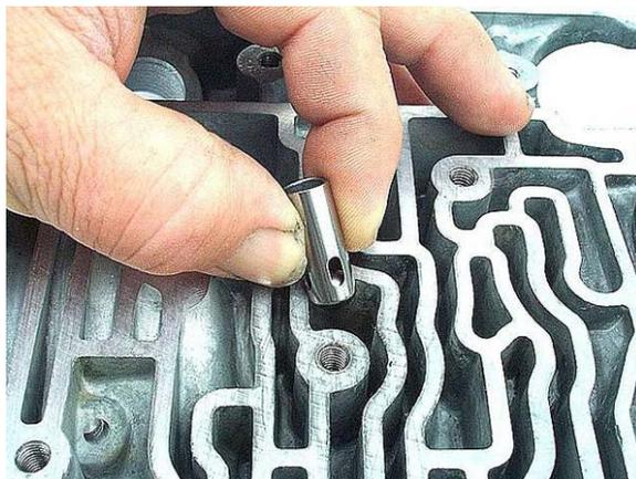
**CAUTION:** The capsule must be driven into the hole to the proper depth. If this is not done properly, serious unit malfunction will occur. Using the driver mentioned above, gently tap the capsule into the bore while watching through the servo bore until the entire capsule window is visible through the servo bore.
