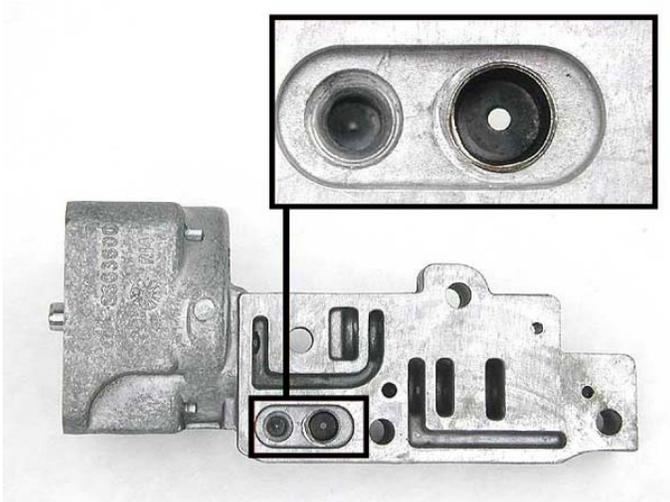
**Step 10:** Install a new seal on the accumulator piston. Coat the housing bore and pin with assembly lube, then install the piston into the bore.
