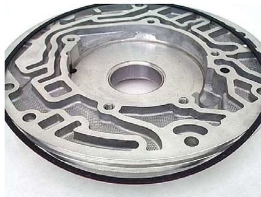
**Step 14:** Remove pump body bushing (unless the bushing is going to be re-used).
