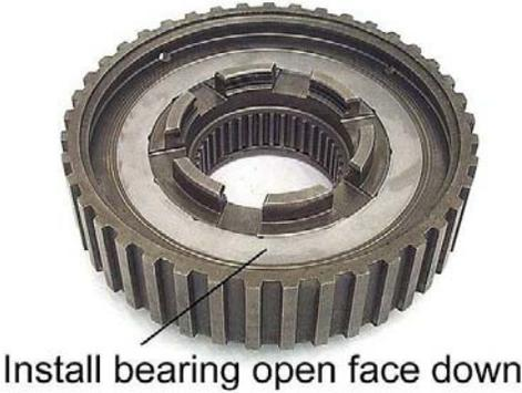
**Step 23:** Place the overrun clutch hub into position on the sprag assembly as shown and lock it into place with the snap ring.
