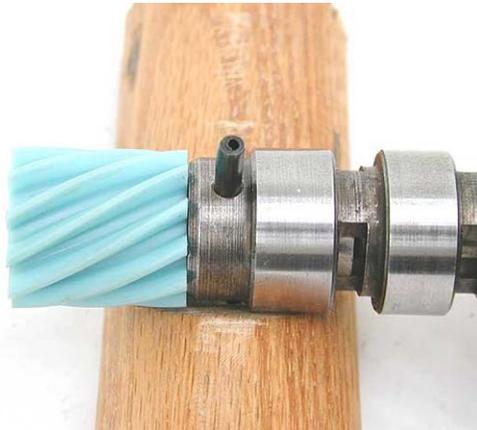
**Step 24:** Using your wood block for support, tap a new roll pin into the governor gear, making sure that both ends are below flush with the governor shaft.
