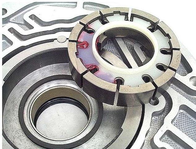
**Step 28:** Place the rotor into the pump pocket (guide ring down, if equipped).
