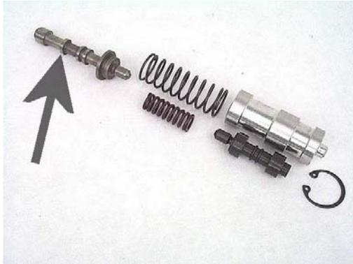
**Step 39:** Before assembling the boost valve and sleeve, drill the hole in the boost sleeve as shown to 0.042" (#60 drill) to improve line pressure response time. Make absolutely sure that there are no burrs left inside the sleeve from the drilling operation.
