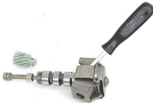
**Step 21:** Place the governor valve back into the shaft, shorter end first. Make sure that the valve moves freely inside the shaft.
