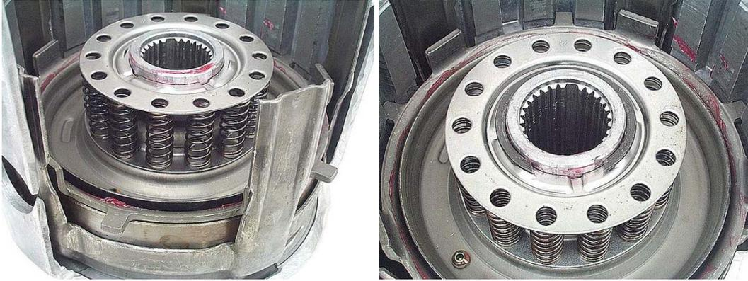
**Step 11:** Using an appropriate compressing tool, compress the overrun return spring assembly far enough to install the snap ring. Make sure that the ring goes inside of all four snap ring retaining tabs on the spring assembly.
