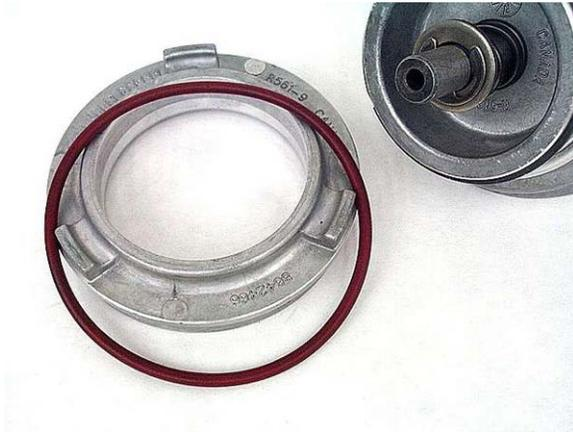
**Step 16:** Remove the seal rings from the 2<sup>nd</sup> gear piston. Remove the e-clip from the servo pin, then slide the washer and spring off of the pin.
