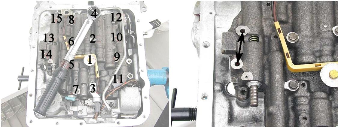
**Step 61:** Connect any switches that still need to be hooked up, then install the manual lever detent spring and tighten the bolt good and snug.
