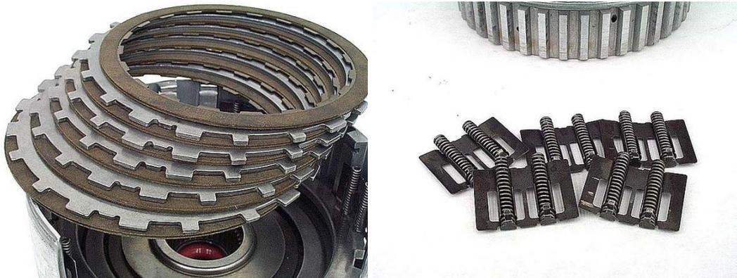
**Step 7:** Remove the 3-4 clutch apply plate. There may be either a single or double apply plate assembly, depending on model.
