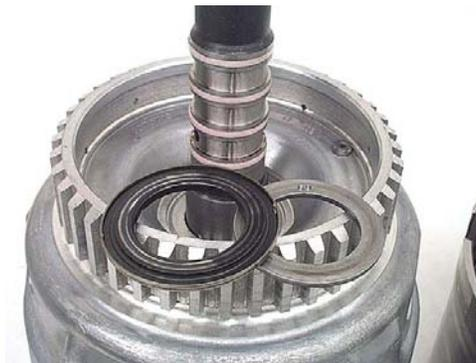
**Step 22:** Remove the turbine shaft o-ring.
