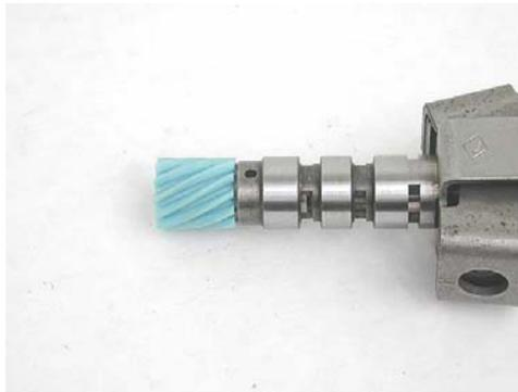
**Step 23:** Using a 1/8" drill, drill *only halfway* through the governor gear. Once this is done, insert the drill into the other side of the governor and drill through the gear. This way the hole in the gear is properly aligned with the hole in the shaft.
