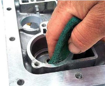
**Step 12:** Flat sand the valve body surface of the case, and remove any pump gasket material from the pump surface of the case.
