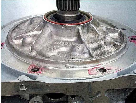
**Step 32:** Torque the pump bolts in a crossover pattern to 18 ft-lbs. Put a new o-ring in the groove on the tip of the turbine shaft.
