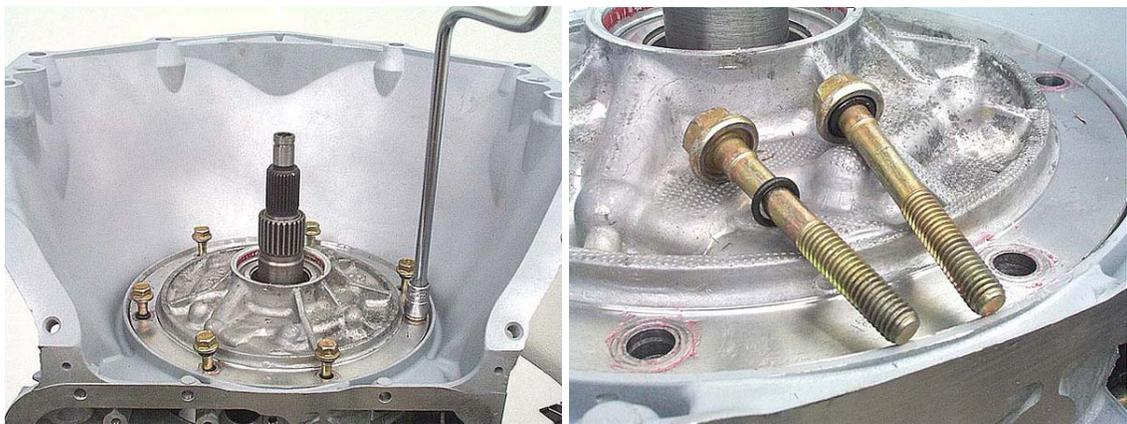
**Step 25:** Using a suitable puller, remove the front pump.
