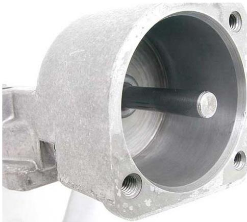
**Step 8:** Remove both valve bore assemblies from the housing and flat sand the mounting surface of the housing.
