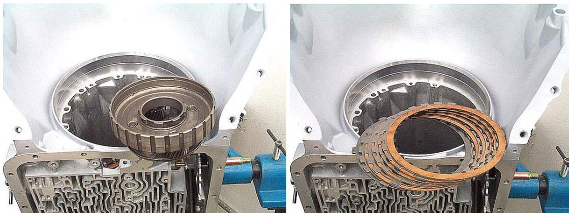
**Step 36:** Reach through the rear ring gear with your finger and remove the rear ring gear from the case. Any low-reverse clutch plates that didn't come out with the planet will come out with the ring gear. Locate and save the rear ring gear thrust bearing, which may be on the ring gear or sitting in the bottom of the case.
