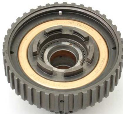
**Step 15:** Place the overrun clutch hub into position on the sprag assembly as shown and lock it into place with the snap ring. Make sure the snap ring ends are on either side of a gap in the race lugs as shown.
