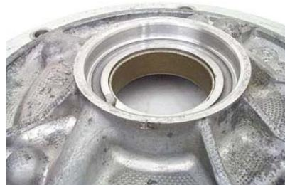
**Step 19:** Place the rotor into the pump bore where it normally rides. Lay a straight edge across the rotor. Measure the clearance between the straight edge and the rotor at several points around the rotor. The clearance must be between 0.0015"-0.0025".
