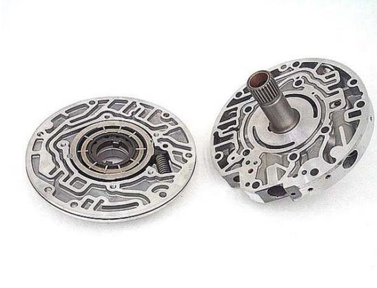
**Step 6:** Remove the top pump vane ring (which may be sticking to the stator support).
