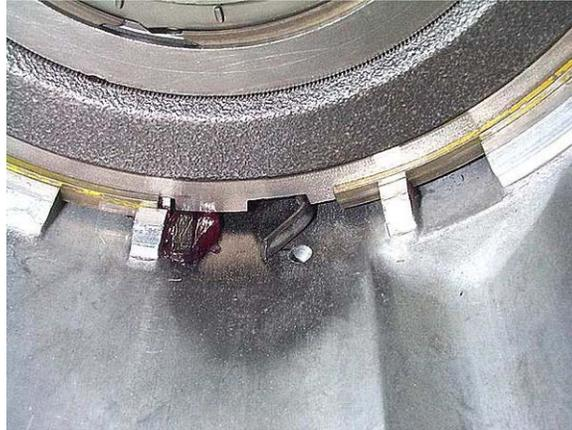
**Step 14:** Place the plastic thrust washer on the low roller clutch inner race, engaging the washer tabs with the race lugs. Use assembly lube to hold the washer in place.
