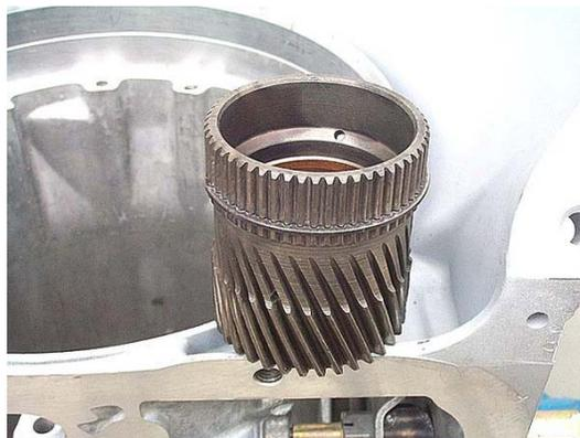
**Step 33:** Remove the snap ring holding the low roller clutch assembly into the case.
