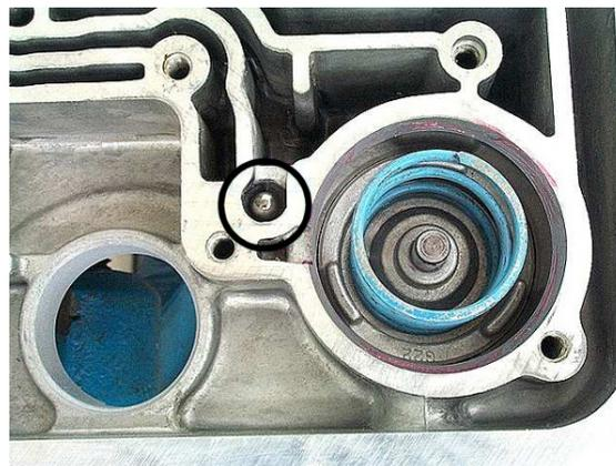
**Step 38:** On 1987 and later units that use a low-reverse waved cushion plate, there should be a checkball inside a capsule near the low-reverse case apply passage. If the ball is not in the capsule, place a 1/4" checkball in the capsule. The 4L60E has no other loose checkballs in the case.
