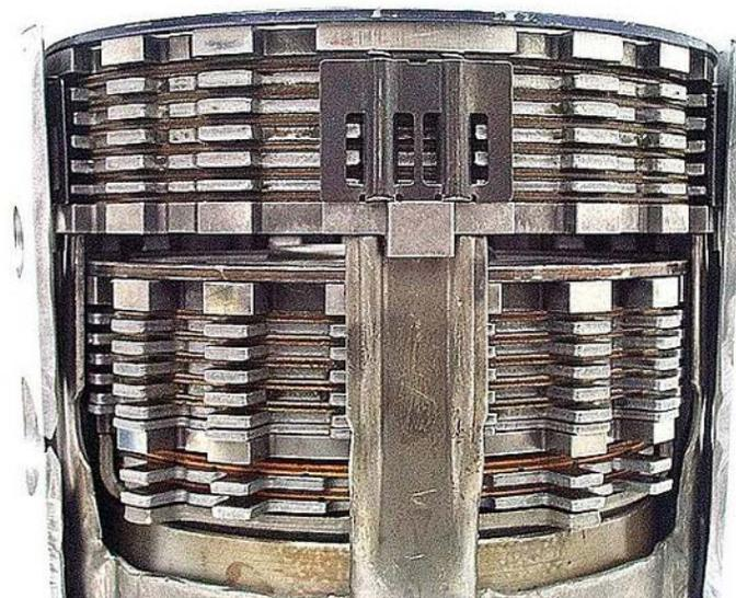
**Step 23:** Measure the clearance between the backing plate and the top friction plate. The factory clearance specification is 0.035"-0.083" (0.90mm-2.10mm), but it's a good idea to keep the clearance under 0.060" for a good, clean 2-3 shift. Clearance can be adjusted by either mixing thick and thin steels or by changing the selective backing plate to a plate of the proper thickness. The backing plates are available in three sizes:
