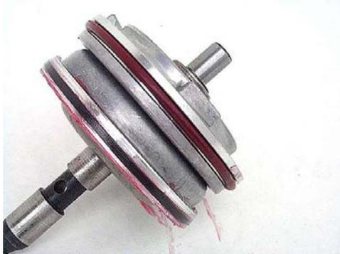
**Step 25:** Coat the 4<sup>th</sup> piston seal ring groove with assembly lube, then install the seal ring into the groove. Place the 4<sup>th</sup> piston over the flat end of the servo pin as shown, with the larger-bump side of the 4<sup>th</sup> piston facing away from the 2<sup>nd</sup> piston.
