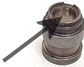
**Step 45:** Slide the pressure regulator valve and spring into the stator support, making sure that it slides freely the full length of its travel.
