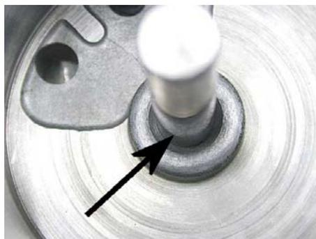
**Step 6:** Inspect the accumulator piston edge for any signs of scoring or wear. If wear is found, replace the piston.
