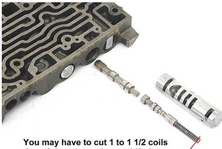
You may have to cut 1 to 1 1/2 coils from 2-3 spring to lower shift time.
