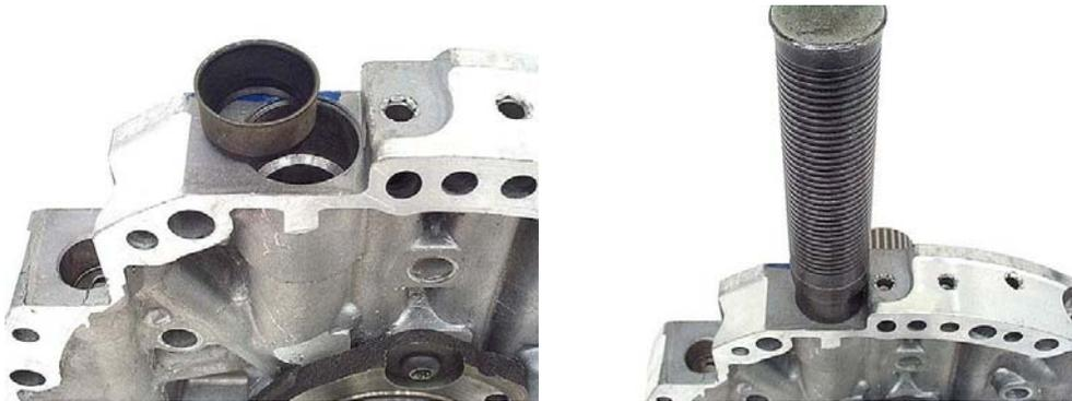
**Step 50:** Lay the serviced pump body face-up on the bench and line up the stator support over it. You can use the two closely-spaced holes next to the pressure regulator valve bore as line-up markers.
