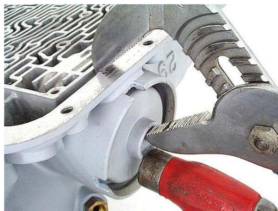
Once the servo bore snap ring groove is exposed, slide the snap ring into the bore groove. Make sure that the snap ring is seated all the way into the groove. Dirt or scale deposits can keep the ring lifted out of the groove a bit, allowing the ring and servo to pop out of the bore in operation.
