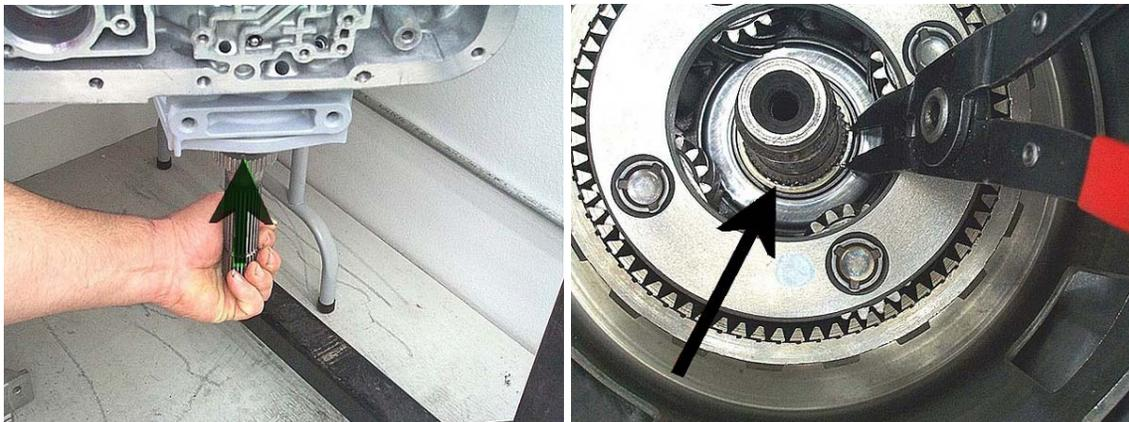
**Step 30:** Grab the outside of the ring gear hub and lift the planet, hub and shaft assembly out of the case. Separate the planet from the ring gear and retrieve the thrust bearing from between the planet and the ring gear.
