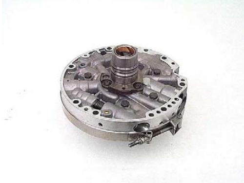
**Step 52:** Tighten the pump strap until it's good and snug. The stator support should still be able to rotate within the strap a little bit. Line up the bolt holes by eye. Torque the five pump bolts to 18 ft-lbs., using a star-shaped tightening pattern.
