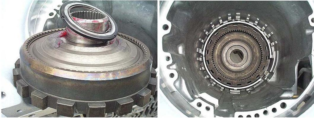
**Step 8:** Place the rear planetary assembly rear thrust bearing into position on the back of the rear planetary assembly as shown, using assembly lube to hold the bearing in place. Lower the planetary assembly into the rear ring gear, engaging the ring gear teeth.
