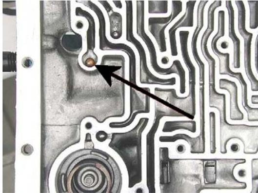
**Step 39:** Make sure that the band anchor pin is fully seated in the case anchor hole. Install two valve body alignment pins into the holes shown. You can make alignment pins out of two long 6mm bolts that fit the valve body bolt holes in the case that you have cut the heads off of, rounded the cut end, then cut a screwdriver slot into.
