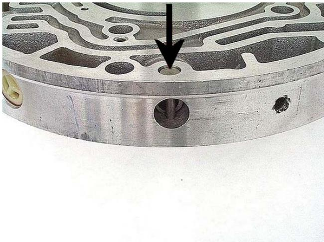
**Step 37:** Drop the two TCC apply valve springs into the TCC apply valve bore. Slide the valve into place after the springs, small diameter end first. Push on the valve with a small screwdriver to make sure that the valve strokes throughout its travel freely. Set the retainer plate in place, then install the retaining clip into the bore. Make sure that the entire snap ring properly locks into the snap ring groove.
