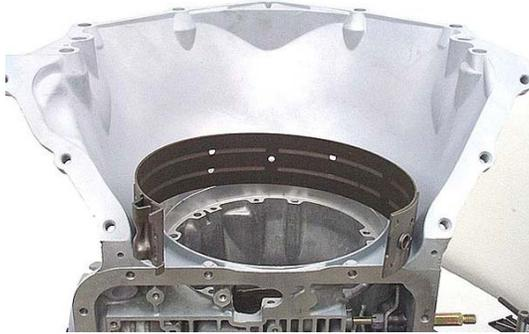
**Step 28:** Remove the front sun gear from the case.
