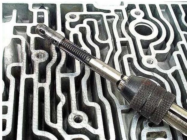
**NOTE:** The tap may bottom out on the ball before getting a good grip on the inside of the capsule. If so, drive a 5/16" punch or bolt into the capsule. This should flatten the capsule bumps that retain the ball, allowing you to pull the ball out with a magnet. The tap should now properly grip the capsule.
