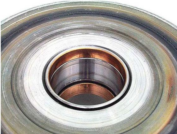
Place the appropriate thrust washer on the stator support, and set the reverse input drum on the support. Check the top drum bushing for clearance. There must be no more than 0.003" clearance between the bushing and the journal. Check the drum for any side-to-side or rocking motion. If there is any motion, replace the drum bushings. Be sure to chamfer the edge of the larger bushing after installation to help the drum go over the seal rings during unit assembly.
