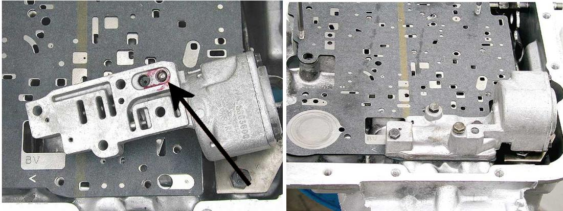
**Step 44:** Place the 1-2 accumulator housing on the separator plate, install the proper bolts, then tighten bolts to 8 ft-lbs.
