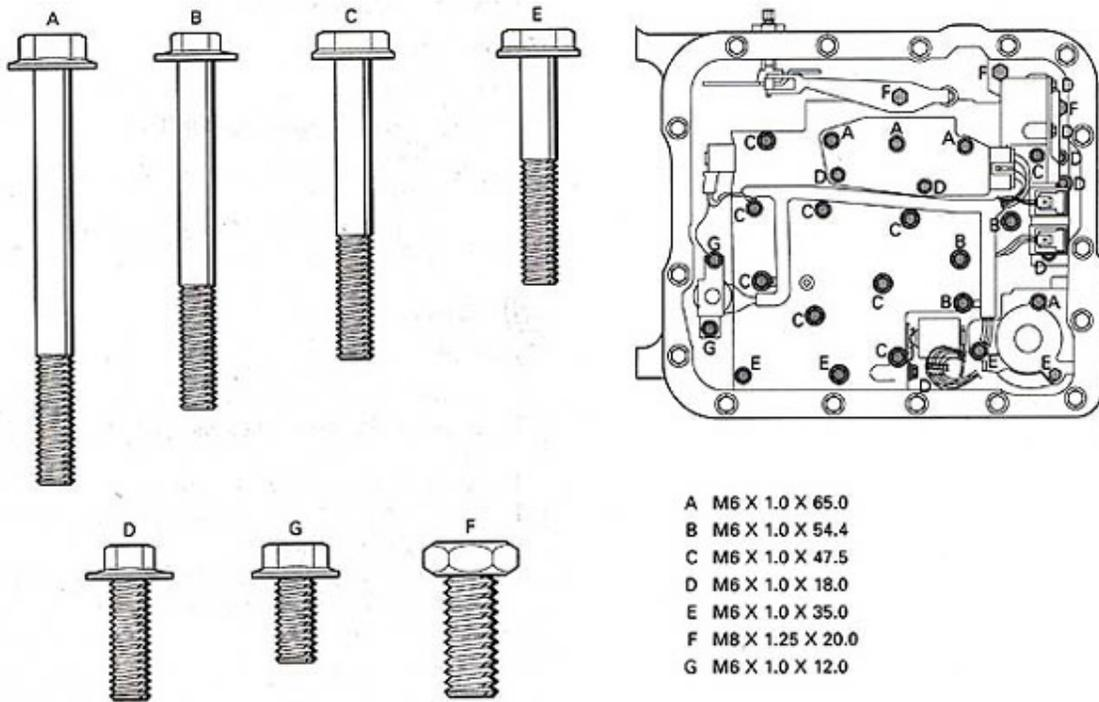
**IMPORTANT-** Be sure you check bolt lengths! Small length differences are important. The wrong bolt in one of the middle valve body holes can snag the sun gear shell, causing wrong gear starts and bind-ups!
