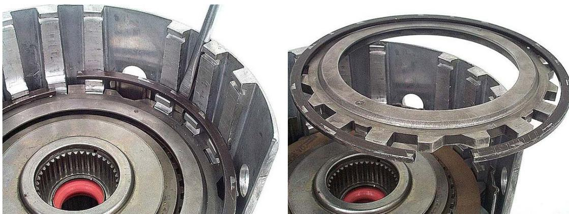
**Step 9:** Remove the forward sprag assembly. Remove the thrust bearing and lube seal from the input drum.
