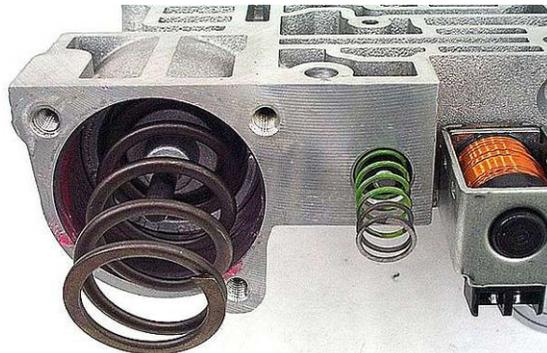
**Step 12:** Install the accumulator cover, hand-tightening the bolts.
