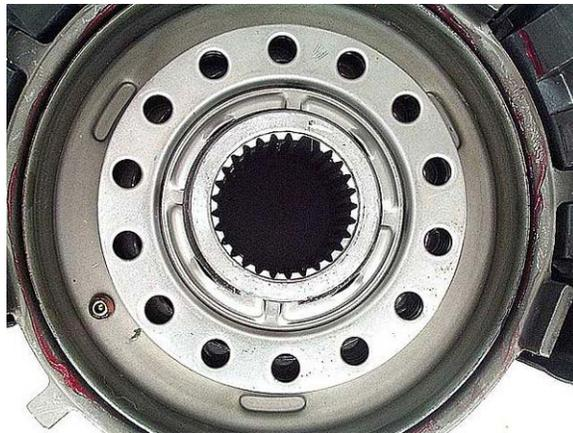
**Step 12:** Install the overrun clutch set, two friction and two steel plates, starting with a steel plate. The teeth of the steel plates must go into the narrow slots of the drum, between the wide forward piston lugs.
