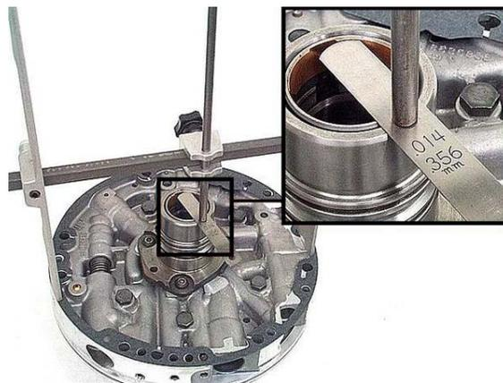
The factory specification for this clearance is between 0.005" and 0.036". Since you need to allow for gasket crush, keep the minimum clearance above 0.010". To maximize unit life, keep the maximum measured clearance below 0.025".
