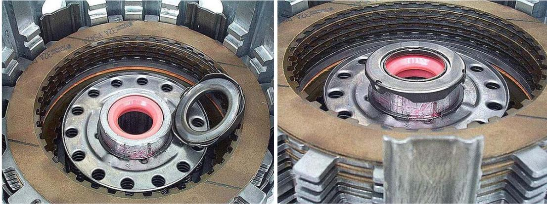
**Step 19:** Install the input sprag into the drum (which is shown being serviced in the Gear Train section), feeding it through both sets of clutches. You will know when the sprag is all the way down against the thrust bearing when you can push down on the sprag and still turn it easily in both directions. Once the sprag is in place, re-install the forward clutch pressure plate and snap ring.
