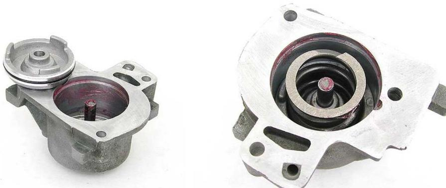
**NOTE:** The spring and piston position may be reversed on your model. Install the parts in the same direction they came out.
