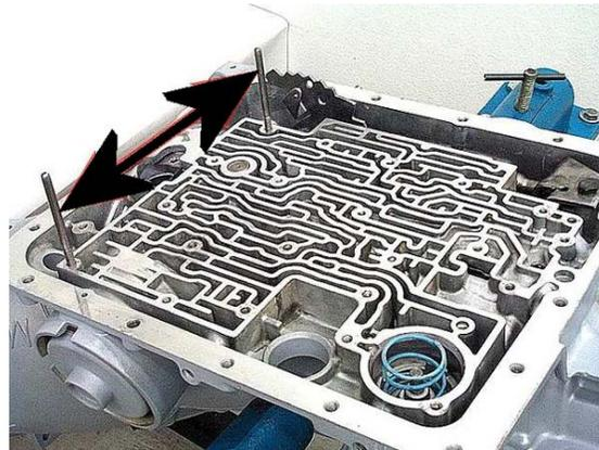
**Step 40:** Place the case gasket (identified by a 'C' cut into the gasket) on the case.
