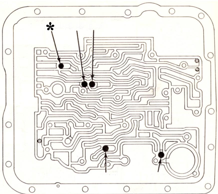
**NOTE:** 4L60s may come with a larger, copper-colored #10 checkball in the pocket shown. If so, *do not* reinstall this checkball. They cause more problems than they're worth.
