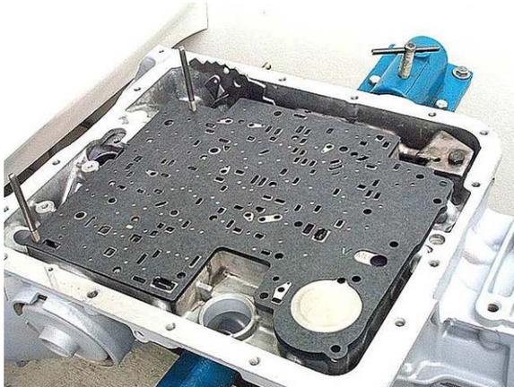
**Step 43: Early 4L60 & 4L60E-** Set the separator stiffener plate into position on the separator plate.
