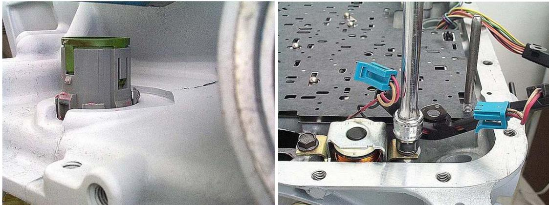
**Step 48:** Pull the wiring harness away from the valve body gasket, then carefully lower the valve body onto the case. You must guide the free end of the manual valve link into position in the end of the manual valve along the way.
