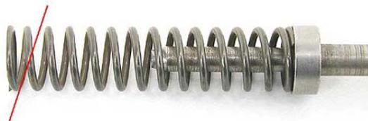
When using this kit, you may find the minimum 2-3 shift time now *seems* just a bit too late. This is because engine RPM is higher at this speed because TCC has not engaged. Remedy this by cutting 1 to 1-1/2 coils from the 2-3 shift valve spring. Always aim the cut spring end *away* from the valve.
