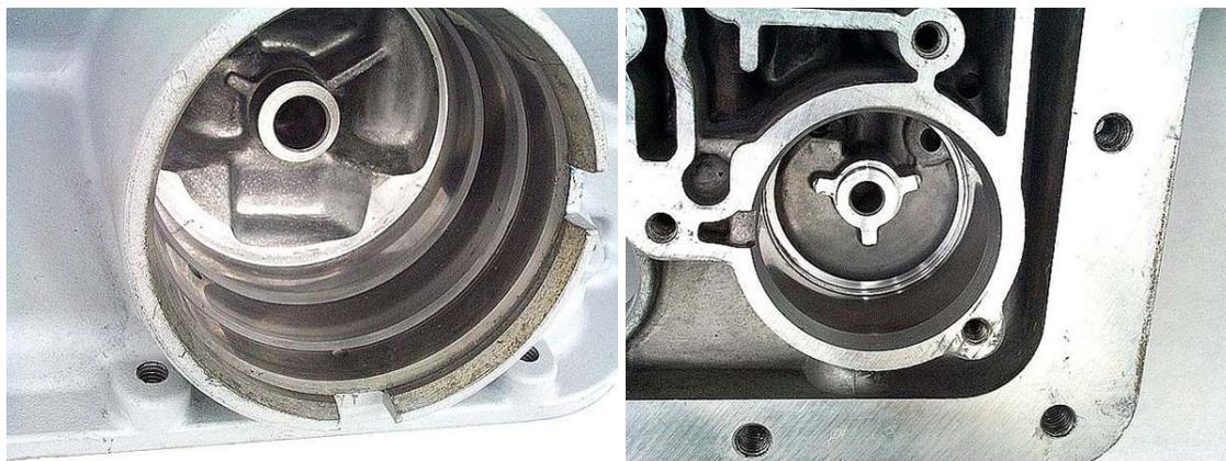
**Step 6:** If the previous steps do not reveal any damage, then the case should be okay to rebuild. Scuff up the accumulator bore with ScotchBrite™.
