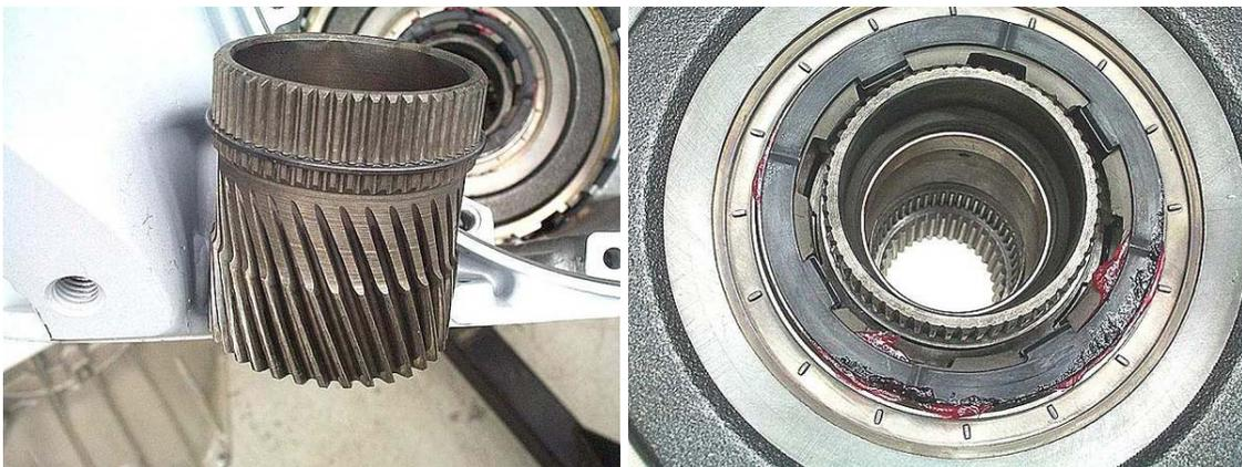
**Step 16:** Place the sun gear shell-to-front ring gear thrust washer in place in the shell, engaging the washer tabs with the holes in the shell. Use assembly lube to hold the washer in place.
