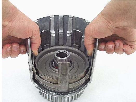
**Step 8:** You will need to help the inside piston seal over the last bump in the drum with a feeler blade or other suitable tool. Once the piston has cleared the last bump and is in the proper position, you will see about 3/16" of drum above the seal below the first step. When you press down on the piston, it will spring back a little bit. Coat the seal bore in the top of the forward piston with assembly lube.
