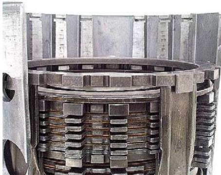
or a thin stamped steel plate with feet for the apply ring fingers, with a stamped steel stepped plate on top of it, followed by an early 4L60-style 3-4 clutch steel plate with wide teeth to engage the drum slots.
