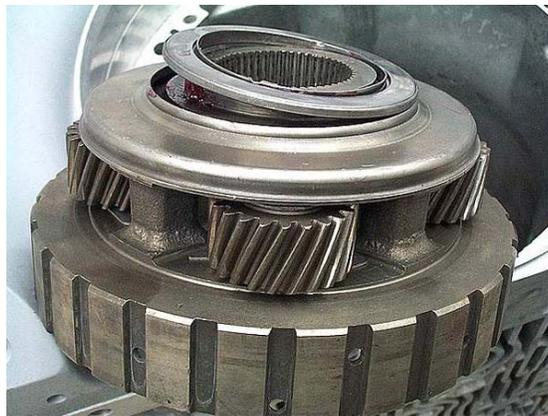
**Step 9:** Install the anti-clunk spring into the case, holding it in place with a blob of assembly lube as shown.
