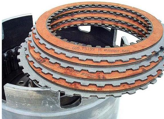
**Step 11:** Install the selective pressure plate and snap ring into the drum.
