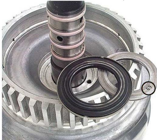
Once you know the correct selective washer size to use, install the correct selective washer under the thrust bearing on top of the input drum.
