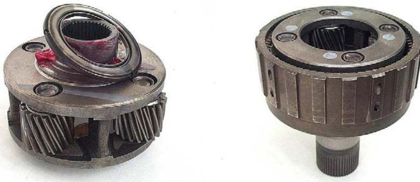
**Step 19:** Lower the hub and planetary carrier into the case, engaging the hub splines with the rear planetary carrier internal splines. Rotate the hub into position, making sure that the hub is all the way down against the sun gear shell thrust washer.
