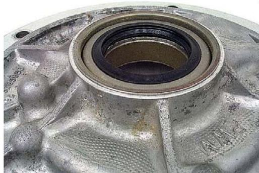
**Step 23:** Coat the pump pocket with assembly lube, then install the slide seal ring and rubber support ring into the slide groove. Install the pump slide into the pump body.
