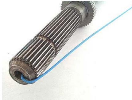
**Step 21:** Install the output shaft into the unit from the back of the case, rotating it to engage the rear ring gear and front planetary carrier splines along the way. Once the shaft is in position, slide the straight end of coat hanger through one extension housing bolt hole. Slide the wire up until the hook on the end of the wire engages with the hole in the rear end of the output shaft. While holding the shaft in place, bend the wire above the case bolt hole to hold the shaft in position.
