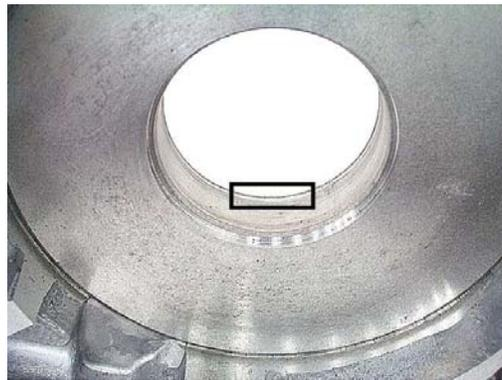
**CAUTION:** The pump body bushing bore may have a ridge at the front of the bore to keep the bushing from moving out of the bore. The bushing must **not** be pressed past this ridge, otherwise the ridge may be removed. Always look for this ridge before removing the pump bushing.
