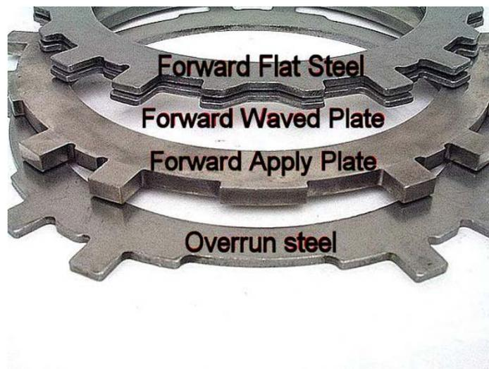
**Step 13:** Install the forward clutch apply plate.
