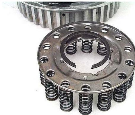
**Step 12:** Grab the drum by the turbine shaft, flip it over and slam it against the bench again. Isn't transmission rebuilding fun? All piston assemblies except for the 3-4 piston should fall out of the drum. Separate the forward and overrun piston assemblies, and remove the lip seals from the overrun piston.
