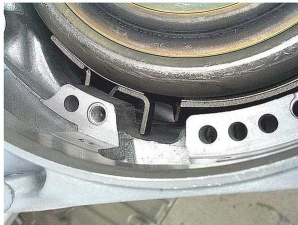
**Step 28:** Install the band anchor pin into the proper case hole. From this point on, be careful not to handle the case in such a way that would allow the anchor pin to fall out of position. It can sometimes be difficult to get the end of the band re-aligned with the anchor pin once it slips out.
