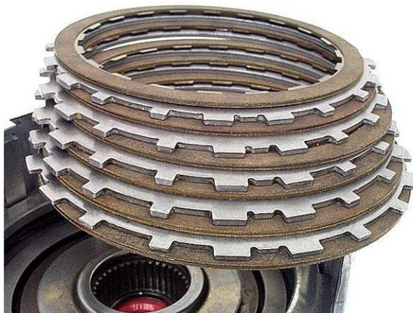
If your drum has the one-piece apply plate, use thick steel clutch plates which measure 0.107" thick.
