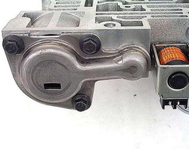
**Step 13:** Remove the 1-2 accumulator piston and spring from the accumulator housing, taking notice of which order they came out of the housing in. Remove the seal from the piston. Clean all accumulator parts.
