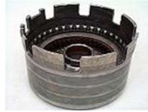
**Step 1:** Remove the clutch snap ring and pressure plate.
