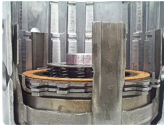
**NOTE:** There are several types of steel plates used in the input drum that are very similar, but will not interchange. The correct plates must be installed in the correct locations. Use this illustration to determine correct plate location. The plates are shown in their proper respective position within the input drum.
