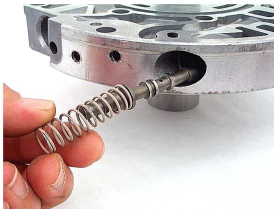
**Step 46:** Slide the reverse boost valve and sleeve into the pressure regulator valve bore, with the exposed valve stem pointing outward as shown.
