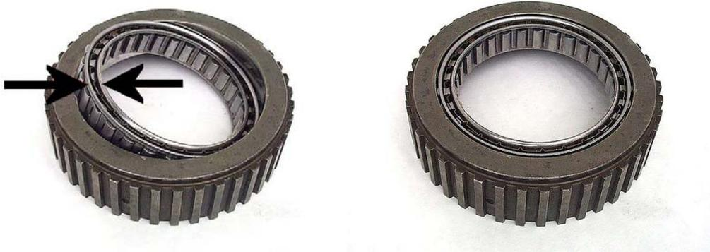
**Step 20:** Place an end bearing on the inner sprag race as shown.
