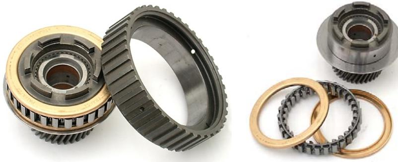
**Step 11:** Use #240 grit emery cloth to break through the glaze on both inner and outer sprag races. Finish both surfaces with #320 grit emery cloth. Thoroughly clean all sprag components.
