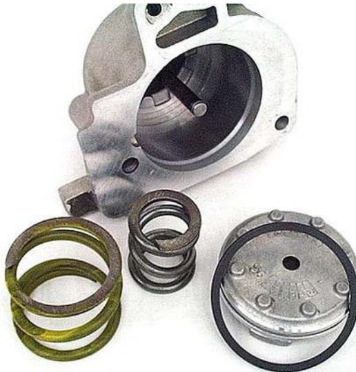
**Step 14:** Recondition the accumulator bore surface with ScotchBrite™. Place a new rubber seal on the accumulator piston. Coat the bore with assembly lube and reinstall the piston and springs into the accumulator housing in their original order.
