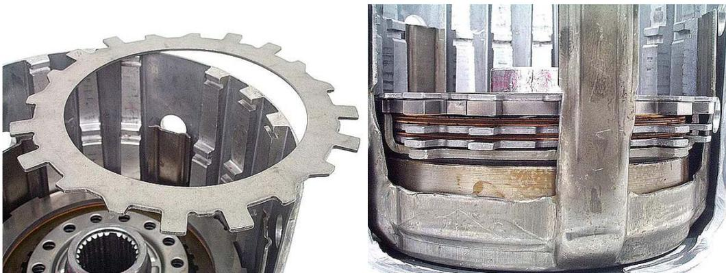
**Step 15:** Install the forward clutch plates, starting with a steel plate against the waved plate.
