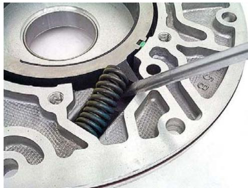
**Step 10:** Remove the pump slide from the pump pocket. Inspect the bottom of the pump pocket and the side of the pump pocket where the slide side seals rub. If there is any noticeable wear or scoring, the pump body must be replaced. Remove the slide side seals and slide top or bottom seal ring and rubber support ring. If the seal ring sticks in place, use an air nozzle to shoot air under/around it to unseat it.
