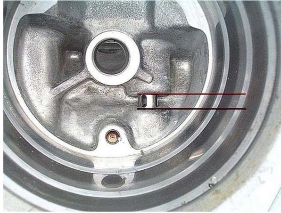
**Step 10:** To change the manual shaft seal, the manual shaft must be removed from the case.
