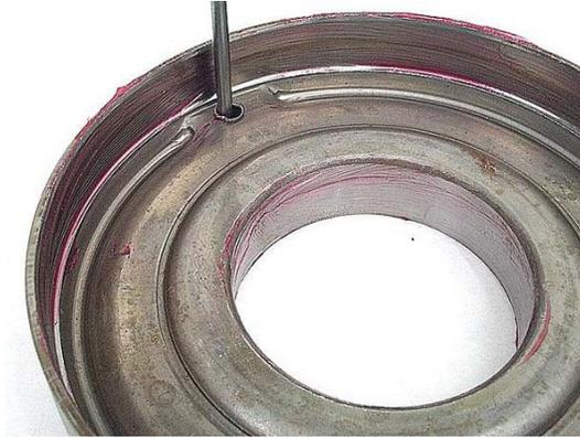
**Step 5:** Install a new forward steel piston into the piston housing. Although you may need a feeler blade to help push the seal into the housing, it can usually be installed by hand without tools. Try pushing the lip in with your thumbnail, if you have one.
