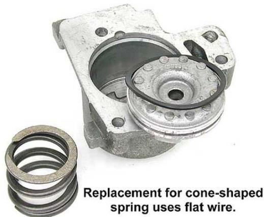
**NOTE:** If the 1-2 accumulator uses a cone-shaped spring, it must be replaced with the new style spring available from your parts supplier.
