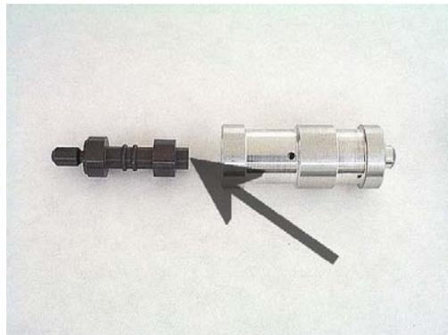
**Step 41:** Slide the pressure regulator valve and pressure regulator valve springs into the pressure regulator bore.
