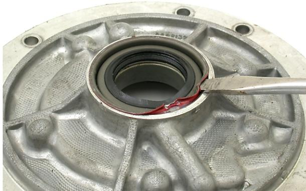
**Step 13:** Remove pump body o-ring if equipped.
