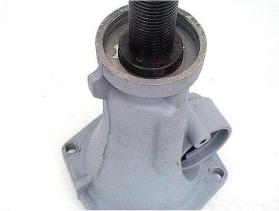
**Step 28:** Install a new bushing into the extension housing, being careful not to drive the bushing in at an angle. An arbor press is best to assure good alignment. You can use an old driveshaft yoke to check for proper bushing clearance.
