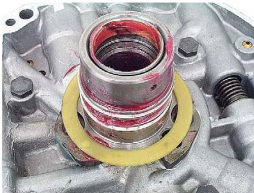
**Step 55:** Install the pump o-ring into the pump body groove without twisting it, making sure that the line on the OD of the ring is visible all the way around the pump.
