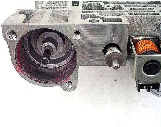
**Step 11:** Install the accumulator spring and the low overrun valve spring.
