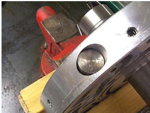
**Step 48:** Put the snap ring onto the snap ring pliers. Hold the snap ring over the TV boost valve sleeve. Use a screwdriver placed inside the snap ring to push the boost sleeves into the bore. Lower the snap ring into the bore, then release the snap ring into the bore groove.
