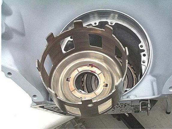
**Step 17:** Lower the sun gear shell into the case, engaging the shell inner teeth with the top outside teeth of the rear sun gear.
