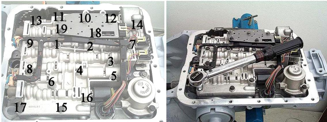
**Step 52:** Install the manual lever detent spring and bolt.
