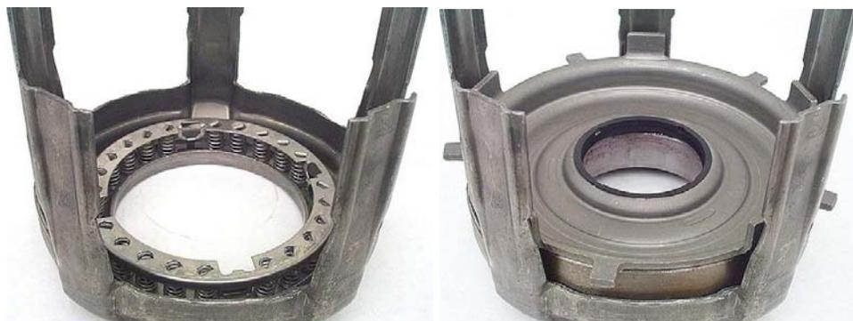
**Step 7:** Grab two fingers of the apply ring and lower it into the input drum with your thumbs, lining up the apply ring fingers with the wide slots inside the input drum.
