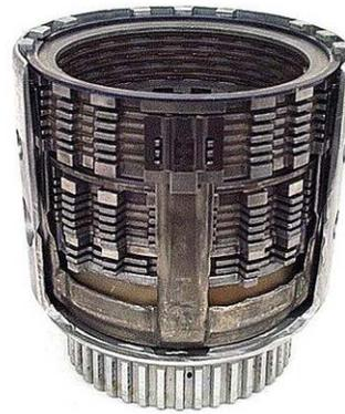
**NOTE:** To assist with easy viewing of the drum's internal parts, the drum shown has been cut open to expose the clutch and piston areas, and the turbine shaft has been removed. If your drum looks like this one, it's in serious trouble.
