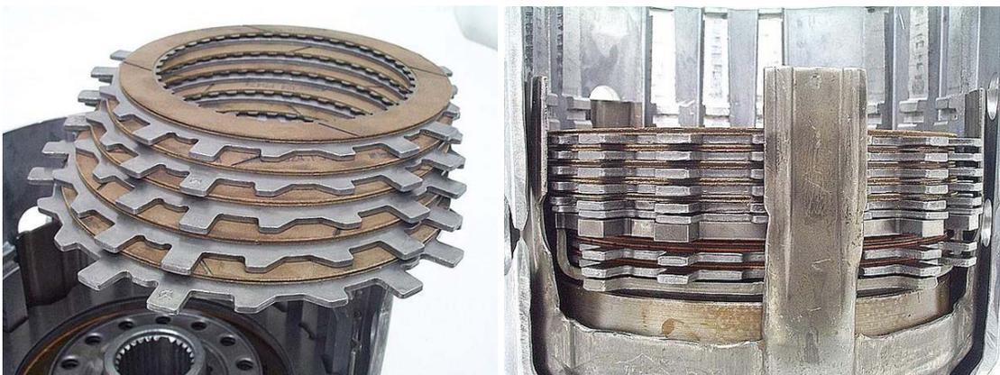
**Step 16:** Install the forward clutch pressure plate and snap ring.
