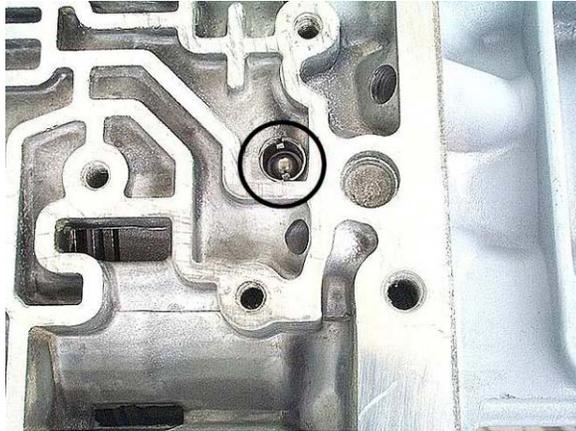
**Case Checkballs, 4L60:** Place the case checkballs in the locations shown. The checkball marked with a '\*' is only used if the separator plate has two holes over the case pocket.
