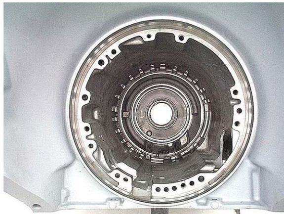
**Step 13:** Thoroughly clean the case. Blow any standing water or cleaning solution out of the case passages rather than let it drip dry. This keeps any cleaning machine deposits from contaminating the new ATF or causing valves to stick after the unit goes back into the vehicle.
