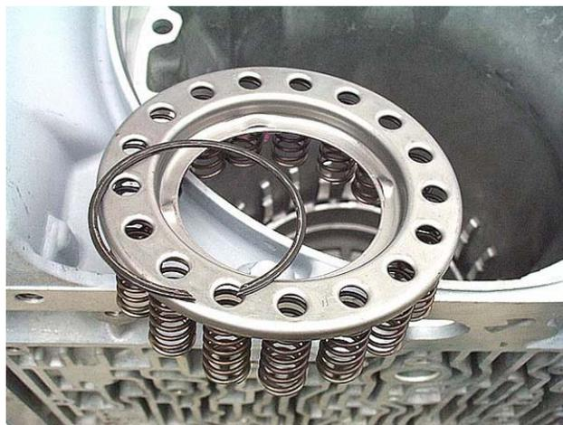
**Step 39:** Blow compressed air into the passage shown to pop the low-reverse piston out of its case bore. Remove the piston from the case. Remove the seals from the piston.
