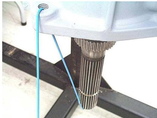
**Step 22:** Install the snap ring into the output shaft groove above the front planetary carrier. You may have to push up on the back end of the output shaft to expose the entire snap ring groove. With the snap ring in place, remove the piece of coat hanger holding the output shaft in place.
