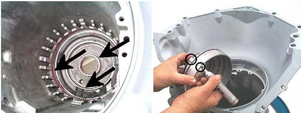
**Step 3:** Using a hammer handle, gently tap the piston into position in the case bore. Be extremely careful, because these seals rip very easily during installation, and ripped low-reverse seals are one of the most common after rebuild complaints for this unit. You will know when the piston is all the way down when you can see the outer seal bore above the edge of the piston near the park pawl.
