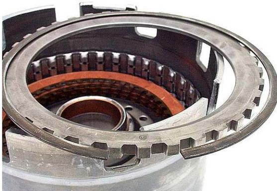
**Step 12:** Measure the clutch clearance between the pressure plate and the snap ring. This clearance must be between 0.040" and 0.076" (1.02mm-1.94mm). If your clearance is not within these specifications, adjust the clearance by installing the correct pressure plate. The available pressure plate thicknesses are:
