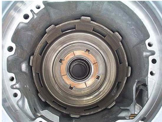
**Step 18:** Place the front planetary carrier rear thrust bearing in position on the back of the planetary carrier, using assembly lube to hold the bearing in place. Install the planetary carrier into the front ring gear and hub assembly.
