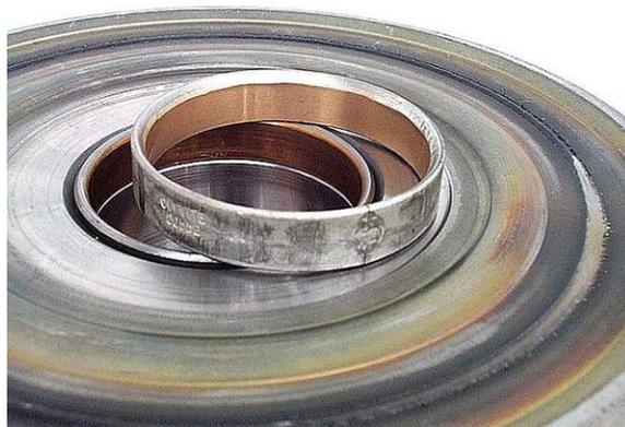
If the drum appears okay but the band surface is glazed mirror smooth, you may resurface the band apply area on the drum, but don't use anything coarser than #400 grit emery cloth or ScotchBrite™. You do NOT want a rough surface on this drum.
