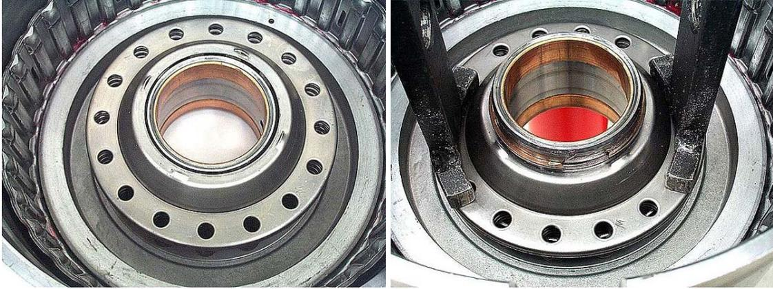
**Step 9:** Place the cushion plate onto the piston, dished side down.
