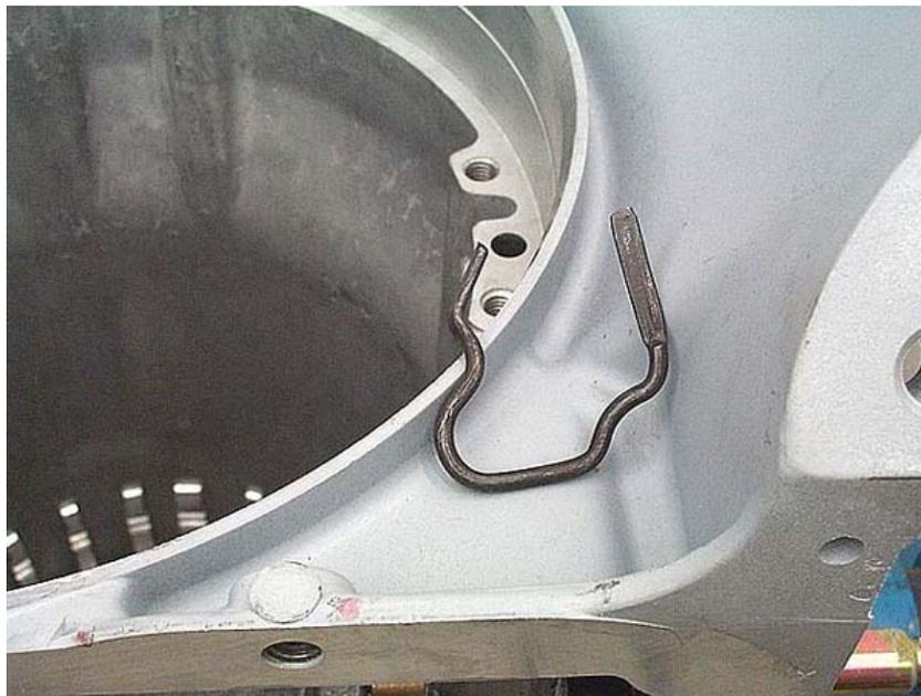
**Step 38:** Using a suitable return spring compressor, compress the low-reverse clutch return spring assembly and remove the retaining snap ring. Release the compressor and remove the compressor and return spring assembly from the case.
