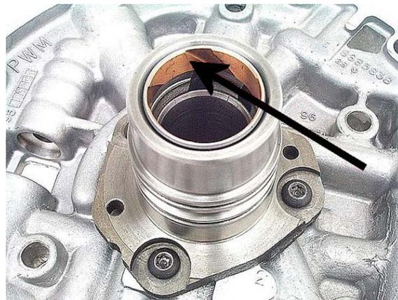
**Step 34:** Flat sand the passages of the stator support, paying close attention to the areas near the bolt holes.
