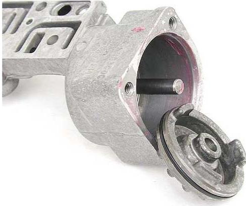
**Step 11:** Install spring onto the piston, then install the cover and hand-tighten the bolts snugly.
