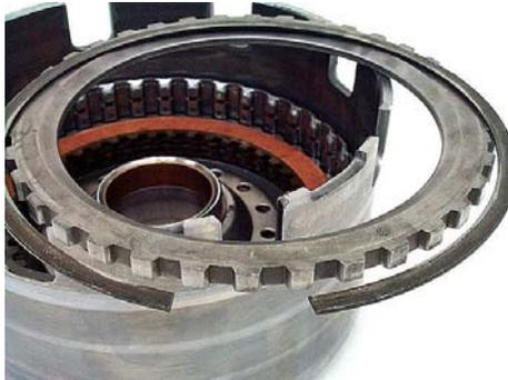
**Step 2:** Remove the clutch friction and steel plates, followed by the dished cushion plate.
