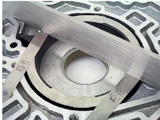
**Step 21:** The pump rotor and slide come in selective thicknesses. If either have to be replaced, be sure to get the correct thickness. If the clearance is close but not within these specifications, sand or replace the parts as necessary. If the clearance is too tight, flat sand the rotor or slide until the clearance is correct. If the clearance is too loose, you can flat sand the pump body to tighten up the clearance. Be certain to clean the parts after any sanding operation.
