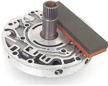
**Step 35:** Install a new pump output screen into the side of the stator support. The replacement screen may be a different color, but should function properly. If you're reusing the screen, make sure that you put a new o-ring on it. It's got to seal against main line pressure.
