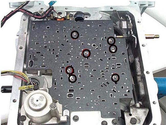
**Step 14:** Remove the TCC solenoid bolts, then remove the TCC solenoid from the unit. Remove the o-ring from the solenoid neck. Remove the harness case connector and harness from the case.
