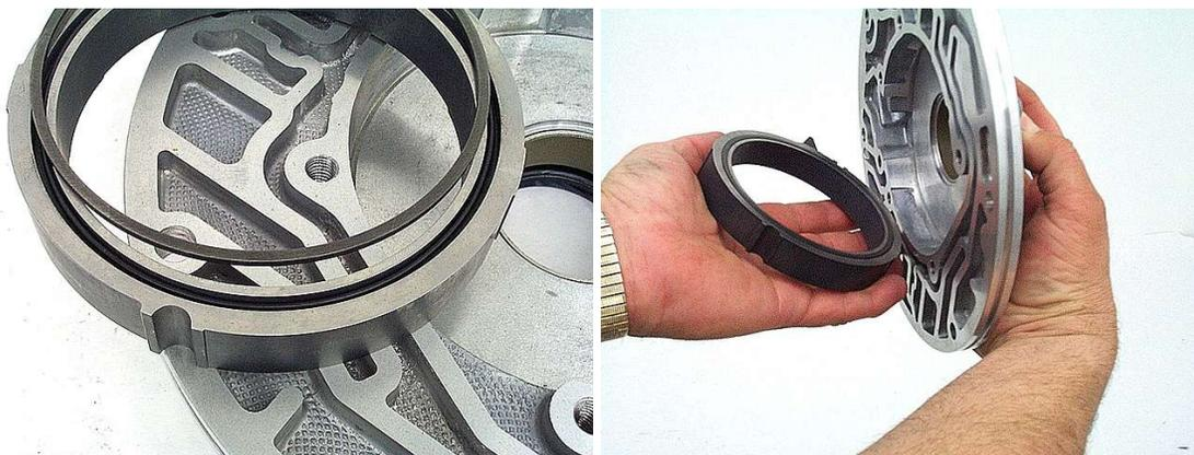
**Step 24:** With the pump on the bench and the slide facing up, install the slide side teflon seal and rubber support strip into the groove on the side of the pump slide. The teflon seal goes against the pump bore and the rubber strip goes into the slide groove.
