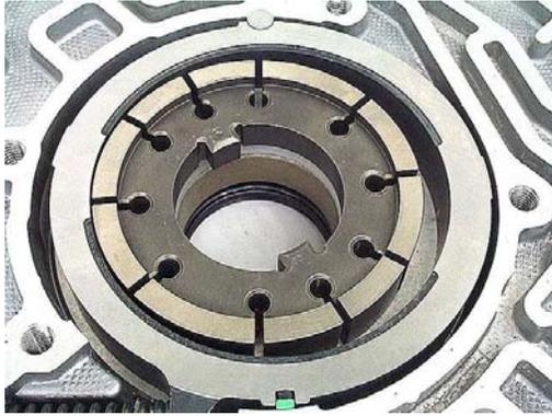
**Step 29:** If you are using used pump vanes, find the side of each vane that has two 'rub marks' from riding against the vane rings, and aim that side of each vane toward the center of the rotor. Install half of the pump vanes in a semi-circle, making sure that the vanes don't go on top of the bottom vane ring.
