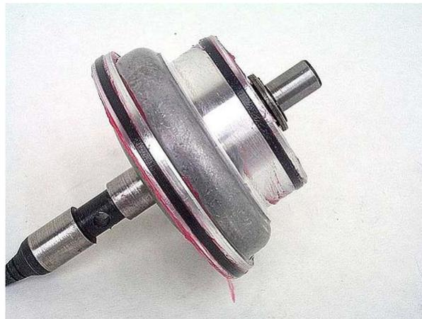
**Step 24:** Place a new rubber o-ring (the smaller of the two servo o-rings) onto the piston guide ring, then slide the guide ring over the small 2<sup>nd</sup> piston seal ring with the flat side of the guide ring facing toward the large 2<sup>nd</sup> piston seal ring. Be careful to guide the smaller 2<sup>nd</sup> piston seal ring into the guide ring without cutting the seal ring.
