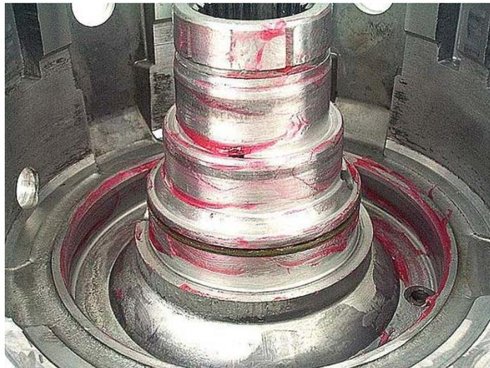
**Step 3:** If you have an aluminum 3-4 piston, install new lip seals into the piston seal grooves, then install the piston into the input drum. If you're not using an aluminum 3-4 piston, install a new molded piston.
