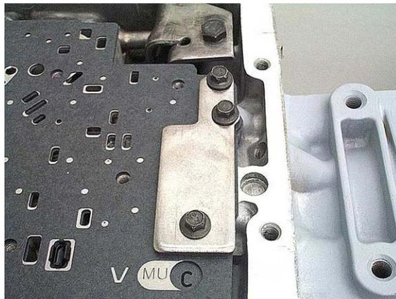
**87 & later 4L60-** Put the checkball into the auxiliary valve body using assembly lube to hold it in place. Set the separator stiffener plate or auxiliary valve body into position on the separator plate and install the bolts, tightening them to 8 ft-lbs.
