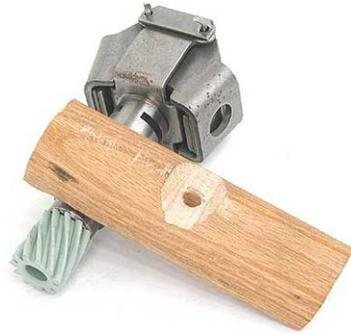
**Step 19:** Remove the roll pin holding the gear to the shaft.
