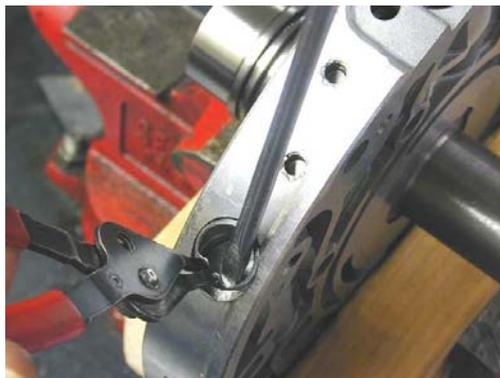
If you can't get the snap ring all the way into the groove this way, release the snap ring as far down in the bore as possible. Use another small screwdriver to press the snap ring the rest of the way into the groove until the snap ring is firmly locked into its groove.
