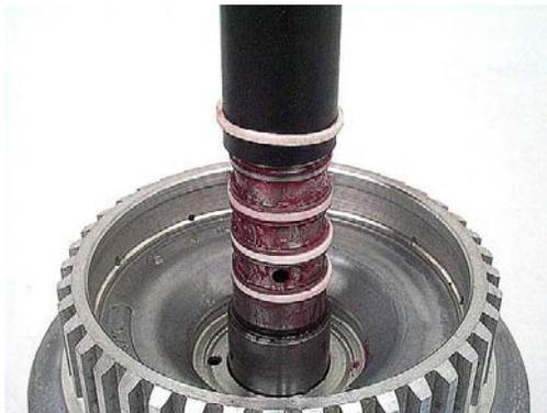
**Step 26:** Place the endplay shim and thrust bearing into position over the turbine shaft as shown, using assembly lube to hold them in place.
