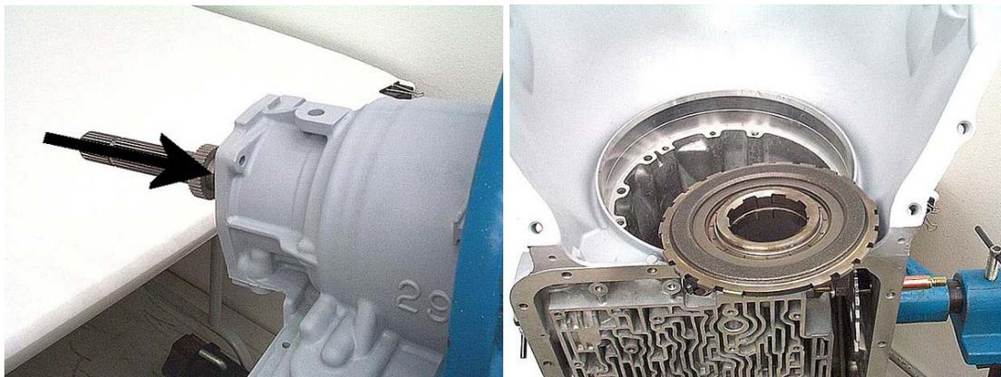
**Step 35:** Remove the rear planet from the case. Some of the low-reverse clutch plates may come out with it.
