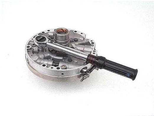
**IMPORTANT:** After the pump body and stator support are bolted together, make sure that the rotor can be turned by hand using the pump shaft, a converter hub, a pick or other suitable tool. Be very careful not to nick the front seal or bushing. If the rotor won't turn, disassemble and re-check your slide and rotor clearances.
