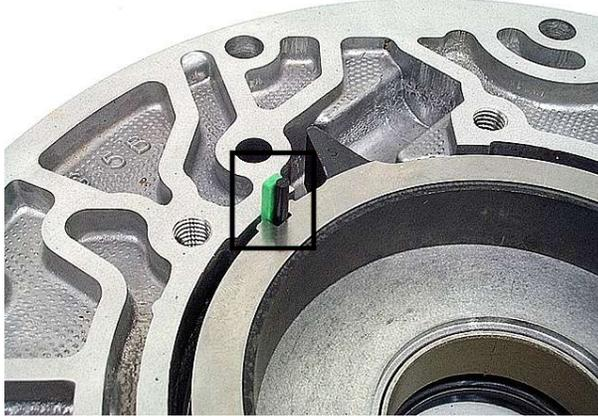
**Step 25:** Pressing the slide toward the side seals to compress the rubber support strip, install the pump slide swivel pin spring and swivel pin.
