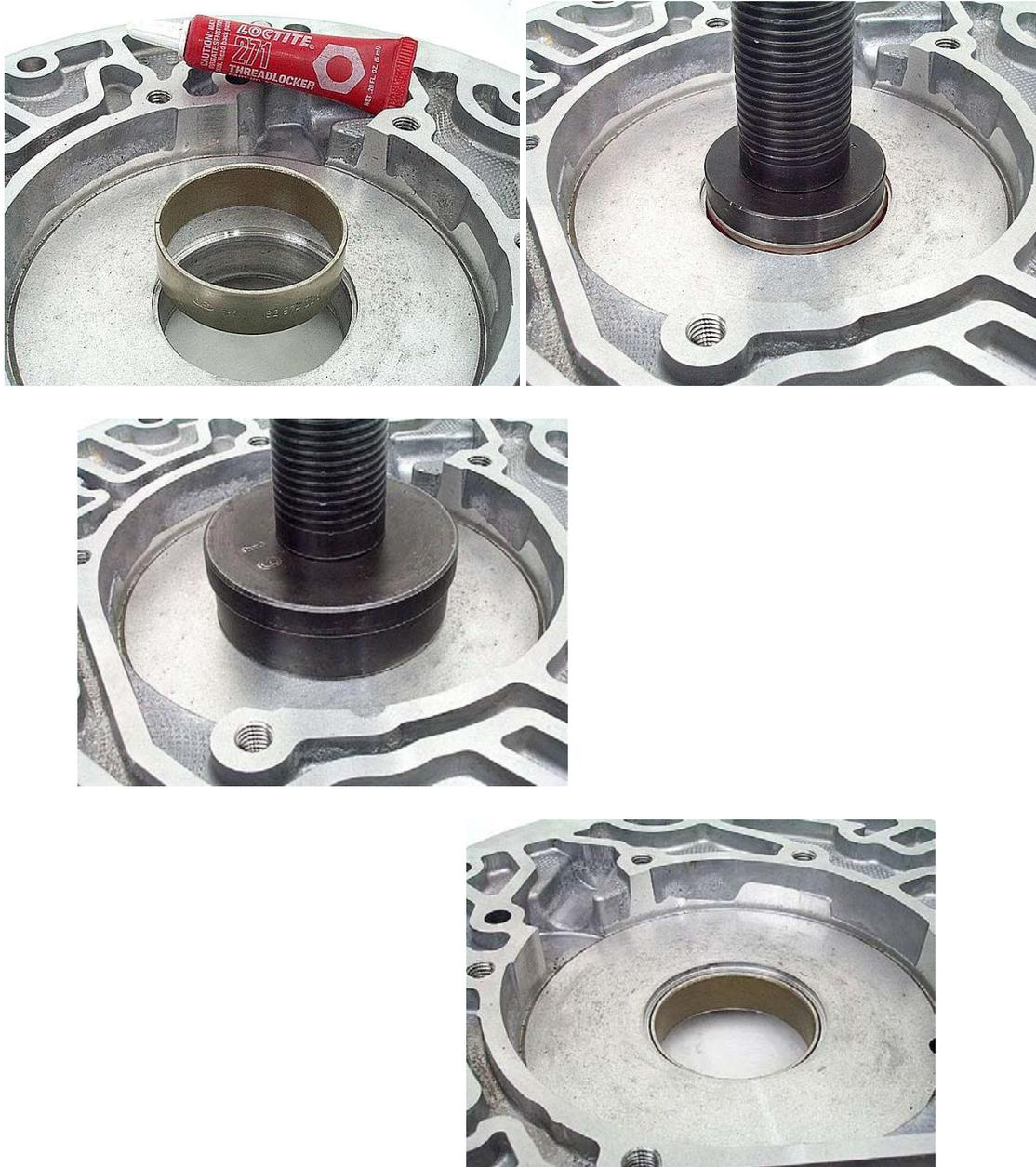
**CAUTION:** Make certain that you wipe off **any** excess locking compound from the bushing after pressing it into place. If any of this compound gets into the pump rotor area, a destroyed pump is practically assured.
