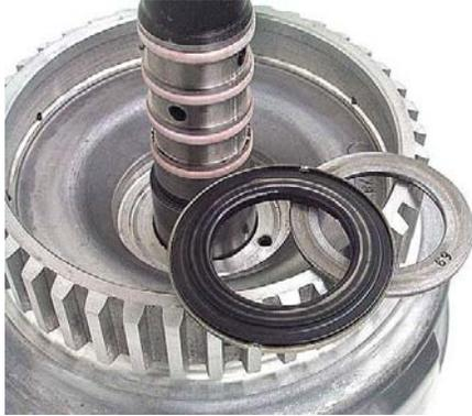
**Step 2:** Inspect the three turbine shaft bushing journals for wear or damage. If problems are found, replace the drum.
