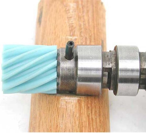
**Step 25:** Use a chisel to stake the roll pin holes so that the pin can't work its way out of the shaft.
