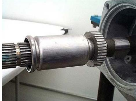
**Step 68:** Install a new lathe-cut seal on the extension housing if one hasn't already been installed. Make sure that the extension housing's speed sensor or speedometer cable adapter hole is aimed toward the same side of the case that the manual shaft is on, then tap the extension housing into place on the back of the case. Torque the four housing bolts to 26 ft-lbs.
