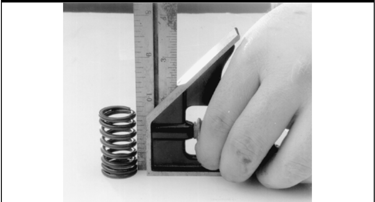
Check the valve spring for squareness on a flat surface; a carpenter's square can be used
