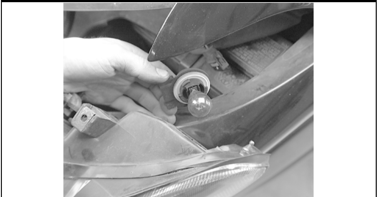
Turn the side marker bulb socket counterclockwise and pull it out of the module
