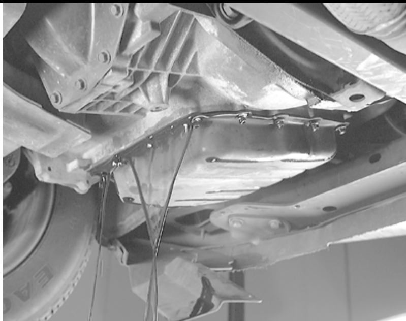
Allow the pan to hang down slightly, enabling the fluid to drain into a suitable container
