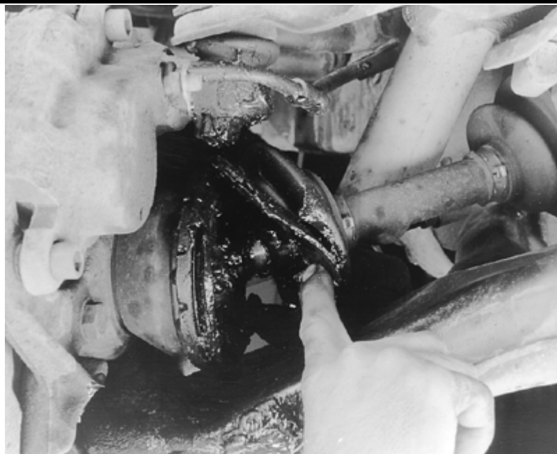
CV-boots must be inspected periodically for damage
