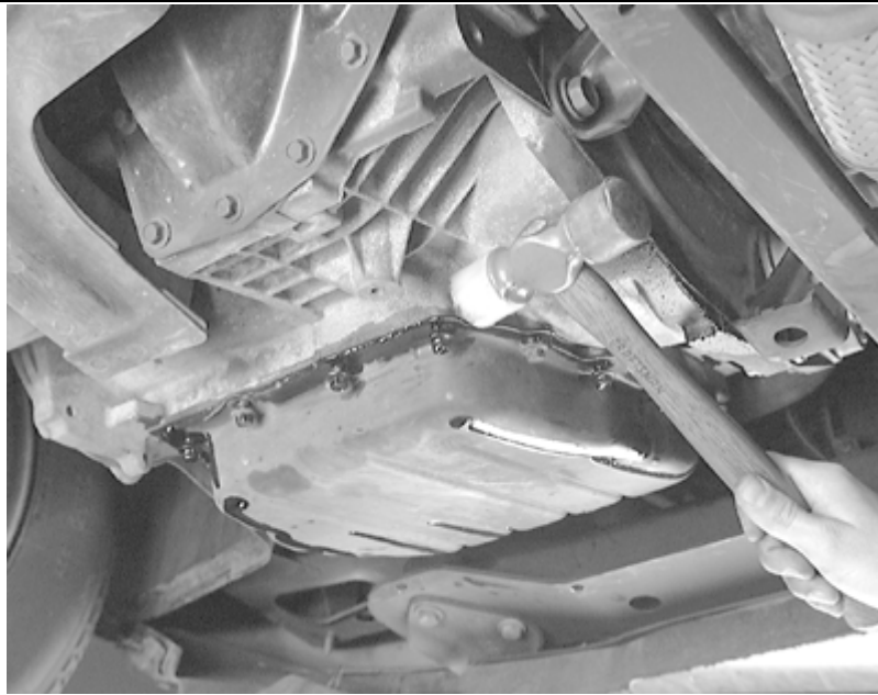
Tap the pan loose with a rubber faced hammer
