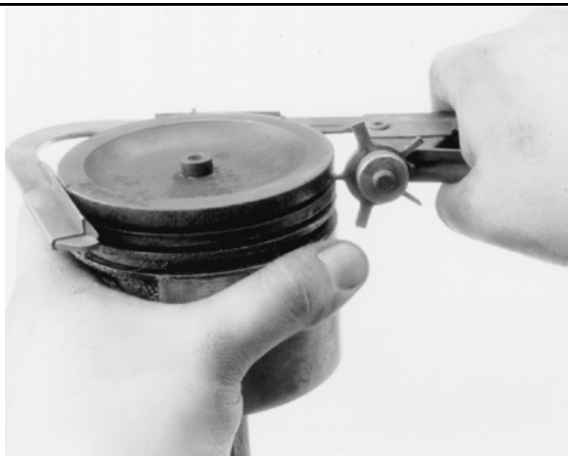
Clean the piston ring grooves using a ring groove cleaner tool, or ...
