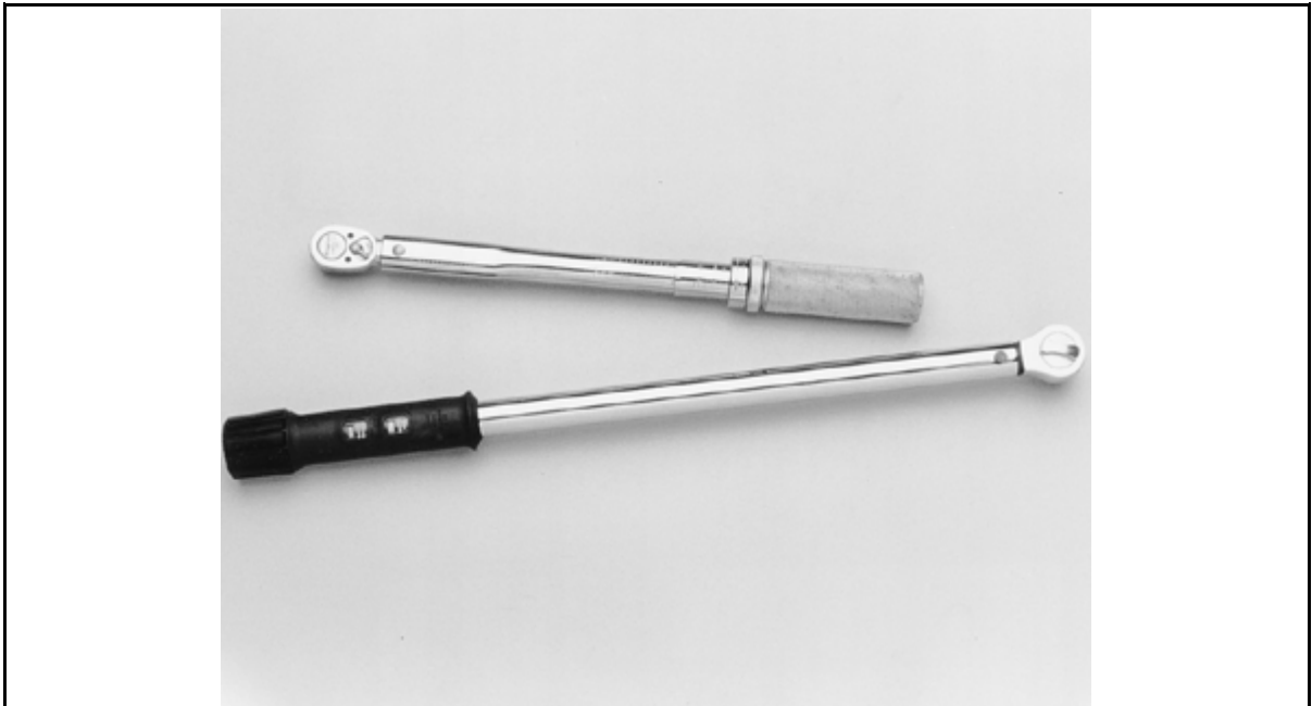
Many repairs will require the use of a torque wrench to assure the components are properly fastened
