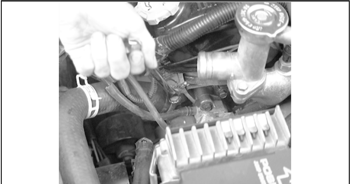
On the front cylinder head, remove the grounding strap
