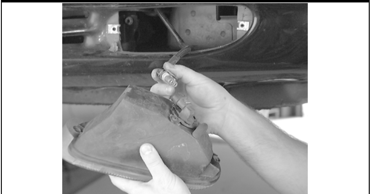
Pull the fog lamp out of the front fascia panel and disengage the wiring connector
