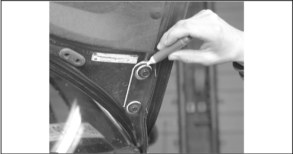
For installation purposes, be sure to matchmark the correct hood mounting bolt-to-hinge position on each side of the hood
