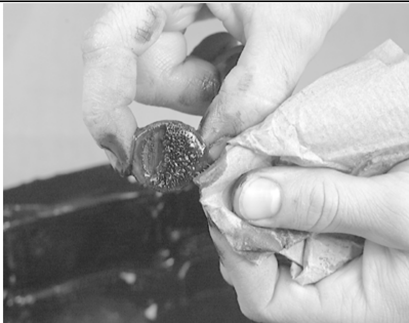
Clean the oil pan magnet of any metallic shavings
