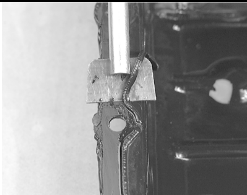
Clean the oil pan of all old gasket material using an appropriate surface scraping tool
