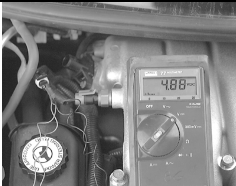
Testing for reference voltage to the MAP sensor
