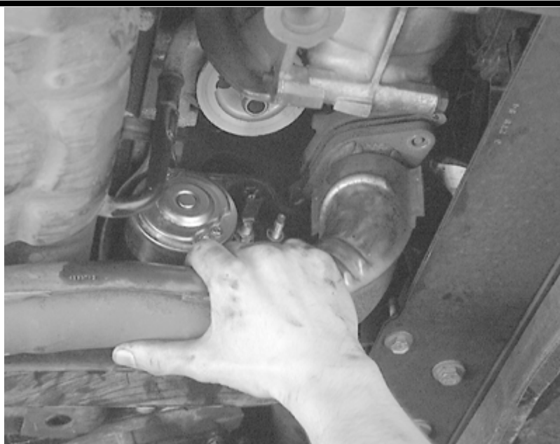
Pull the exhaust pipe down just enough to provide removal clearance for the starter
