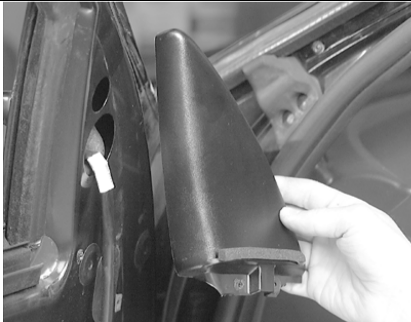
Remove the side view mirror interior trim panel from the door
