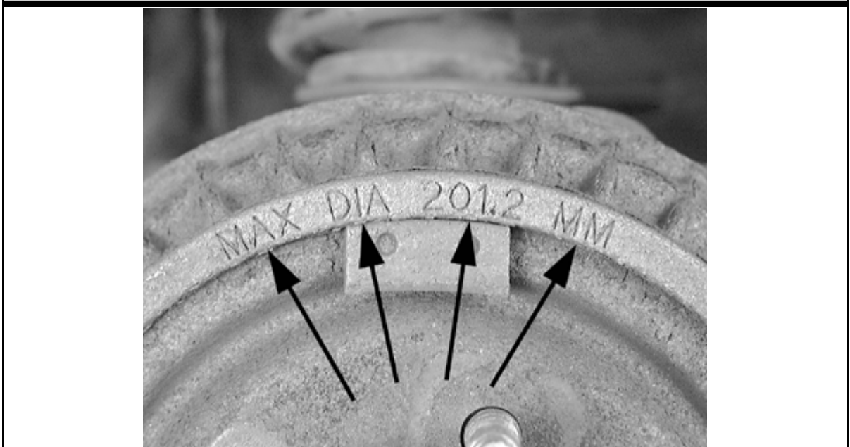
The maximum machining diameter is cast into the outer rim of the brake drum
