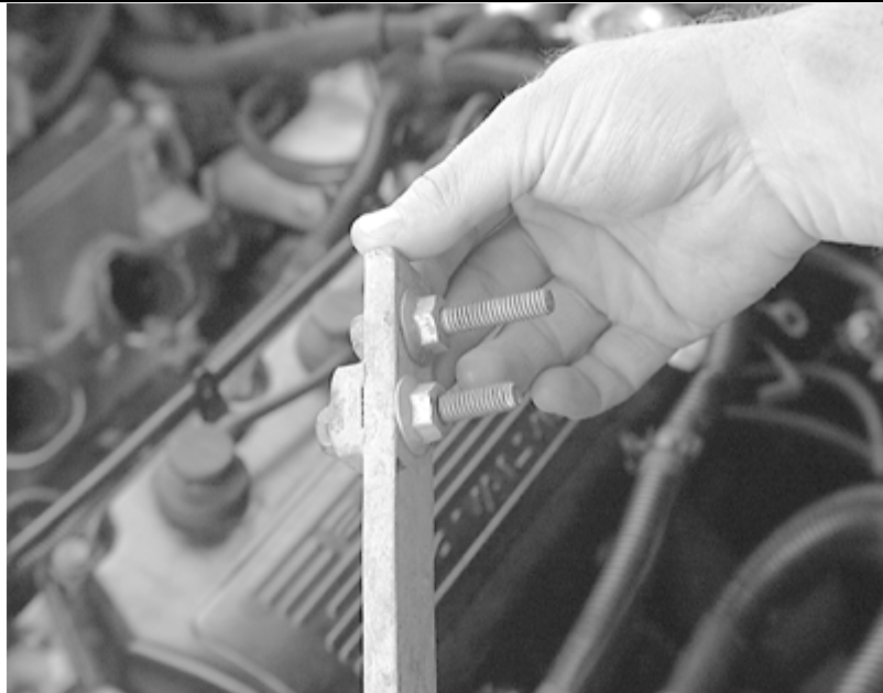
If a sprocket holding tool is not available, one can be fabricated with a couple of nuts, long bolts and a thick, long piece of metal stock
