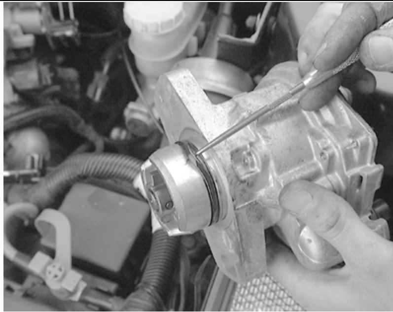
Inspecting the distributor shaft rubber O-ring seal for nicks or cracks
