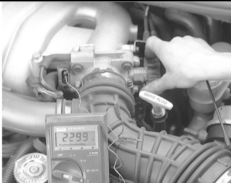
While checking resistance of the TPS, readings should change smoothly in proportion to the opening angle of the throttle lever
