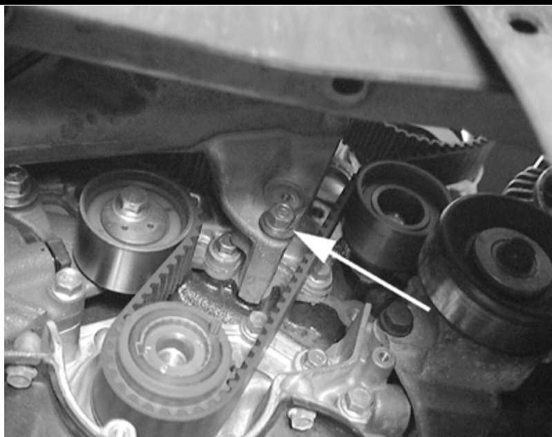
When removing the right side engine mount assembly to access the timing belt, this mounting bolt is hidden by the lower timing belt cover
