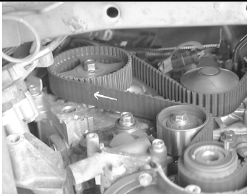
Mark the rotational direction of the timing belt if it is being removed and reused
