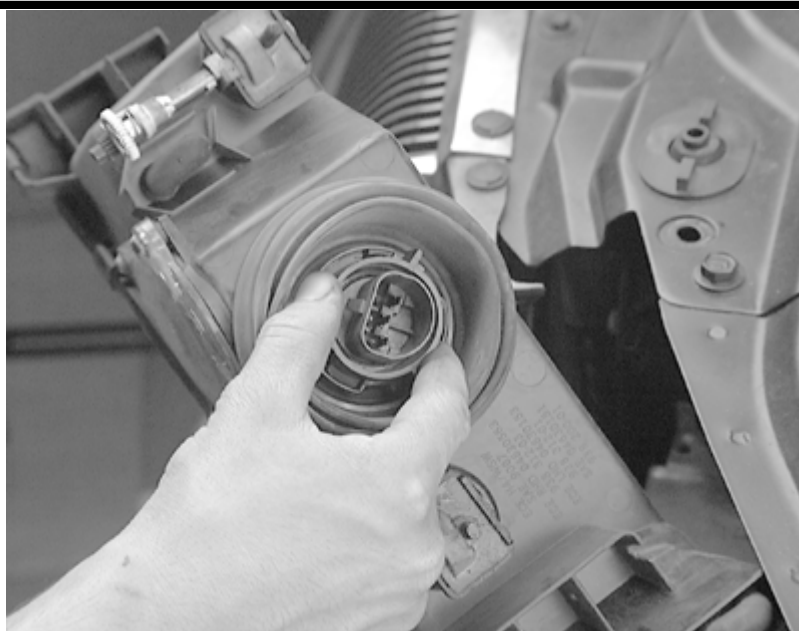
Turn the light bulb retaining ring counterclockwise, and remove it from the back of the module
