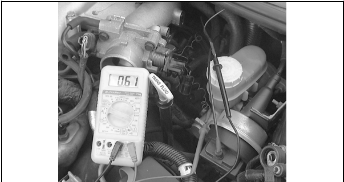
Using a DVOM connected to jumper wires to test the ignition coil on the distributor housing
