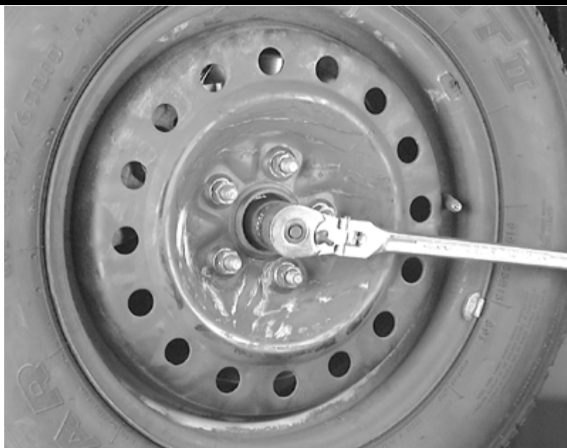
Loosen the hub nut with the vehicle on the floor and the brakes applied
