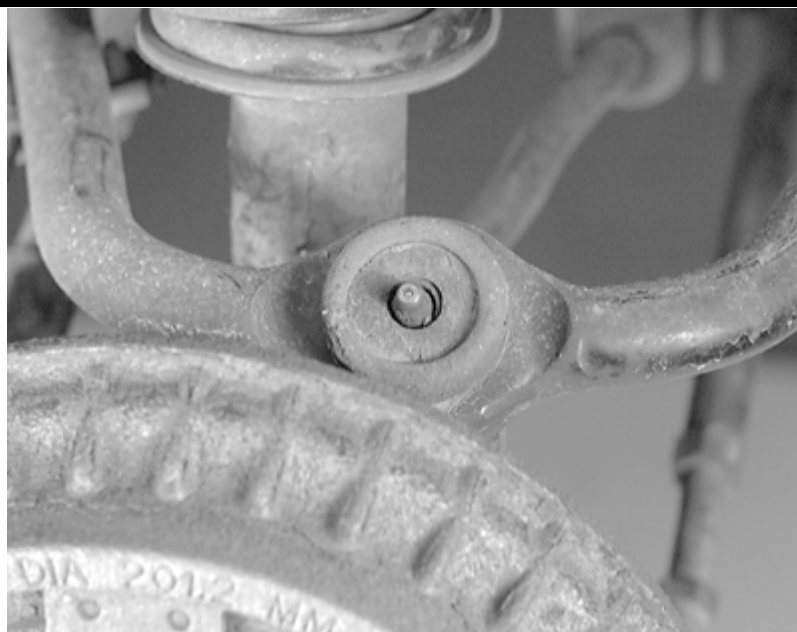
Location of the rear ball joint grease fitting on top of the rear upper control arm
