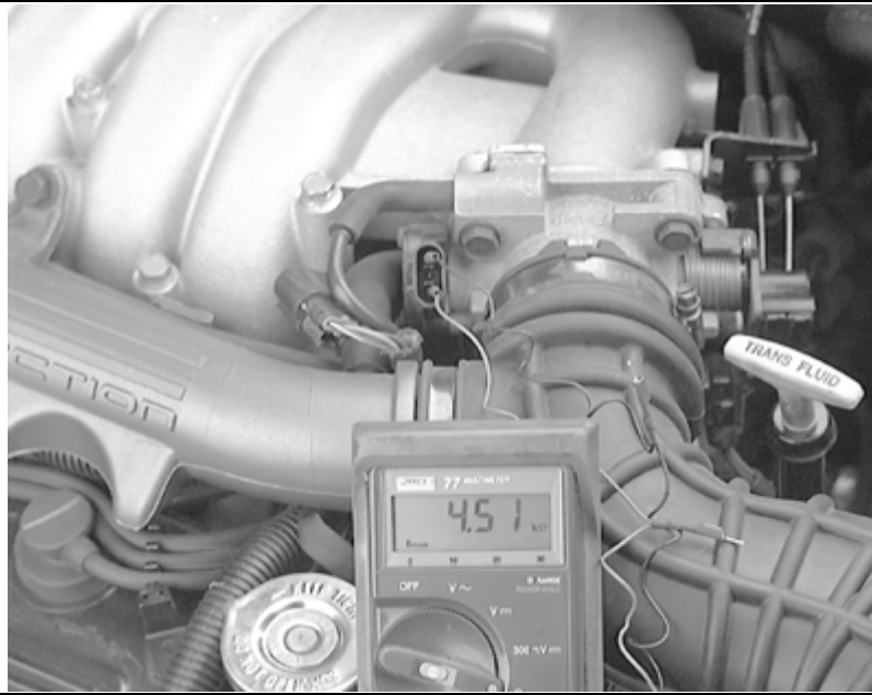
Checking resistance of the TPS, which reads 4.51K ohms with the throttle lever closed
