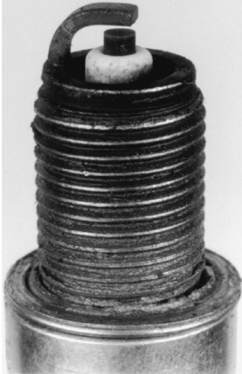
A normally worn spark plug should have light tan or gray deposits on the firing tip
