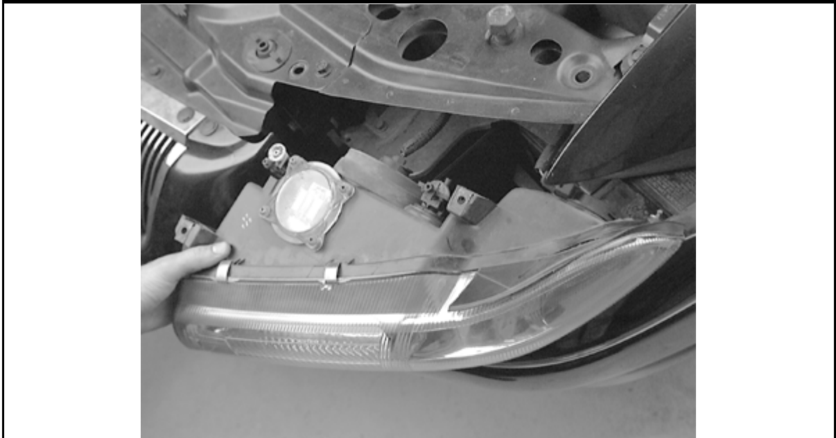
Pull the headlight module straight out of the front of the vehicle to remove the bulbs
