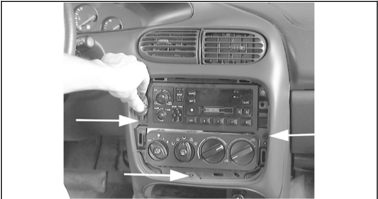
Remove the 3 attaching screws under the center trim bezel
