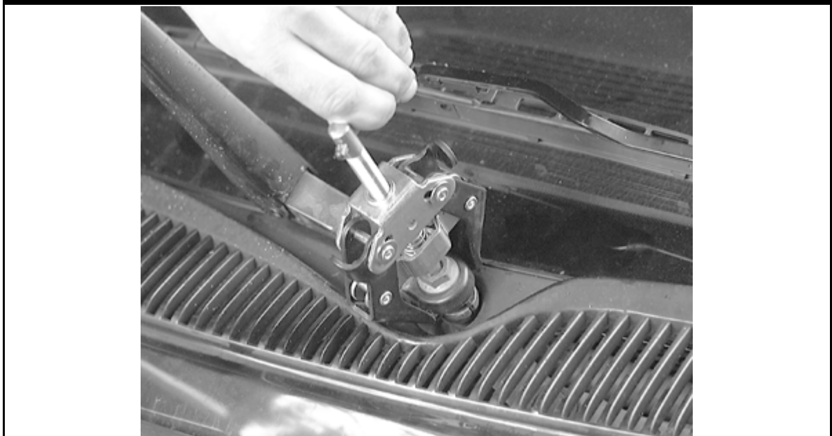
Removing the wiper arm assembly with a puller tool
