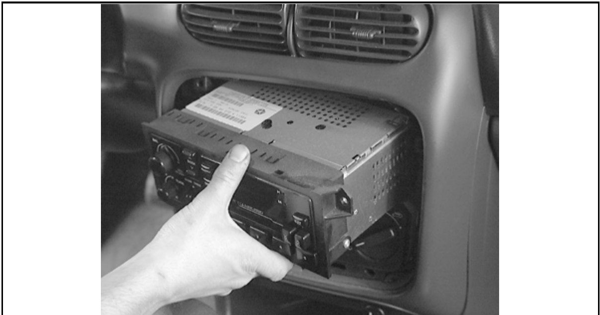
Removal of the radio unit from the instrument panel
