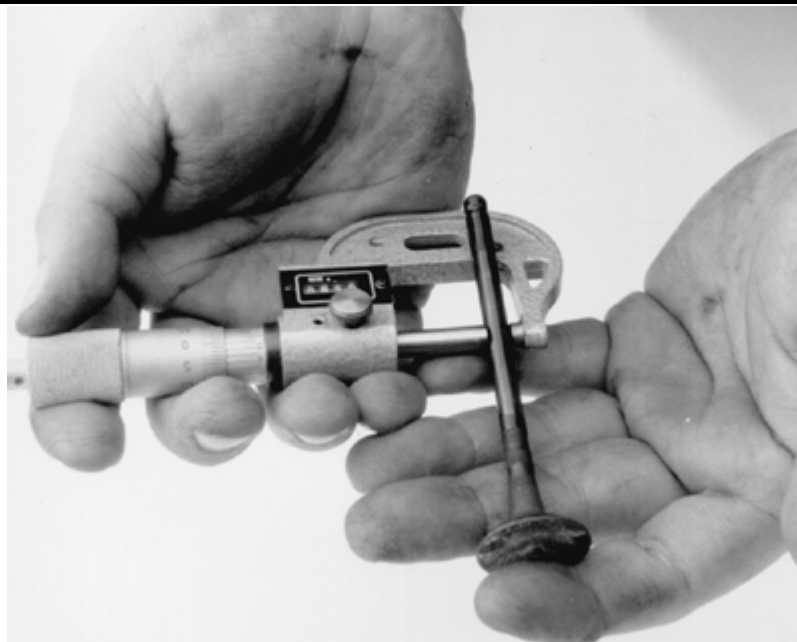
Use a micrometer to check the valve stem diameter
