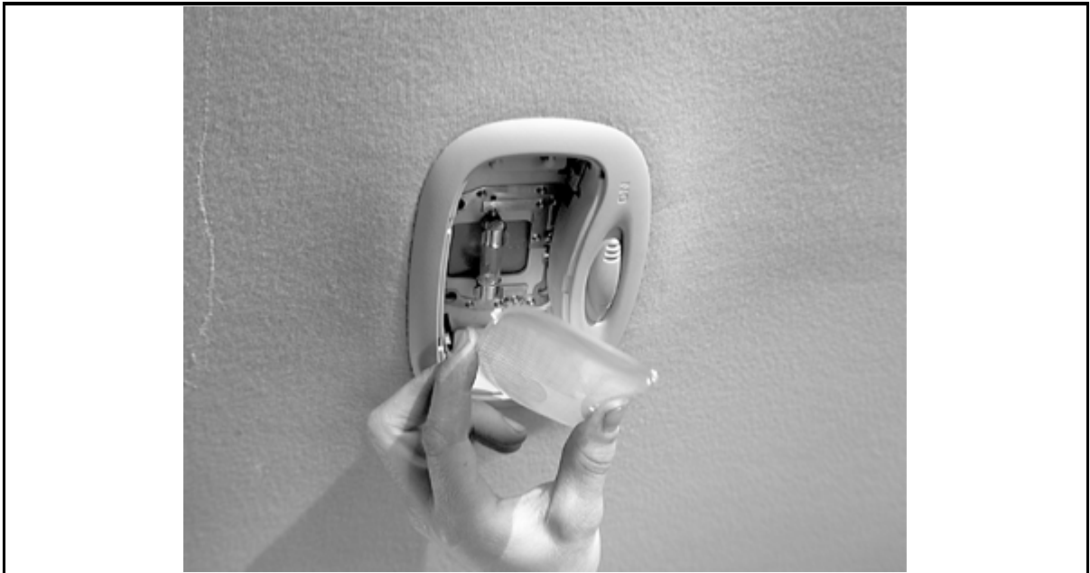
Removal of the middle interior dome light lens
