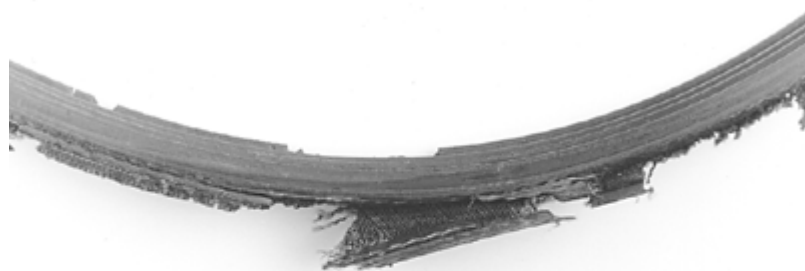
The cover of this belt is worn, exposing the critical reinforcing cords to excessive wear
