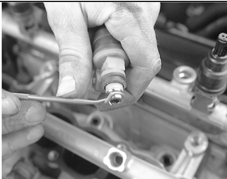
Use a small awl, or equivalent, to remove the fuel injector O-ring gaskets
