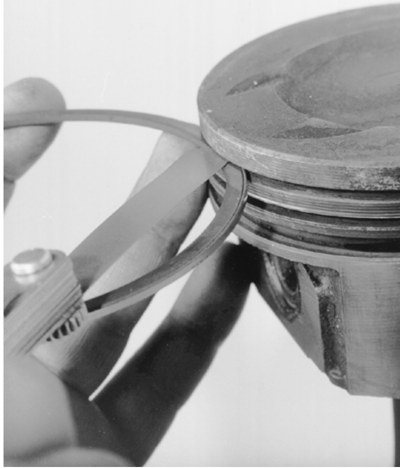
Checking the piston ring-to-ring groove side clearance using the ring and a feeler gauge
