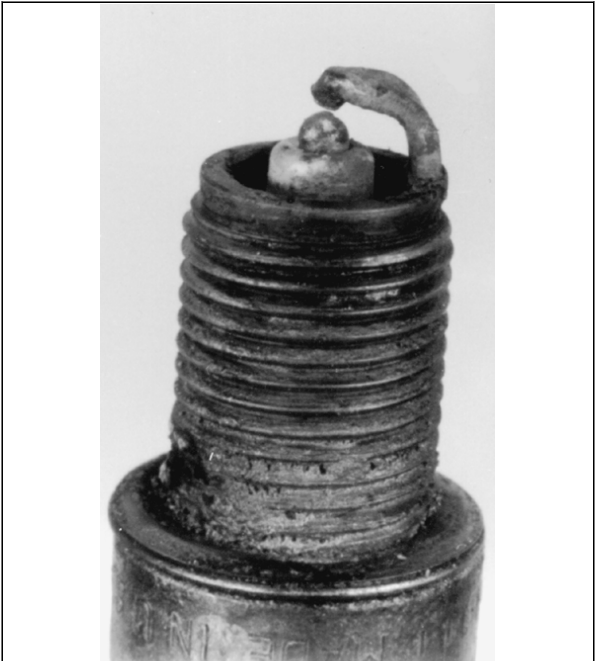
A bridged or almost bridged spark plug, identified by a build-up between the electrodes caused by excessive carbon or oil build-up on the plug
