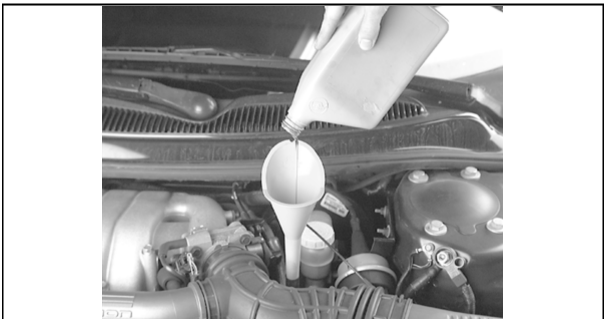
To avoid a mess in the engine compartment and on the ground, always use a funnel when pouring automatic transmission fluid into the transaxle
