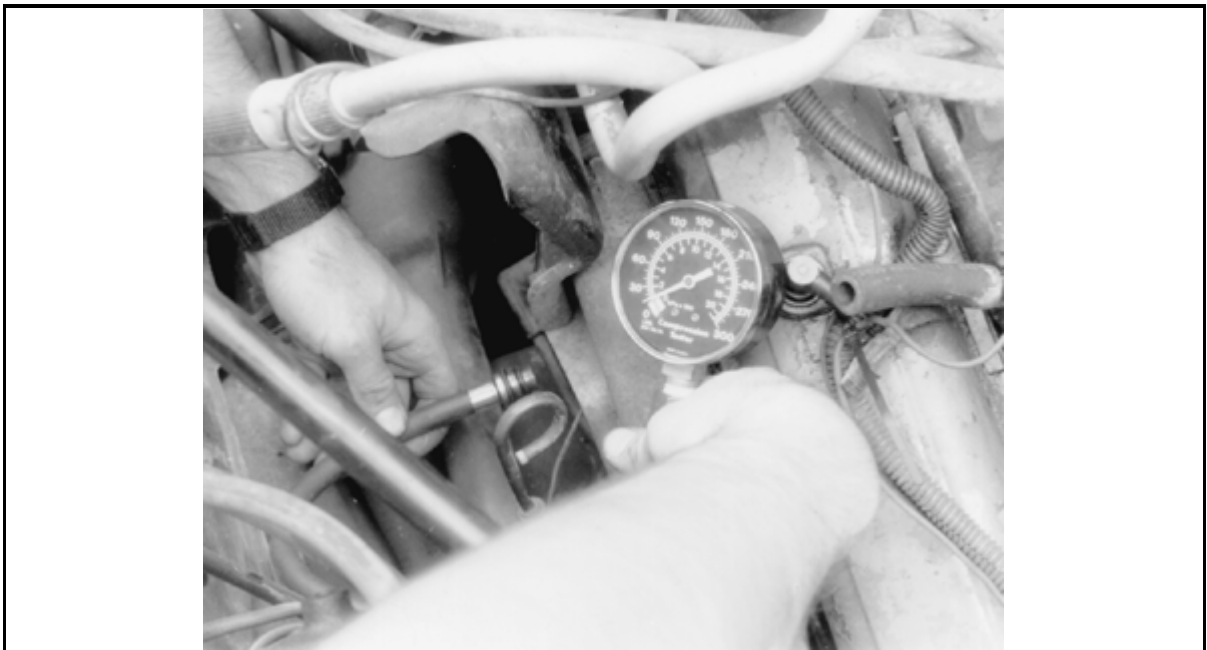
A screw-in type compression gauge is more accurate and easier to use without an assistant
