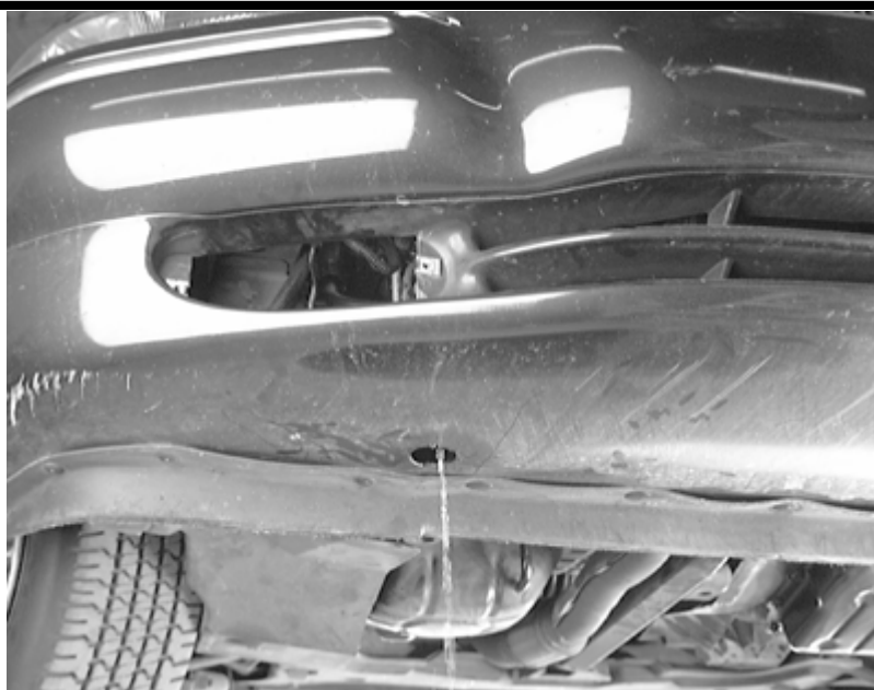
Coolant draining through an opening and into a suitable container
