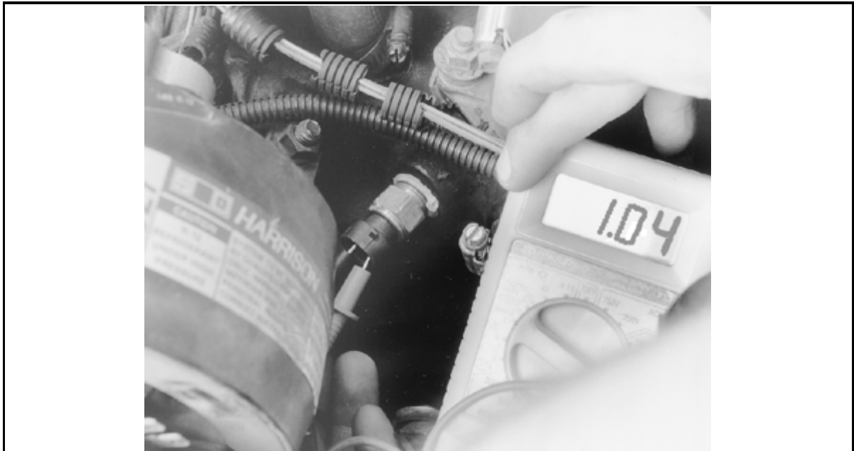
Checking the resistance of a coolant temperature sensor with an ohmmeter. Reading is 1.04 kilohms
