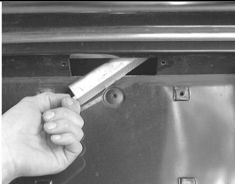
Carefully pull out the license plate light module from inside the trunk lid
