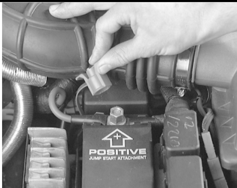
Location of the positive battery cable remote connection behind the engine compartment fuse box
