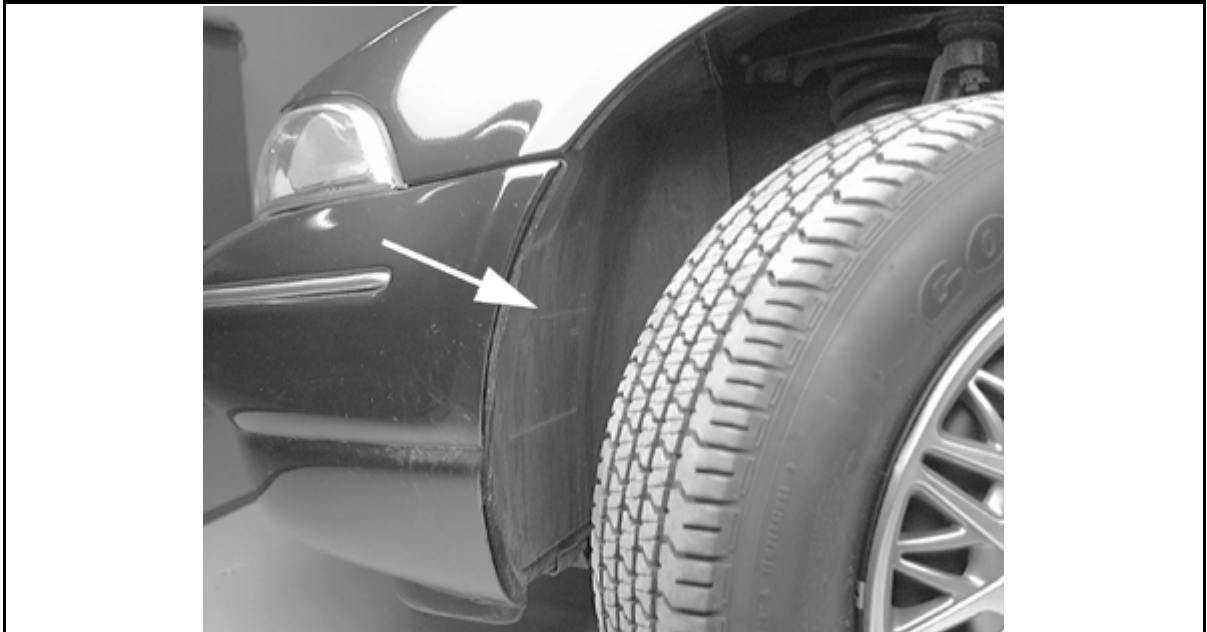
The Cirrus' battery is located behind the access panel, just ahead of the left front wheel-Stratus, Breeze and Sebring convertible similar
