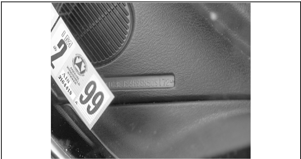
Location of the Vehicle Identification Number (VIN) code plate at the left side of the instrument panel
