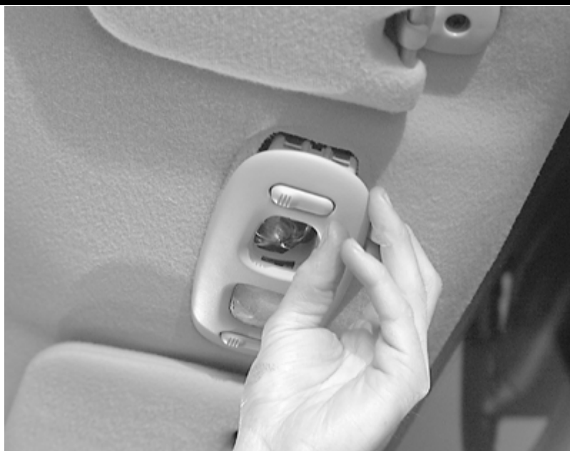
Pull the front dome light fixture down from the headliner by disengaging the retaining clips
