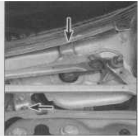
11.8a Wiper motor/linkage mounting bolts (arrows) - left side
