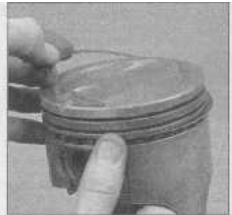
24.9b DO NOT use a piston ring installation tool when installing the oil control side rails
