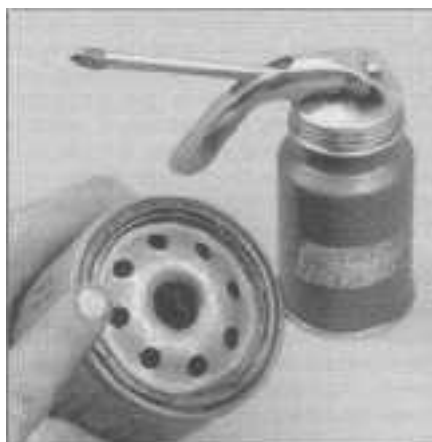
8.18 Lubricate the oil filter gasket with clean engine oil before installing the filter on the engine
