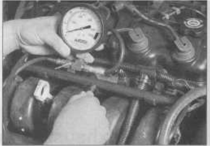
3.4 On four-cylinder engines, connect a fuel pressure gauge to the fuel rail at the test port
