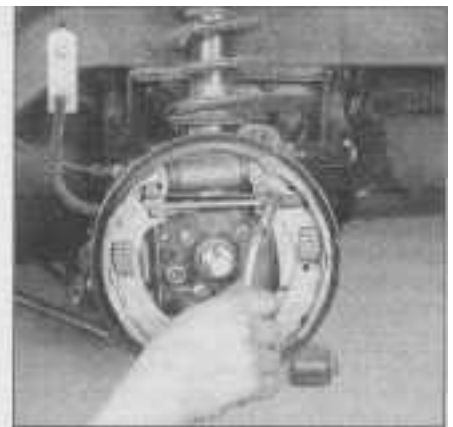
6.4u Install the upper return spring
