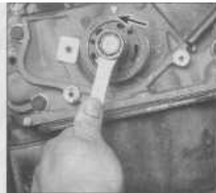
6.21a On 2.0L engines, use a box-end wrench or socket to rotate the crankshaft timing sprocket until the TDC mark on the sprocket is aligned with the arrow on the oil pump housing (arrow) . . .
