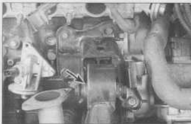
17.9a Front engine mount (arrow) - exhaust manifold removed for clarity
