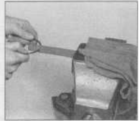
24.5 If the ring end gap is too small, clamp a file in a vise as shown and file the piston ring ends - be sure to remove all raised material
