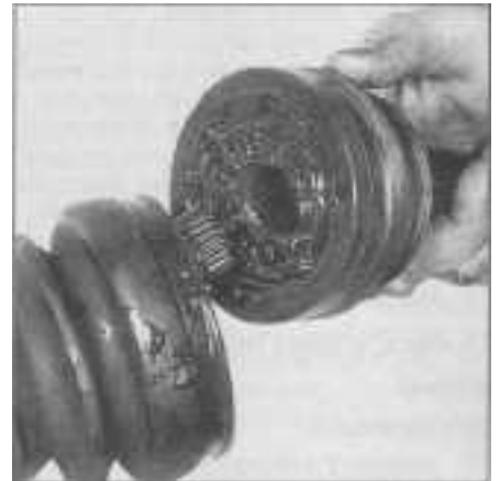
9.5b ... and remove the outer CV joint from the axle shaft
