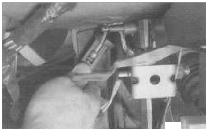
3.5c ... and remove the up-stop/spacer from the clutch cable end
