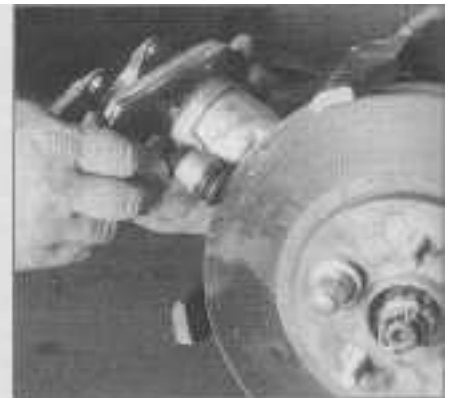
3.4i Install the inner brake pad - make sure the retaining spring is fully seated into the piston bore
