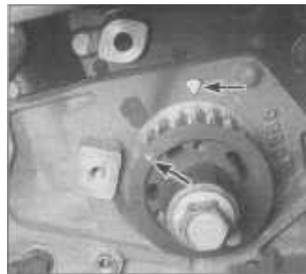
6.21b . . . then back it off counterclockwise 3 teeth BTDC (arrows)
