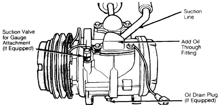
If the compressor on your vehicle has a drain plug, remove it and drain the oil, then reinstall the plug with a new O-ring - if it doesn't have a drain plug, you will have to remove the compressor, turn it upside down and drain the oil out of the suction and discharge ports
