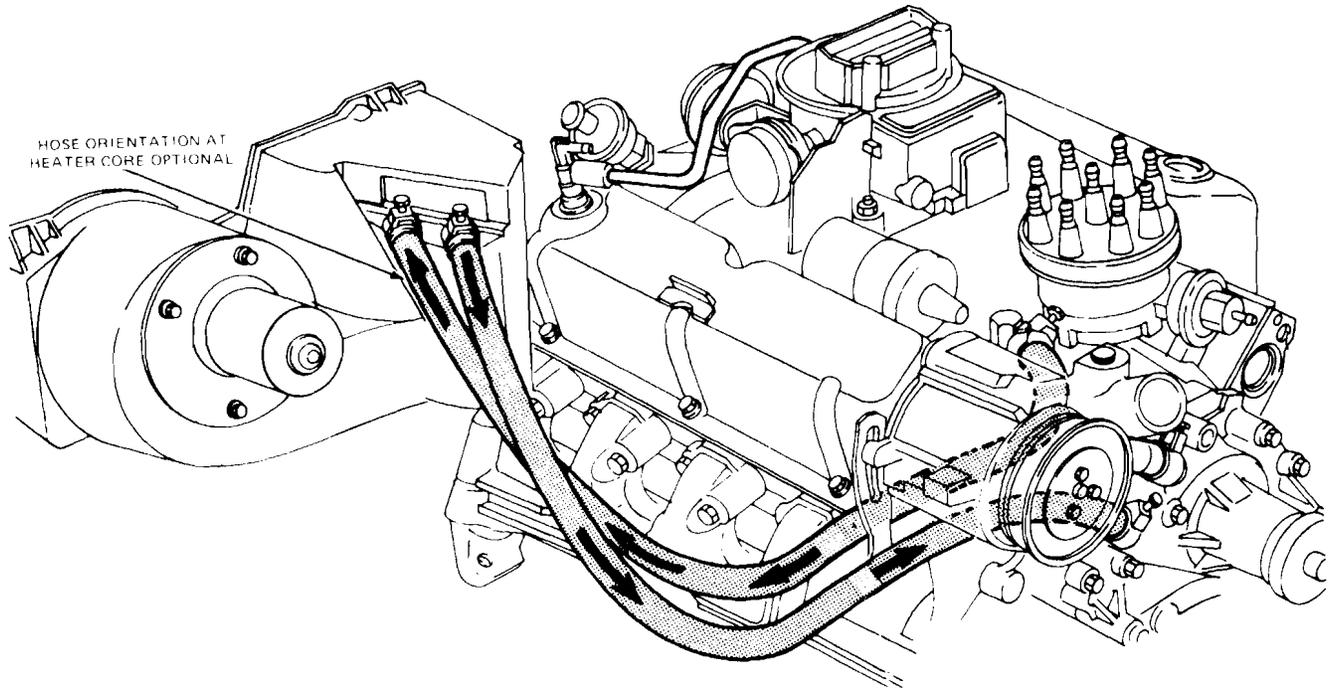
The easiest way to find the heater hoses is to locate them where they come out of the firewall, then trace them forward and detach them from the water pump and intake manifold (or block) - as a rule of thumb, you should force clean water through the heater hoses and the heater core in the direction opposite normal flow (the hose attached to the water pump carries coolant back to the engine, so that's the one you want to use)
