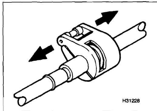
. . . and simultaneously pull the two pipes apart
