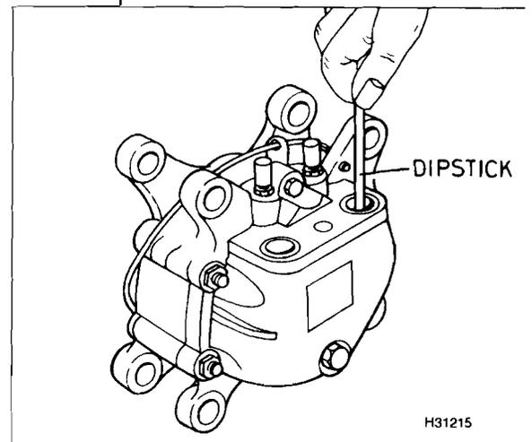
Using a dipstick to check the oil level on a York rotary vane compressor
