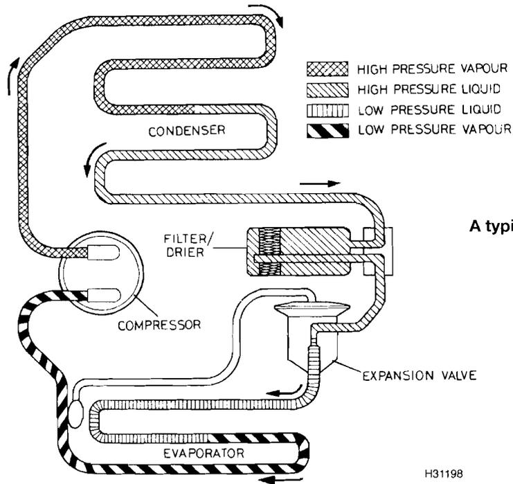
A typical expansion valve system
