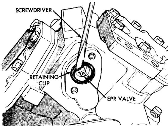
To replace the EPR valve, remove the retaining clip and pry out the valve (some valves can even be removed by simply grasping the center shaft of the valve and pulling it out - others may require a special extraction tool)
