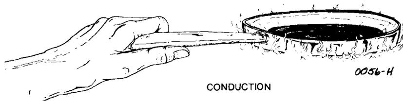
When you pick up a cast iron pan from the stove, the handle feels warm, even though it's not directly exposed to the flame, because the heat "conducts" through the metal pan to the handle - do the same thing with an aluminum pan, however, and you could burn your hand, because aluminum is a better conductor of heat than cast iron (in other words, the rate of heat transfer depends on the thermal conductivity of the substance)
