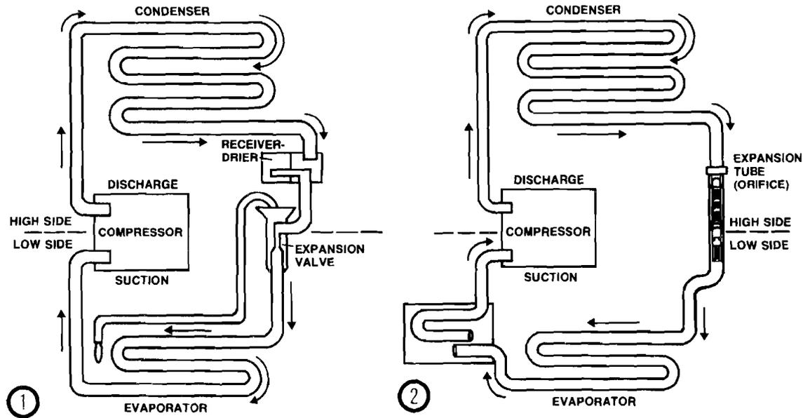
The compressor raises the pressure (and the temperature) so the refrigerant can condense and release heat as it moves through the condenser. A "pressure differential" is created at the expansion valve or orifice tube - the dividing point on the front side of the system. We will explain the expansion valve and orifice tube in detail later in this chapter.
