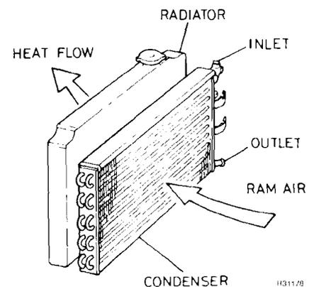
**The condenser looks and works just like a heater core, evaporator or radiator and is always installed right in front of the radiator to receive the full airflow from the vehicle's forward motion**
