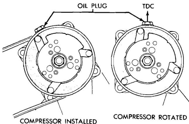
When you put the compressor on the workbench, make sure that the oil filler plug is at the top
