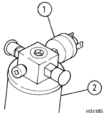
**Typical low pressure cut-out switch location (expansion valve system with receiver/drier)**
