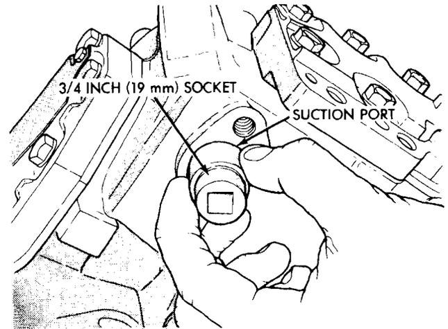
To install a new EPR valve, use a 3/4-inch or 19mm socket and carefully tap the valve into place
