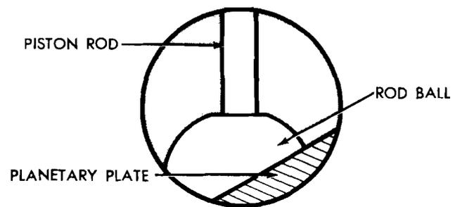
To verify that the hub plate lobe and index notch are aligned, look through the oil fill hole and verify that the ball end of the top piston rod lines up with the fill hole
