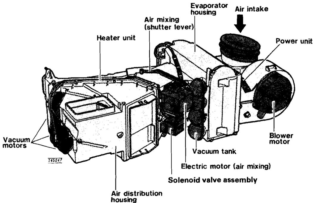
Typical under-dash heater/air conditioning housing assembly
