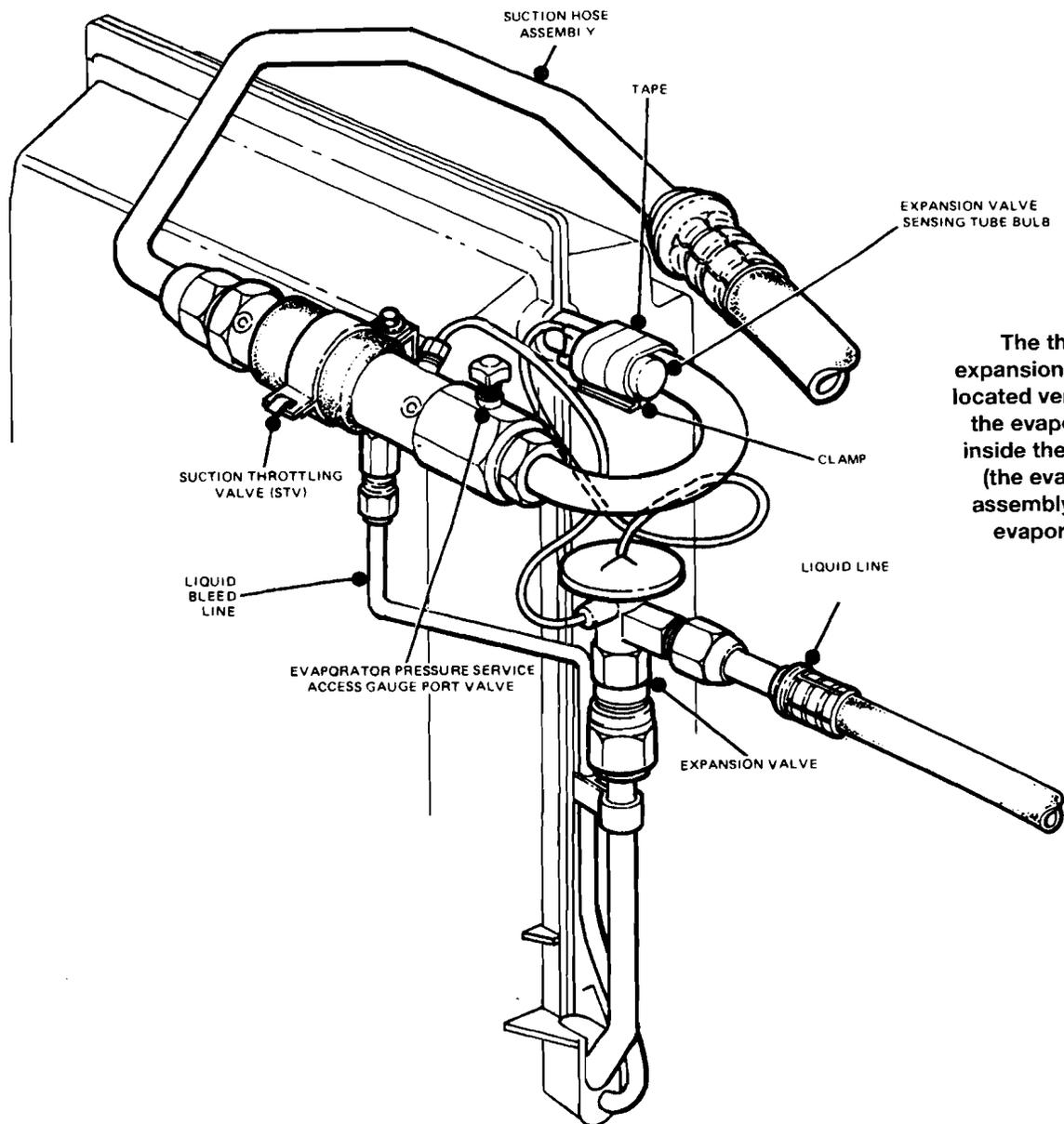
The thermostatic expansion valve is always located very, very close to the evaporator, usually inside the same housing (the evaporator case assembly) in which the evaporator resides
