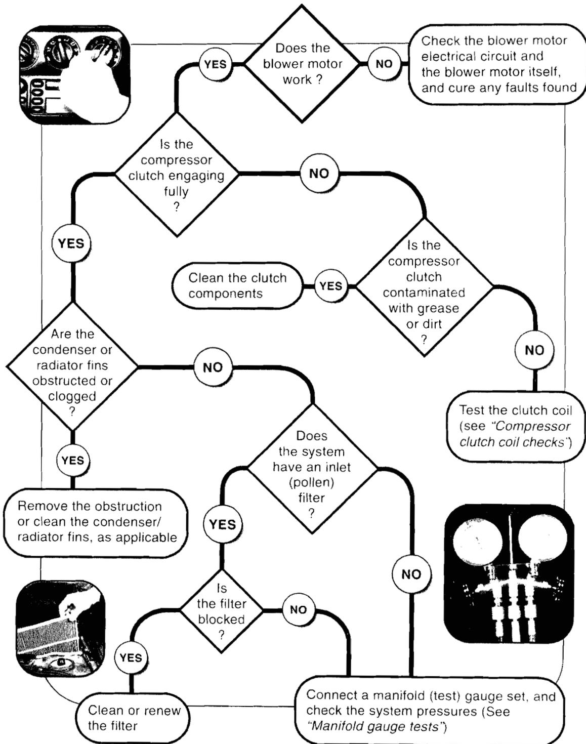
Chart 3: The cool air output is inadequate
