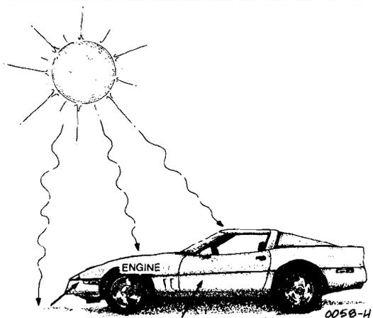
The sun, of course, isn't the only heat source - everything with heat radiates (because it's moving from warmer to cooler substances, remember?). Add up the heat radiating off your vehicle, its engine, the road, etc. and you can see why it gets hot inside the passenger compartment
