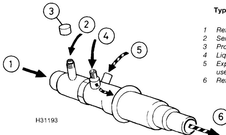
**Typical Pilot Operated Absolute Suction Throttling Valve (POA STV)**
