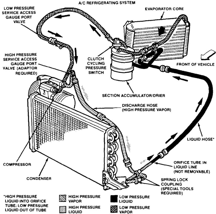
fice Tube (CCOT). Ford calls its system Ford Fixed Orifice Tube (FFOT).
