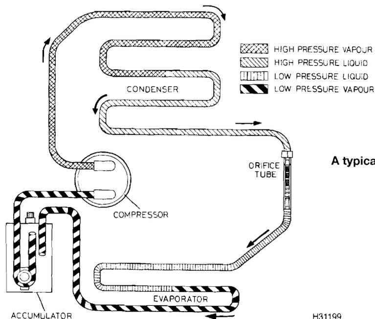
A typical orifice tube system
