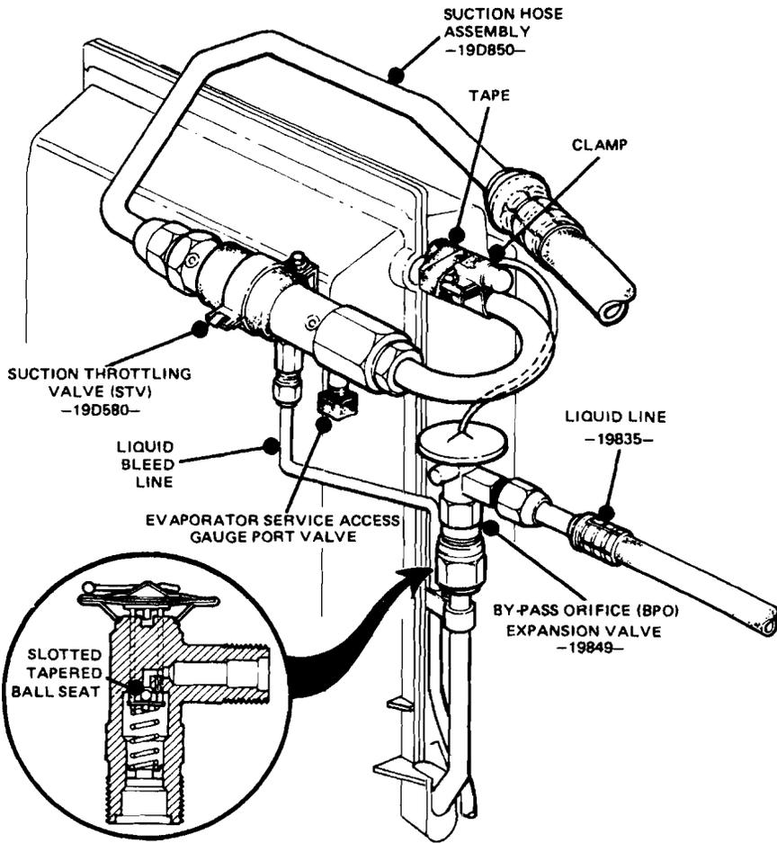
Ford Motor Company's By-pass Orifice (BPO) expansion valve uses a ball and slotted seat arrangement—the slotted seat keeps the valve from closing completely, allowing a small amount of refrigerant to flow into the evaporator, thus providing additional refrigerant and oil to the compressor for lubrication and cooling when the system is not operating at capacity - upper illustration shows location of principal components of assembly at evaporator, lower cutaway shows operation of the valve
