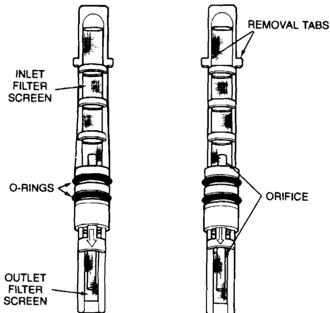
Cutaway of Ford Motor Company "fixed orifice" tube assembly - no matter what they're called or who uses them, all orifice tubes work the same way: they have filter screens to remove contaminants and a calibrated orifice tube to meter refrigerant flow
