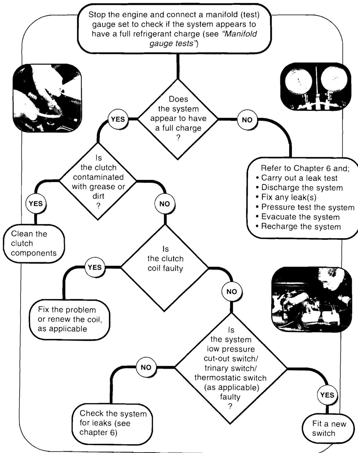
Chart 6: The compressor clutch does not engage
