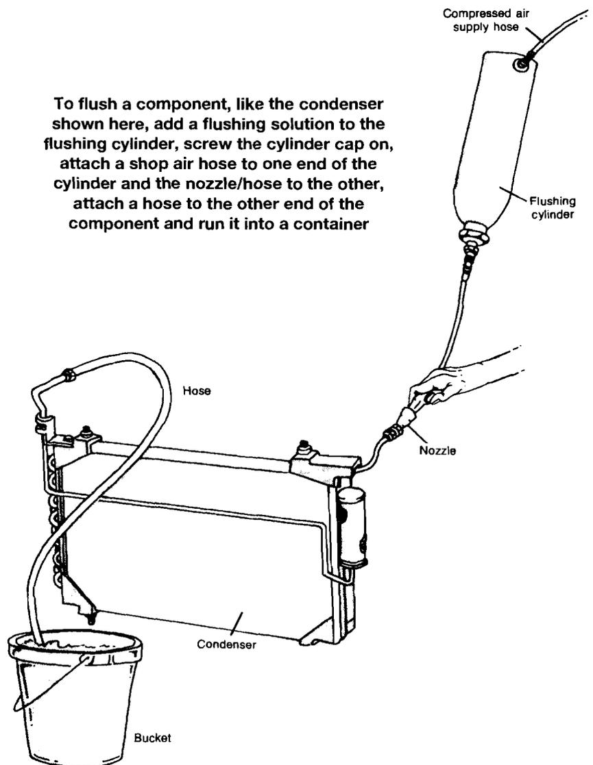
To flush a component, like the condenser shown here, add a flushing solution to the flushing cylinder, screw the cylinder cap on, attach a shop air hose to one end of the cylinder and the nozzle/hose to the other, attach a hose to the other end of the component and run it into a container
