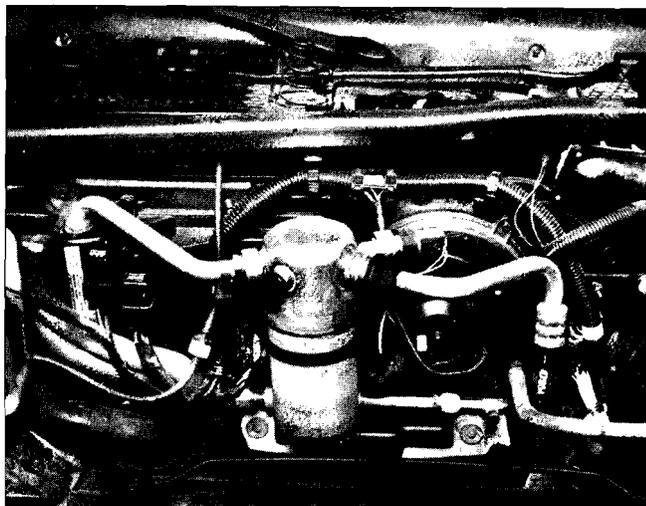
A typical accumulator assembly is not always this easy to see - this one's on a Pontiac Fiero, so it's not obscured by the engine - but, like all accumulators, it's mounted on the firewall right at the evaporator outlet pipe
