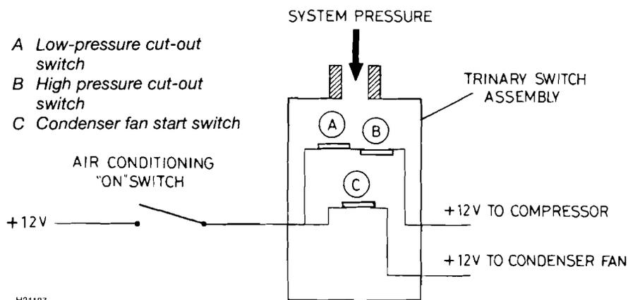
Schematic view of a typical trinary switch
