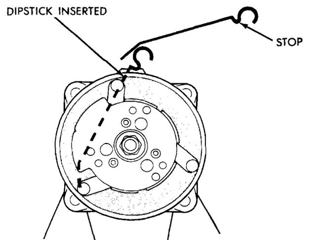
Insert the dipstick diagonally from the upper left to the lower left until the dipstick stop contacts the filler hole surface
