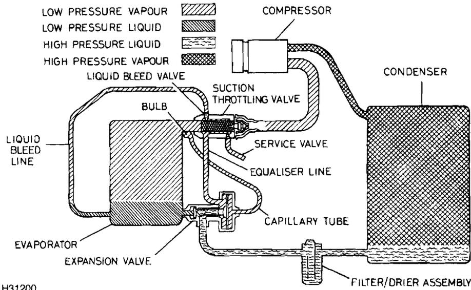
A typical Suction Throttling Valve (STV) system
