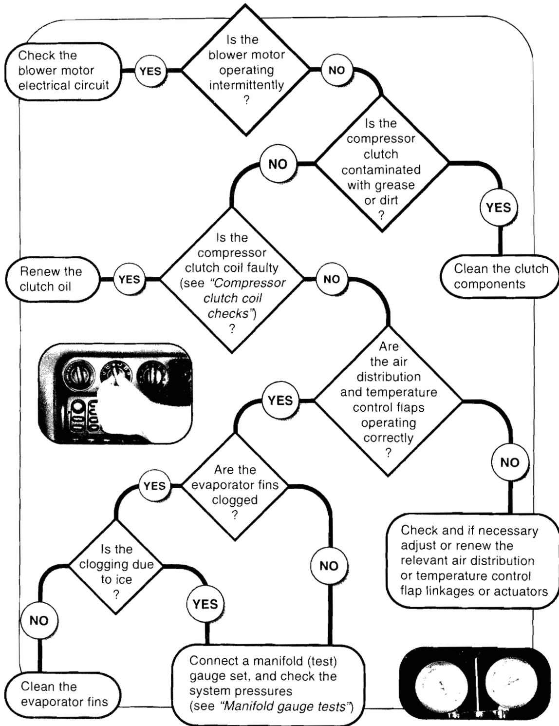
Chart 4: The system provides intermittent cooling airflow
