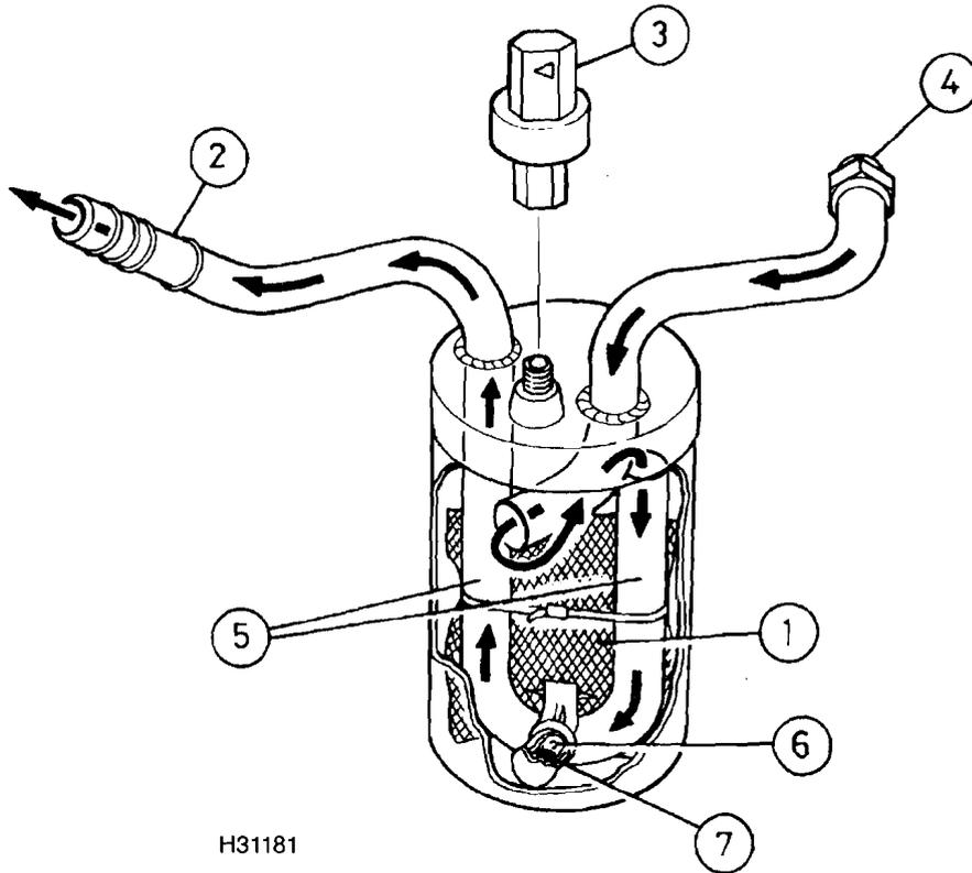
Cutaway view of a typical accumulator assembly
