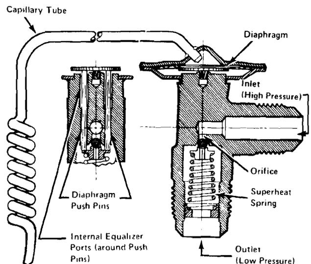
**Cutaways of another typical expansion valve (Volkswagen); note the similarity between this design and the Ford unit**
