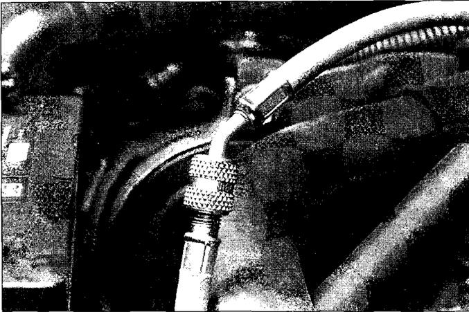
Note the angled metal line on this high side service hose - though not absolutely necessary, this design offers more flexibility when trying to attach it to hard to reach fittings
