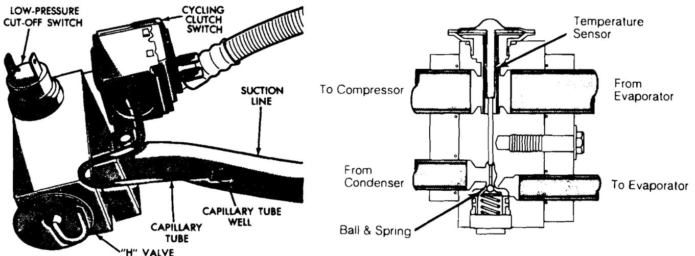
A typical Chrysler "H" valve (left); a cutaway of the same valve (right), which gets its name from the refrigerant passages which form the legs of the "H":
