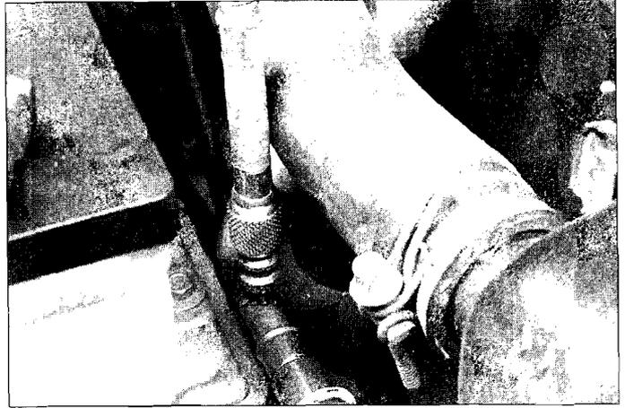
The high side fitting is usually in the high side line between the condenser and the evaporator - if it's difficult to get at, like this one, you may need to use a 6-inch flexible extension adapter to hook up the high side hose
