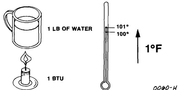
One British Thermal Unit (BTU) is equal to the amount of heat required to raise the temperature of one pound of water one degree Fahrenheit
