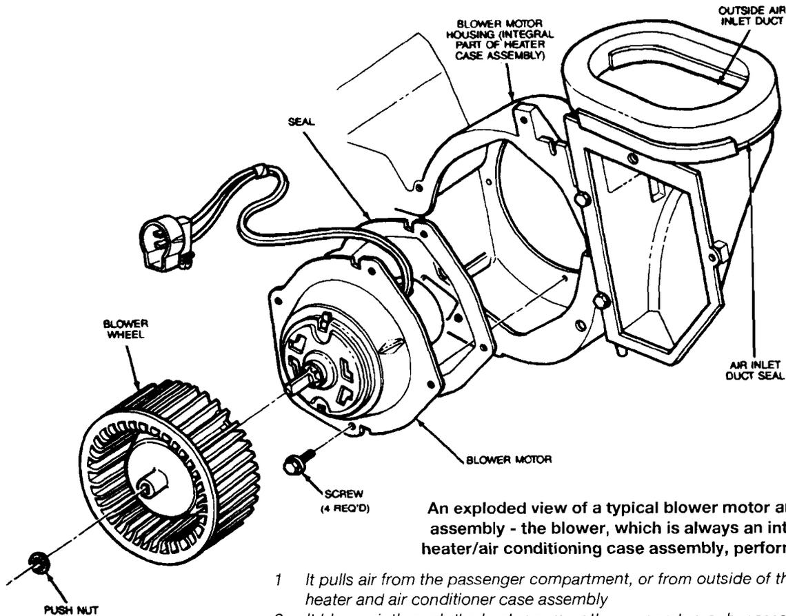
An exploded view of a typical blower motor and fan (or wheel) assembly - the blower, which is always an integral part of the heater/air conditioning case assembly, performs two functions:
