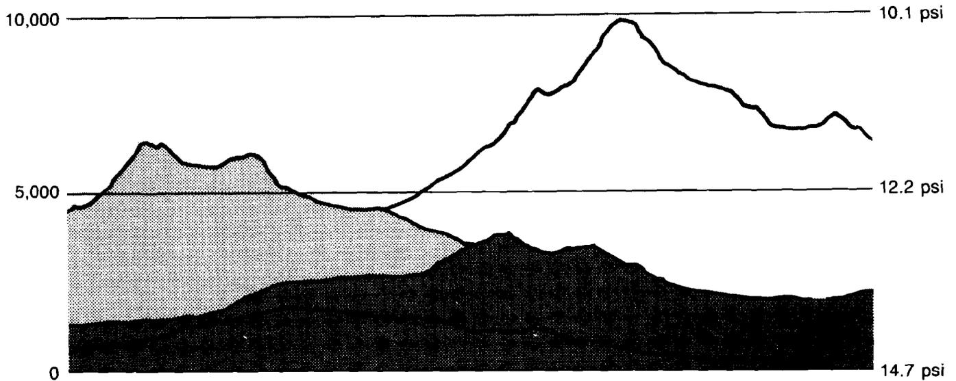
The higher the elevation, the lower the atmospheric pressure and the greater the necessary gauge correction)
