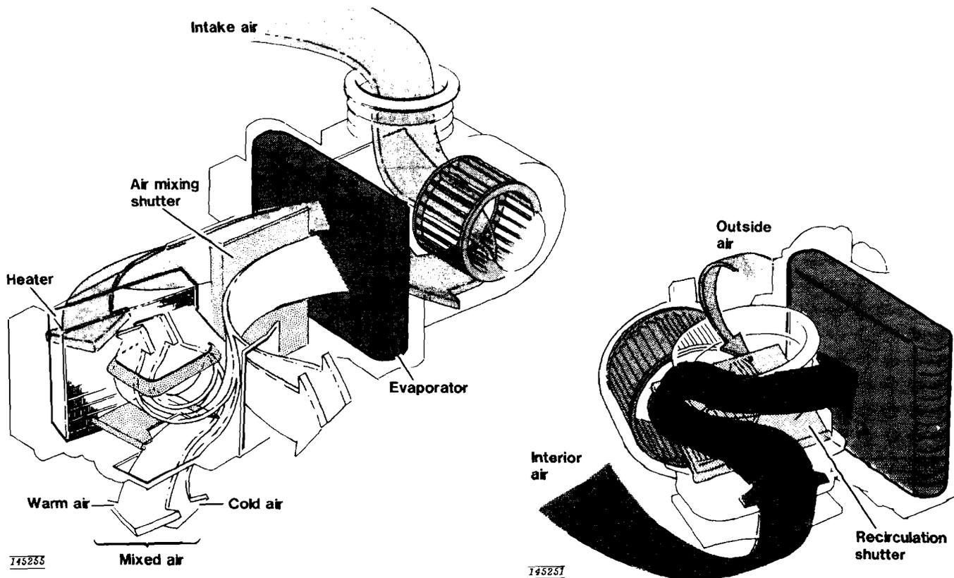
Heated, air-conditioned and/or outside air are mixed inside the under-dash ducting by opening and closing various doors
