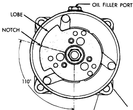
Rotate the hub plate lobe until the index notch is 110° from bottom dead center
