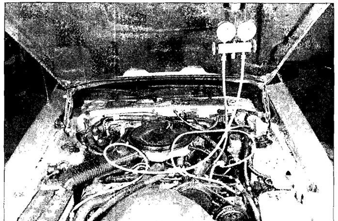
Once the manifold gauge set is hooked up, make sure both hoses are routed away from all moving and hot components
