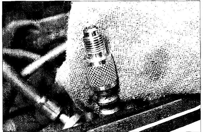
It's a good idea to protect the surrounding area of the engine compartment, and your eyes and skin, from refrigerant and oil with a shop rag when tightening or loosening a high side adapter fitting
