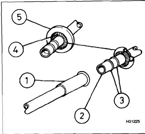
**Spring-lock refrigerant line coupling components**
