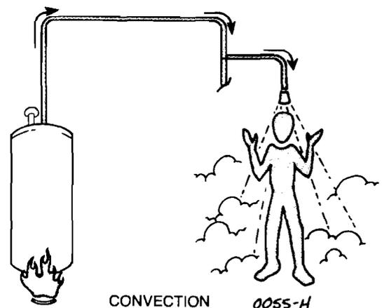
What happens when you turn on the hot water faucet in the shower? Hot water comes out the shower nozzle, even though the hot water heater is some distance away, because the water - or any liquid or gas, for that matter - has the ability to carry heat from one place to another - this phenomenon is known as convection
