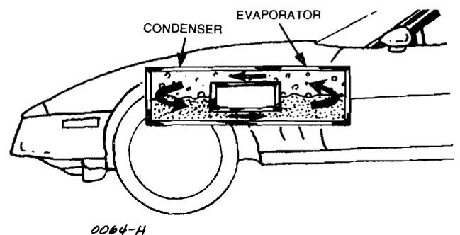
At the condenser, the R-12 is at a high temperature and pressure - higher, in fact, than the outside air around the condenser, so the heat in the R-12 flows away, through the condenser tubing and fins and into the outside air - by giving off heat, the R-12 condenses back to a liquid again and the cycle starts all over
