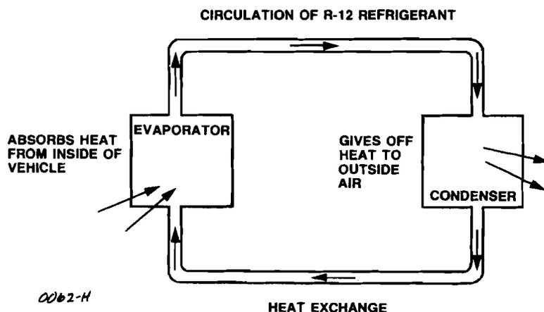
In its simplest terms, refrigerant absorbs heat from the passenger compartment at the evaporator, transfers it through a tube and sheds it to the outside air at the condenser
