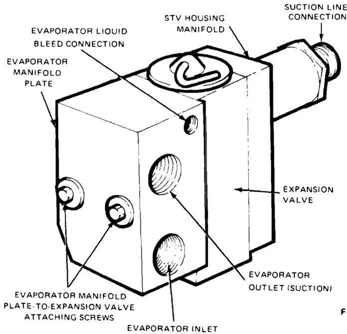
**Ford Motor Company's combination, or block, valve combines an expansion valve (similar in design to the Chrysler "H" valve) with the suction throttling valve for quicker valve response**
