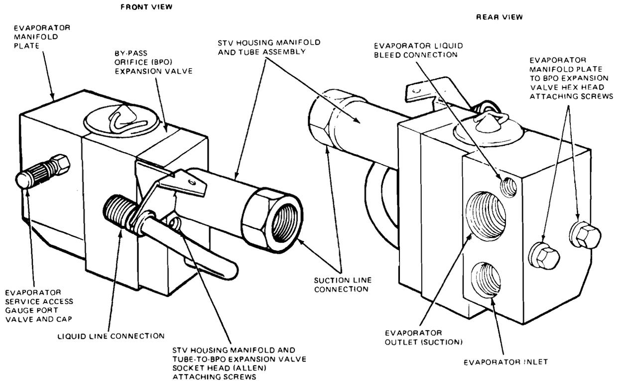
Ford Motor Company's By-pass Orifice (BPO) combination valve also uses the ball and slotted seat arrangement (upper illustration shows principal features of valve, lower cutaway shows operation of the valve)
