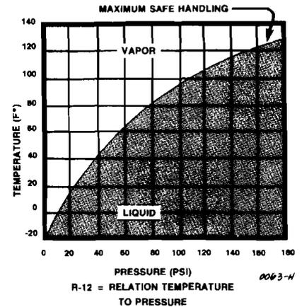
The most important characteristic of R-12, or refrigerant, is the relationship it maintains between pressure and temperature: If the pressure of R-12 is low, the temperature will also be low; if the pressure is high, the temperature will also be high - and, as the graph shows, within the 20 to 80 psi range, temperature and pressure vary directly
