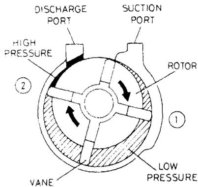
**Diagram of compressor operation**
