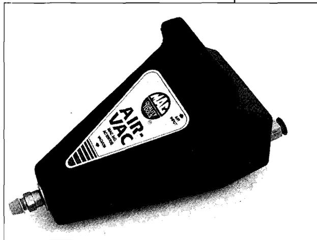
Venturi type vacuum pumps operate on compressed air (about 80 to 90 psi air power from a compressor) to pull down a vacuum in the system in about 1/2-hour - this type of pump is inexpensive to buy, but uses a lot of electricity (to run the compressor for 1/2-hour)
