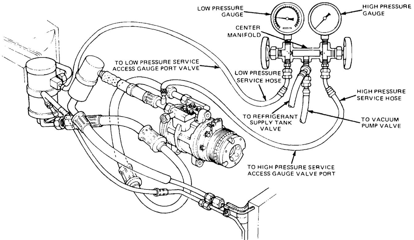
This is what the gauges look like when you start the vacuum pump: both gauges read zero - and the low side gauge will continue to drop below zero into the vacuum range as the pump sucks the system dry - the reading you're looking for is at least 25 in-Hg and even 30, if you can get it
