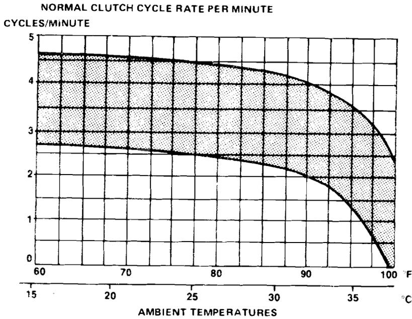
THESE CONDITIONAL REQUIREMENTS FOR THE FIXED ORIFICE TUBE CYCLING CLUTCH SYSTEM TESTS MUST BE SATISFIED TO OBTAIN ACCURATE PRESSURE READINGS
