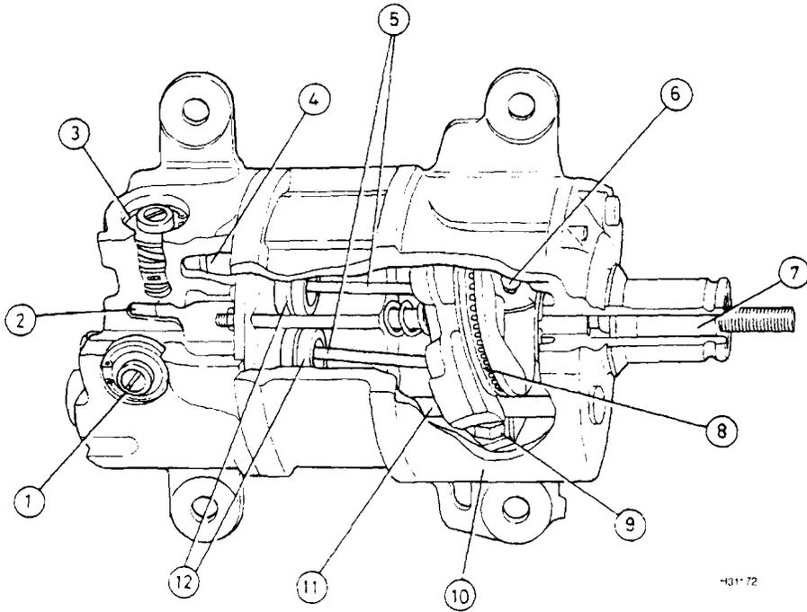
**Cutaway view of a typical variable displacement piston-type compressor**
