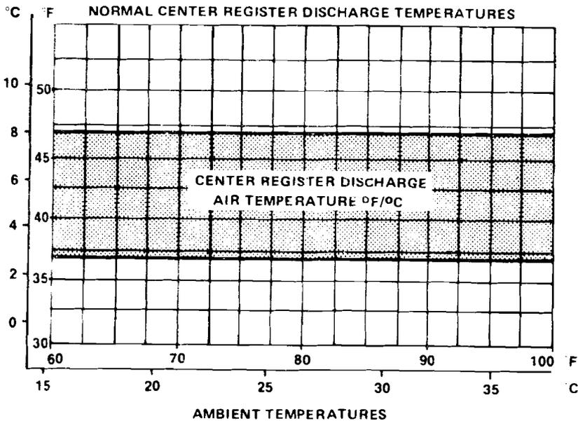
Refer to these charts to determine the normal clutch cycle rates and times and pressure/temperature relationships for Ford Fixed Orifice Tube (FFOT) system on F-100 through F-350 trucks and Broncos
