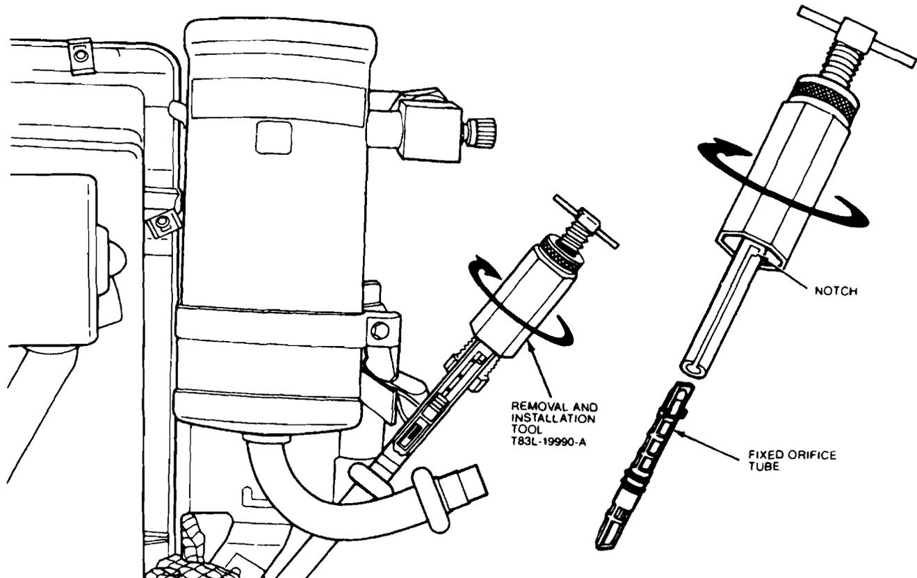
Insert the special tool into the tube, turn the tool clockwise to engage the tangs on the tube, then turn tool nut slowly to avoid breaking the orifice tube during removal
