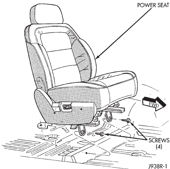
Fig. 4 Power Seat Remove/Install - Typical
