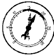
POOR VALVE SEATING AT IDLE
