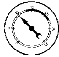
LATE VALVE TIMING, VACUUM LEAK AT IDLE
