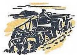
PLOWING. The Universal 'Jeep' operates pulltype and hydraulic-lift implements—has power andtraction for field work, with low speeds of 2½ to 7 mph.
