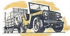
TOWING. The Universal 'Jeep' makes a highly efficient tow truck, capable of towing a braked payload of 5,500 lbs. with plenty of reserve for steep grades and heavy going.
