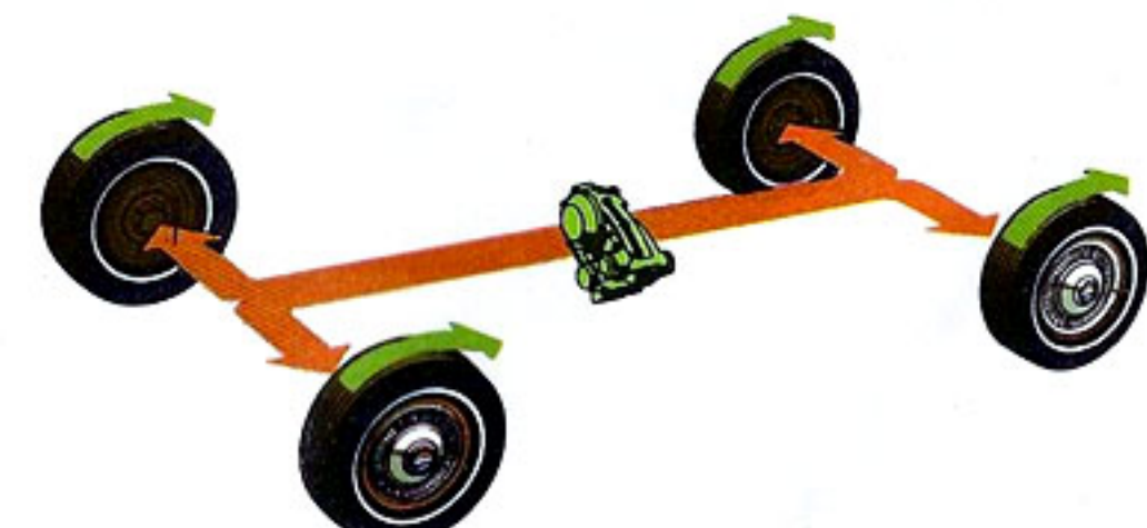
Traction is automatically distributed to all four wheels.
