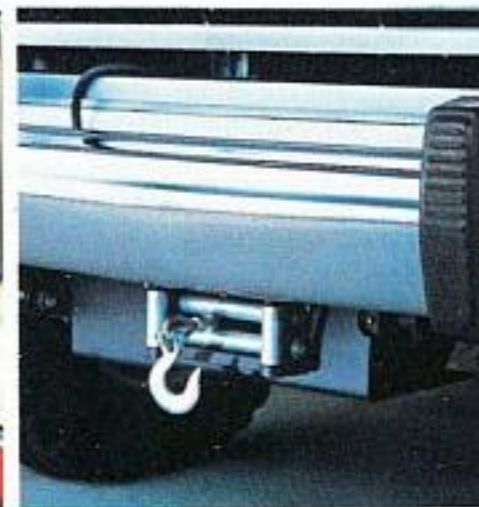
Hidden winch—dealer installed
