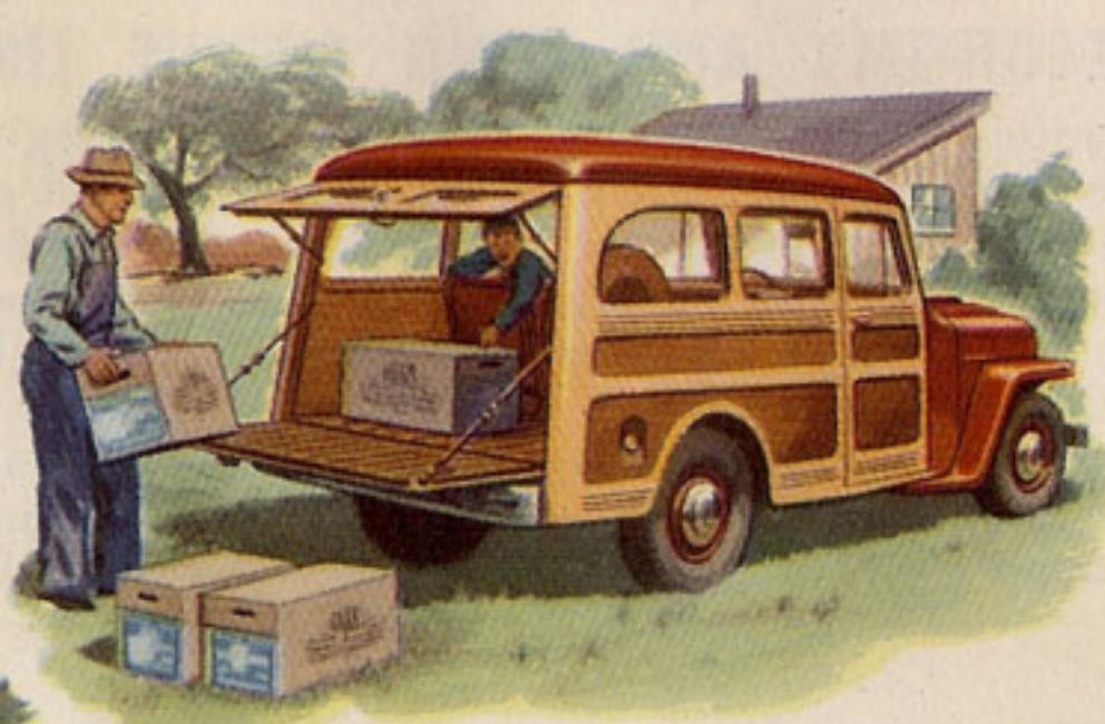
(Above) With seats removed, the "Jeep" Station Wagon has 98 cubic feet of usable cargo space, and even bulkier loads can be carried with the tailgate down. Steel floor, grained panels and seats are easy to wash.
