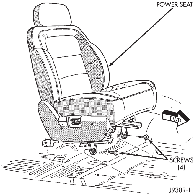
Fig. 2 Power Seat Removal—Right Side Shown
