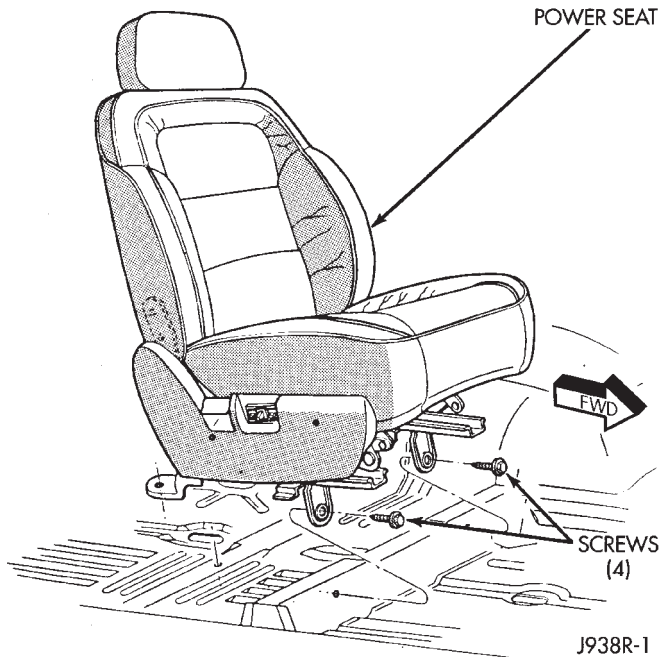
Fig. 2 Power Seat Removal—Right Side Shown
