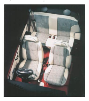
A new sports style steering wheel (derived from the MGF) not only looks and feels better, but brings the safety of airbag technology to the Mini for the first time. The new steering column incorporates the latest design of column stalks with both lights and wiper switching - intermittent wipe becomes a new Mini feature.
