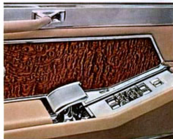
POWER CONTROLS: Provide remote adjustment of windows and ventilator panels. Consult your dealer about which controls are standard equipment on the particular model of your choice.
