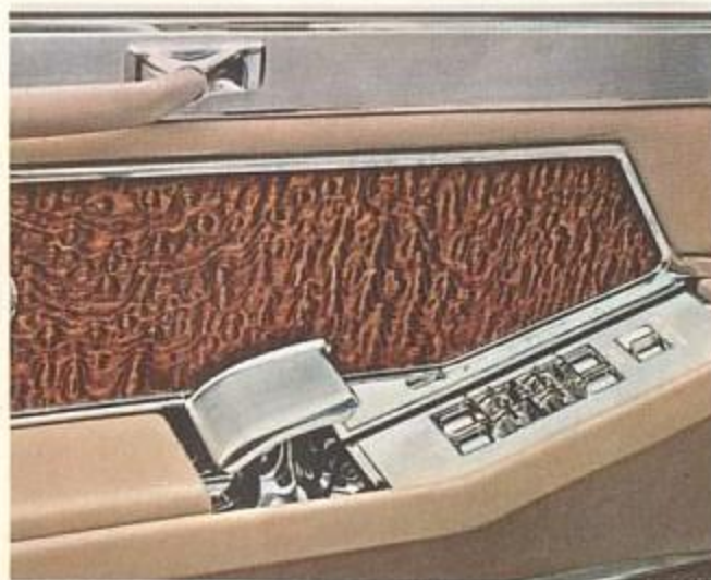
POWER CONTROLS: Provide remote adjustment of windows and ventilator panes. Consult your dealer about which controls are standard equipment on the particular model of your choice.
