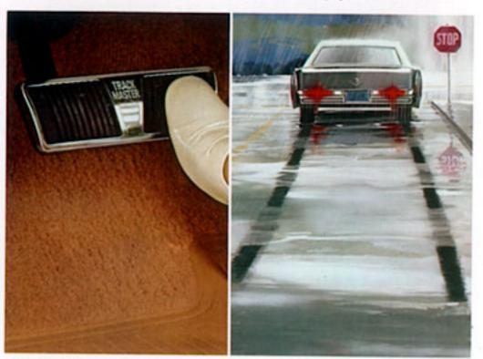
Track Master. This computerized skid-control system automatically pumps your brakes and maintains rear-wheel rotation for improved control during severe braking situations.
