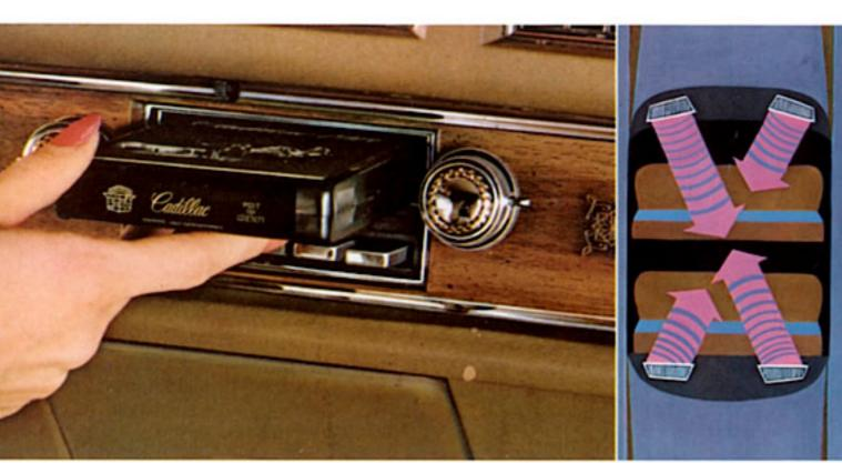
Stereo with Tape Deck. This AM/FM pushbutton stereo with integral 8-track tape player has set an exceptionally high standard of sound fidelity and styling for car radios. Its cross-fire design incorporates a total of four speakers, diagonally opposed within the passenger compartment, to give listeners a superb stereo effect. The speakers are positioned so that the windshield and rear window act as acoustic bandshells.
