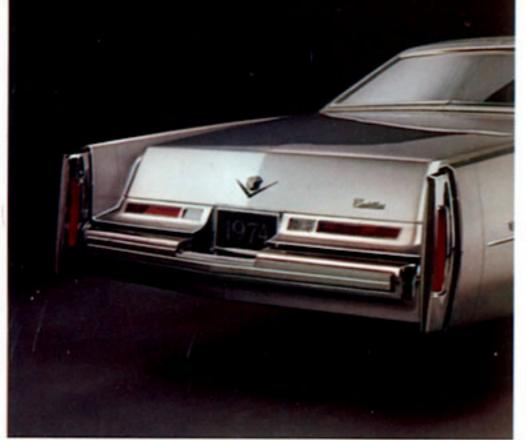
on-gray bumper impact strips and color-keyed flexible urethane filler material. The use of such material adds appreciably to the attractive exterior design of all 1974 Cadillac models-especially in the areas adjacent to bumpers.
