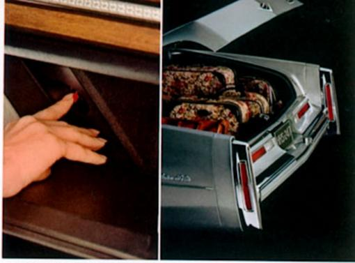
Automatic Trunk Lock Release. A control button inside the glove compartment releases the trunk lid. And when the lid is brought to a nearly closed position, the power trunk lock latches it securely again. There is also a warning light on the instrument panel to indicate when lid is unlocked.
