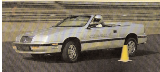
After it was fitted with an intercooled Turbo II engine and stiffer suspension, the LeBaron pace car was thoroughly tested to make sure it met or exceeded the exacting performance standards set by the Indianapolis Speedway.
