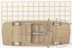
**E**sential to the Customer Satisfaction Audit, a finished LeBaron Convertible is fastened atop a leveled ramp in front of a machine that measures the exactness of the assembly plant's computerized front-end alignment procedures.
