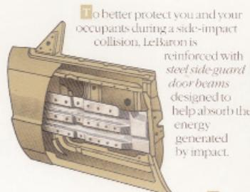
To better protect you and your occupants during a side-impact collision, LeBaron is reinforced with *steel sideguard door beams* designed to help absorb the energy generated by impact.
