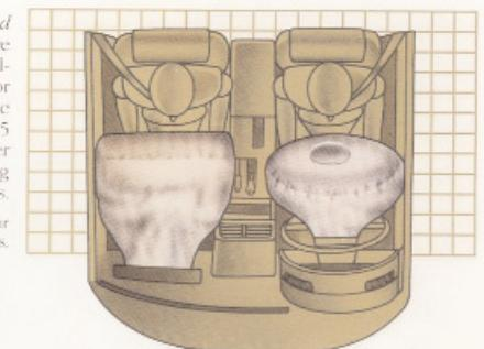
LeBaron's driver and front passenger air bags\* are deployed at a barrier frontal-impact speed of 14 mph or more. The driver-side bag deploys in 25 milliseconds; larger passenger-side bag in 35 milliseconds.
