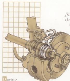
During hard braking, LeBaron's available *four-wheel disc antilock brake system* prevents lockup and allows you to maintain steering control for better maneuverability of the car. Special wheel speed sensors detect impending lockup, then the system's microprocessor selectively adjusts braking pressure up to 15 times per second.
