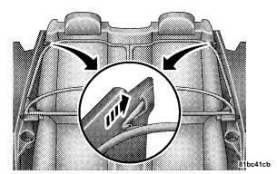
7. Align the pins at the front of the large frame with the hole in each trim panel. Slide the pins outward until fully extended into each hole.
