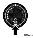
Press in on this button to engage the Air Conditioning. A light will illuminate when the Air Conditioning System is engaged. Rotating the dial left into the blue area of the scale indicates cooler temperatures while the rotating right into the red area indicates warmer temperatures.
