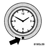
To set the analog clock, at the top center of the instrument panel, press and hold the button until the setting is correct. The clock will adjust slowly at first and then quicker the longer the button is held.
