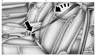
**Inserting Latch Plate Into Buckle**
