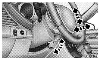
To unlock the steering column, push the control handle downward. To tilt the steering column, move the steering wheel upward or downward as desired. To lengthen or shorten the steering column, pull the steering wheel outward or push it inward as desired. To lock the steering column in position, pull the control handle upward until fully engaged.
