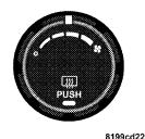
Rotate this control to regulate the amount of air forced through the ventilation system in any mode. The blower speed increases as you move the control to the right from the "O" (Off) position. There are four blower speeds.
