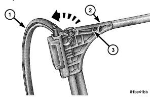
5. Unfold both stems at the rear of the large frame.
