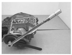
CAUTION: Never tighten the retaining nut with your impact gun. As tempting as it may be, the hammering could easily damage the roller bearing cages.
