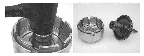
**Step 19:** Pull the input clutch retainer out of the OD/reverse piston. Remove the lip seal from the groove inside the OD piston. Remove the o-ring from the groove in the inside diameter of the piston.
