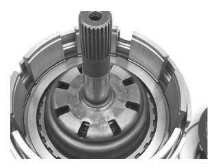
**Step 31:** Install the #3 thrust washer (5 locating tabs) on the underdrive shaft hub. Use assembly lube to hold the washer in place.
