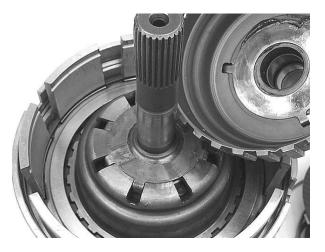
**Step 33:** Slide the overdrive shaft assembly over the underdrive shaft, and into the input drum assembly.
