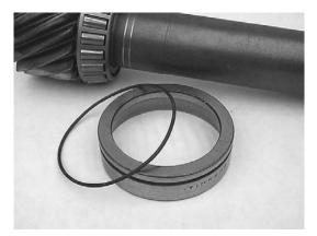
**Step 42:** Slide the lower bearing race and oil baffle into place on the transfer shaft. Coat the race and o-ring with assembly lube.
