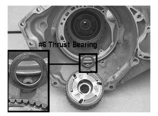
**Step 24:** Remove the rear sun gear and #7 thrust bearing (the bearing between the sun gear and the rear carrier) from the rear carrier.
