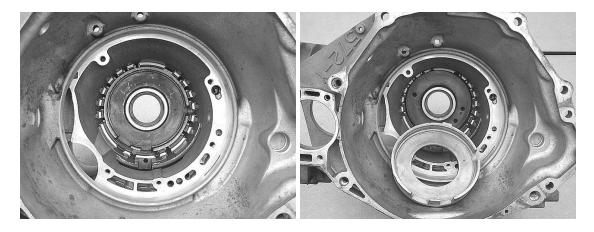
**Step 36:** Remove the three torx bolts from the low/reverse clutch piston retainer, and remove the retainer and gasket from the case. There may be a small aftermarket retainer support plate held on by two of the bolts. These support plates are an excellent update to the retainer, and should always be reused.
