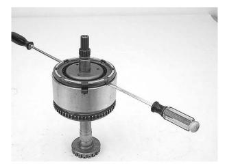
**Step 40:** Apply assembly lube to the #4 thrust plate and press it onto the OD clutch hub. This plate comes in several thicknesses and is the selective adjustment for input shaft end play.
