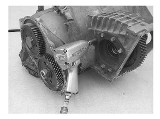
**Step 6:** Support the differential carrier while working the differential retainer loose, and remove the differential retainer from the case. Once you remove the differential retainer, the differential should roll right out of the housing.
