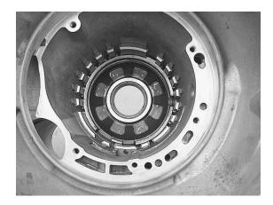
**Step 6:** Use an appropriate compressor to compress the spring — just far enough to clear the snap ring groove. Miller\* special tool #5058-3, #5059 and #6057 comprise the recommended compressor tools for this piston. Install the snap ring, making sure that the snap ring ends are both between two spring fingers, then remove the compressor.
