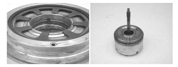
**Step 11:** Flip the assembly, and install the retaining snap ring onto the hub, with the tapered side of the snap ring facing up. Use a screwdriver and hammer to gently set the snap ring all the way into the groove. When seated, the gap between the ring ends is approx. 1/4".
