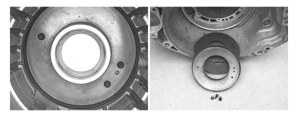
**Step 37:** Remove the low/reverse accumulator snap ring, and remove the accumulator cap from the case.
