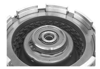
**Step 23:** Press down on the pressure plate to compress the waved lower snap ring and install the upper flat OD/reverse pressure plate snap ring. Work your way around the piston, pressing the snap ring into the groove as you go.
