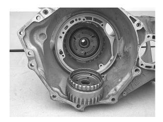
**Step 23:** Using the same rotating motion, remove the front planetary carrier assembly and #6 thrust bearing (the bearing between the carrier and the rear sun gear) from the case.
