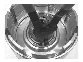
**Step 18:** Use a soft plastic or rubber mallet to tap the input shaft and hub assembly out of the input clutch retainer.
