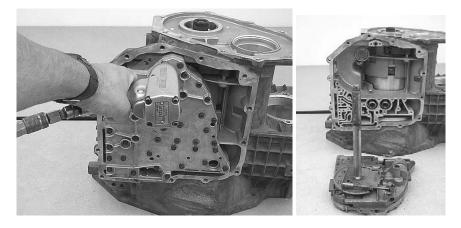
Step 16: Remove the overdrive and underdrive accumulator pistons and springs.
