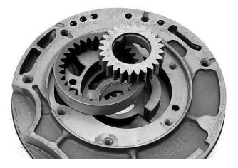
**Step 5.** Inspect pump gear and pocket surfaces for wear or damage, using the following measurements as guidelines:
