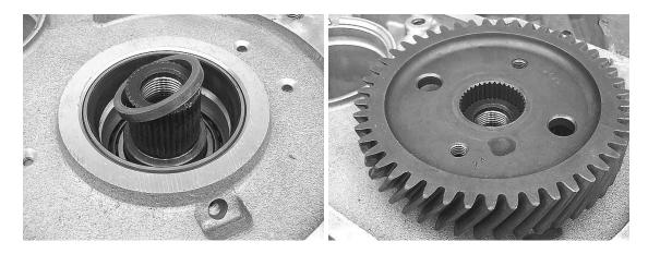
**Step 10:** Start the retaining bolt and cone shaped lockwasher by hand. When the bolt tightens, hold the gear with the holding tool, Miller\* special tool #6259, and torque the retaining bolt to 200 ft-lbs (270 Nm).
