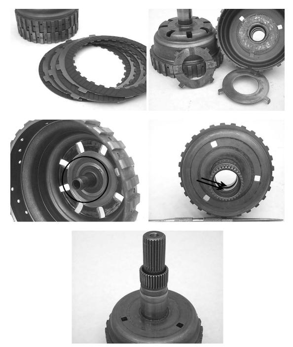
NOTE- The overdrive clutch hub has been known to break in the groove just below the splines. ATRA Technical Bulletin #321 covers an available kit which replaces the hub with an improved version and the other parts needed to make it fit.
