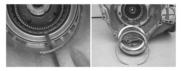
Step 26: Remove the 2-4 friction and steel plates from the case.
