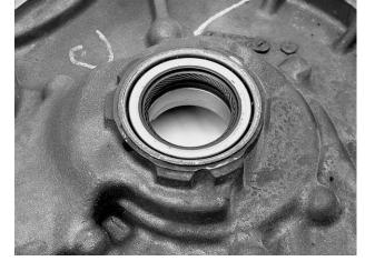
**Step 10.** Coat the pump pocket with assembly lube and place the pump gears into the pump body. Make sure that the side of the gears with the greater chamfer on the end of the teeth goes into the pump pocket first.
