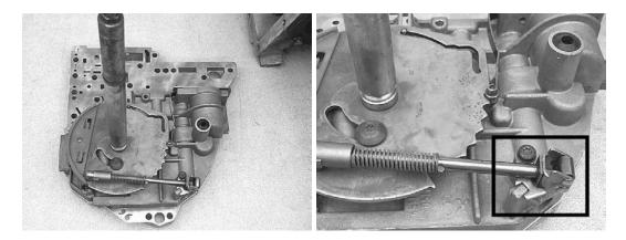
**Step 54:** Carefully work the valve body down into position. Install the valve body bolts by hand. Once all the bolts are in place, torque them down evenly to 40 in-lbs.
