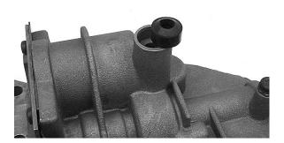
**Step 4:** Remove the 2-4 accumulator retainer bolts, and remove the plate and detent spring. Slide the accumulator and springs out of the valve body, and lay them aside.
