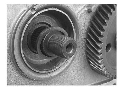
**Step 47:** Install the transfer shaft gear onto the transfer shaft. Install the lock washer and thread the retaining nut onto the transfer shaft.
