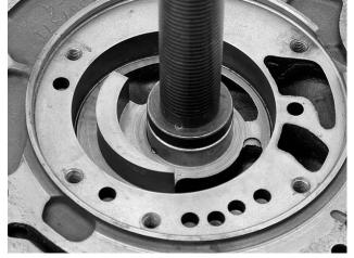
Step 7. Use a 1/8" punch to stake the bushing into the pump bore stake pockets.
