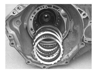
Step 27: Remove the low/reverse clutch reaction plate tapered snap ring.
