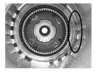
**CAUTION:** Be very careful not to scratch the top clutch surface of the reaction plate.
