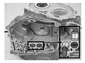
**Step 17:** Before removing the pump, check input shaft end play with a dial indicator. This end play should fall between .005" and .015" (0.12mm to 0.38mm). Excessive end play will give you a clue regarding internal wear, and if it checks to be within specification will allow you to save some time during reassembly. Once this check is complete, remove the pump retaining bolts.
