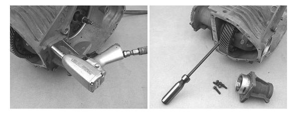
Step 5: Remove the differential retainer bolts.
