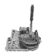
**Step 1:** Remove the retaining screw from the rooster comb, and lift the manual shaft off of the valve body.
