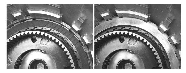
**Step 15**: Install the tapered snap ring in the case, with the tapered side facing up, and the opening toward the top of the case, installing both snap ring ends into the top case lug (the lug at the 12:00 case position).
