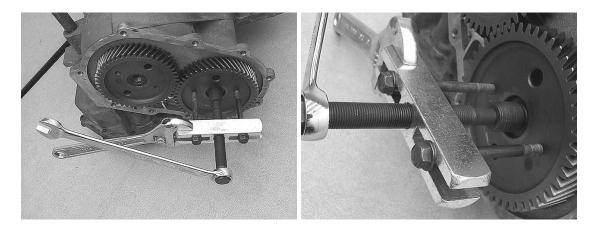
**NOTE:** It is advisable to mark the transfer gear and shim to avoid swapping them with the output gear and shim. Small marks from a grinding or cutting wheel will do nicely. Mark all 41TE units the same way and you'll always remember which is which, i.e., "Transfer gears and shims always have my grinder marks, output gears and shims don't".
