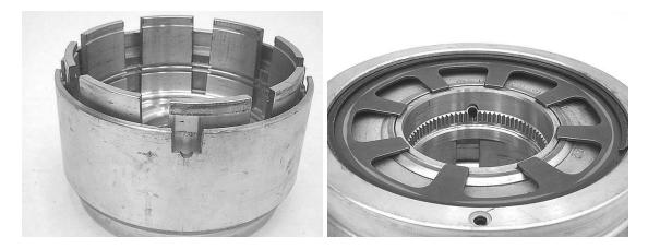
**Step 10:** Coat the inside diameter of the input drum assembly with assembly lube. Coat the lip seal surface on the outside of the OD/reverse piston. Set the input shaft and hub assembly into the input drum assembly, and press it into place. You may have to rotate the hub slightly to align the splines.
