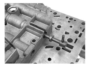
**Step 18:** Using a seal pick, replace the manual shaft seal. Slide the manual shaft onto the valve body — you'll have to hold the detent spring back while you're aligning the shaft. Make sure the manual valve pin lines up with the rooster comb. Install the retaining screw, and torque to 40 in/lbs.
