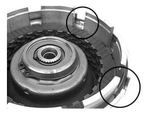
Step 22: Lay the overdrive pressure plate into the drum, Stepped side down.
