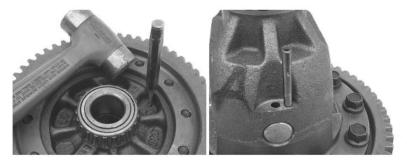
Step 3: Slide the pinion shaft out of the differential housing.
