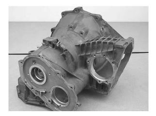
**Step 2:** Check for pulled or stripped threads in the case. Check for and remove any sizeable amounts of cured silicone from the bottom of bolt holes. Repair or replace as necessary.
