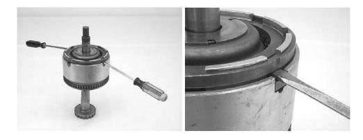
Step 4: Remove the reverse clutch disks from the input clutch assembly.
