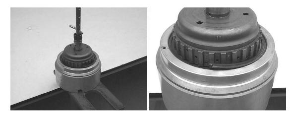
**Step 8:** Install the OD/reverse piston inner lip seal into the piston inner groove, then install the o-ring into the groove in the piston inside diameter. Coat them with assembly lube.
