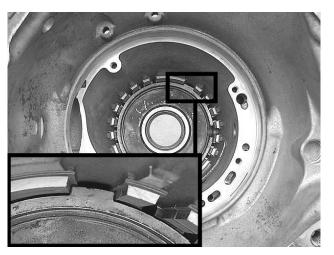
**Step 5:** Lay the low/reverse return spring into the case, inner finger ends facing up, outer edge of spring facing down.
