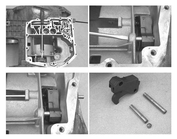
Removing the park pawl and **stamped steel** guide (guide has only one pin hole): Using a long thin screwdriver or punch, tap the park pawl guide pivot pin out, and remove the park pawl and guide bracket from the case. If it seems stuck, slowly rotate the rear planetary carrier while pulling on the bracket.
