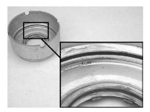
**Step 9:** Set the input clutch drum into the OD/reverse piston, and press the drum into place inside the piston. You'll know it's all the way in when the bottoms of both drums are flush with each other.
