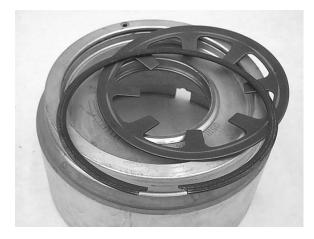
Step 22: Remove the lip seal from the groove inside the input drum.
