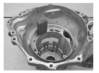
**Step 4:** Check for wear or damage in the accumulator bores. Replace as necessary. If bores are not damaged or excessively worn, condition bore sealing surfaces with a brake hone if necessary, then with ScotchBrite <sup>TM</sup> or equivalent material.
