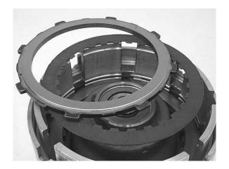
**Step 12:** Remove the flat snap ring from the underdrive clutch.
