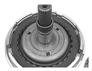
Step 38: Install the reverse clutch pressure plate, with the flat side facing down.
