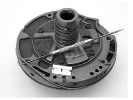
Step 2. Remove the seal rings from the stator support.
