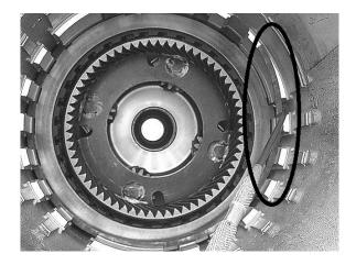
**Step 30:** The rear planetary carrier should be loose in the back of the case behind the low/reverse clutch pack. Gently pulling on the carrier, remove the carrier and the rest of the low/reverse friction and steel plates, which will come out of the case at the same time.
