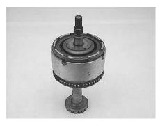
NOTE- The stand being used to support the drum is not a 41TE part. This is a 4T60 (440T4)  $4^{th}$  clutch shaft and hub.
