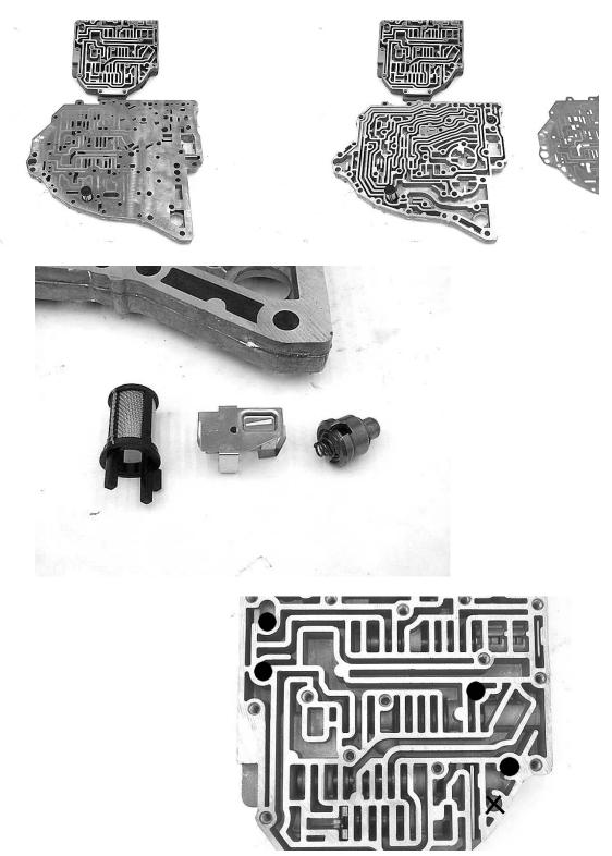
Step 7: Disassemble the valve body carefully. Set the valves, springs and retainers aside.
