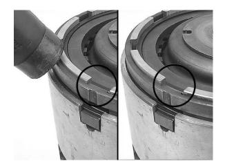
Step 2: Remove the reverse clutch snap ring.
