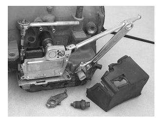
**Step 2:** Unbolt the transfer gear cover and differential cover and remove them from the case. Allow any oil to drain out of the unit.
