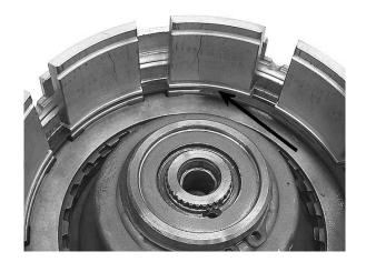
**Step 17:** Install the last thin friction plate in the underdrive stack, and then lay the reaction plate in place. Be sure the reaction plate is oriented correctly, because it can get confusing- If the plate has only one **Step**, this **Step** goes down. If it has two **Steps**, the **Step** at the lug goes down and the **Step** partway across the apply surface goes up.
