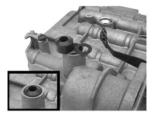
**Step 13:** Install new checkballs in the valve body, and reinstall the thermal valve, screen and spring-loaded orifice into the transfer plate. Lay the separator plate in place.
