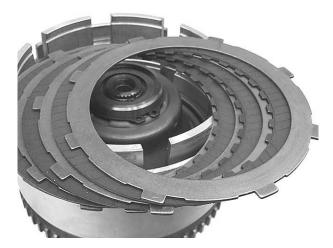
**Step 16:** Install the flat overdrive/underdrive reaction plate snap ring into place, making sure that both ends of the snap ring are inside one drum lug. Be careful not to scratch the clutch plate.
