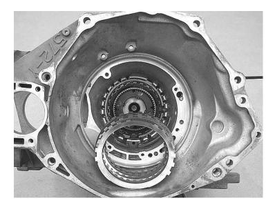
**Step 13:** Install the flat snap ring in the case, with the opening facing the top of the case. Be absolutely sure that the snap ring goes into the lower groove, and both ring ends inside one case lug, preferably the top (12:00) case lug. Be careful not to scratch the top surface of the clutch plate with the snap ring.
