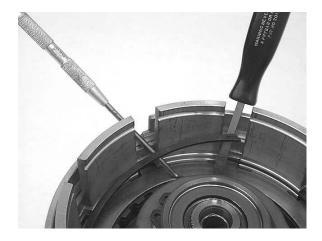
**Step 13:** Flip the drum over to remove the underdrive clutches from the input clutch assembly.
