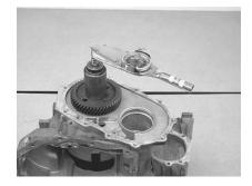
There should be between 3 and 8 inch/lbs of turning torque\*\*.
