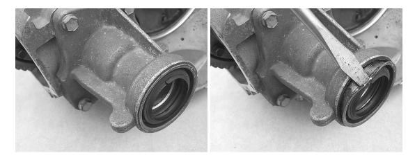
**Step 4:** Remove the extension housing bolts, then work the extension housing loose (try a prybar on the carrier inside the case), and remove it from the case.
