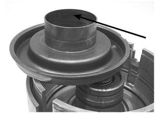
Step 17: Remove the input hub tapered snap ring from the input hub.
