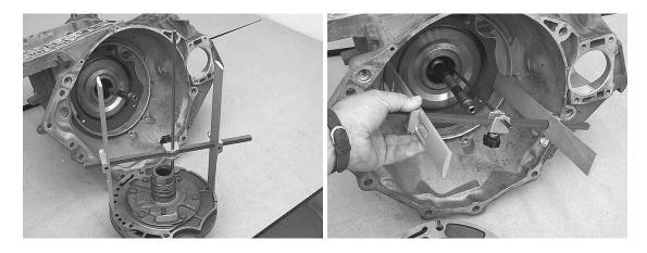
**Step 27:** To check input shaft end play, lay the pump gasket in place, using a dab or two of assembly lube to hold it in position.
