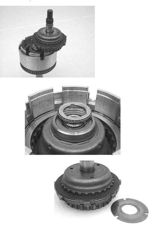
**Step 9:** Lift the OD clutch off of the OD clutch hub. Separate the two clutch hubs, and remove the #3 thrust washer and #3 thrust plate from between the two hubs. Check the shaft journal on the underside of the UD clutch hub for wear. There are two bushings inside the OD clutch hub that ride on the UD clutch hub bushing journals. These bushings do not fit the UD clutch hub shaft snuggly, and it is normal two feel some wobble between the two parts.
