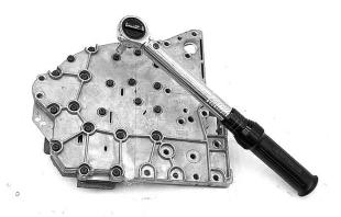
**Step 16:** Assemble the 2-4 accumulator and springs into the valve body, and set the detent and retainer in place. Bolt the retainer and detent onto the valve body, and torque to 40 in/lbs.
