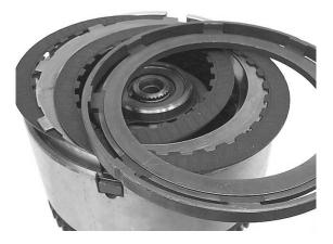
**Step 26:** Install the reverse selective snap ring in the clutch drum, and use two screwdrivers to raise the reverse pressure plate up against the snap ring.
