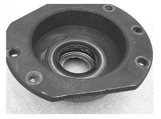
**Note-** If checking or adjustment of the differential preload will be necessary (due to changing the carrier, the carrier bearings, the case, or one of the extension housings, or differential noise or wear), you can prepare the differential bearing retainer for quick and easy testing and changing of the differential preload adjustment shim.
