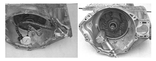
**Step 18:** Use slide hammers or an appropriate puller to remove the pump from the case. Remove and discard the pump gasket.
