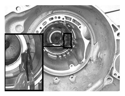
**Step 33:** Remove the low/reverse clutch return spring from the case.
