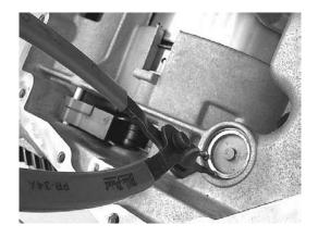
**Step 52:** Install the overdrive and underdrive accumulator pistons in the case, and then install the springs in the accumulators. Some later model units have different springs for these two accumulators. Make sure that the proper springs go into the proper pistons.
