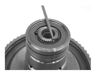
**Step 25:** Use a suitable press to press the input shaft out of the hub assembly, taking care not to let the shaft fall out and hit the ground.
