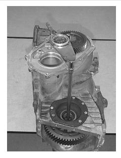
**IMPORTANT-** This measurement does not accurately indicate excessive preload. A shim that is substantially thicker than it should be will typically show turning torque within acceptable limits, possibly misleading you to believe that the current shim is acceptable when it may in fact be too thick. Always use the aforementioned end play test to establish shim thickness upper boundary.
