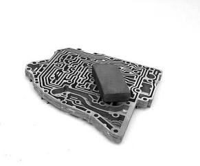
**Step 9:** Resurface the 2-4 accumulator bore. A brake hone is good for this, but be sure not to remove too much material from the bore, just enough to clean up the surface. Smooth the texture a bit with some Scotch-Brite  $^{TM}$ .
