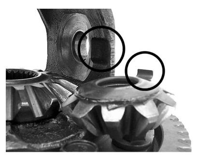
Rotate the side gears to spin the pinions into place. Make sure the pinion gears align with the shaft openings in the differential. If not, rotate the pinion gears back out, and adjust their position relative to the side gears.
