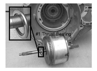
**Step 21:** Remove the input clutch assembly from the case. The #4 thrust washer, which is normally installed on the front sun gear hub, may come off with the clutch assembly. Be sure that this washer is located and set with the other small parts before continuing further.
