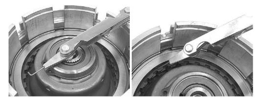
**Step 20:** Install the overdrive clutch stack in the clutch drum, which includes four thin frictions and three thin steels. If your unit only takes three thick frictions and two thick steels, it must be updated to the new style drum that accepts four frictions. See the note at the beginning of this section.
