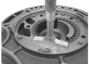
Clearance between the top of the inner pump gear and the top of the pump pocket should be less than 0.002".
