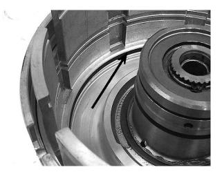
**Step 13:** Coat the inside and outside diameters of the underdrive piston with assembly lube. Lay the underdrive clutch piston into the drum, and rotate it into place.
