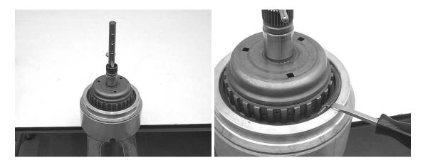
Step 21: Remove the snap ring and return spring from the piston.
