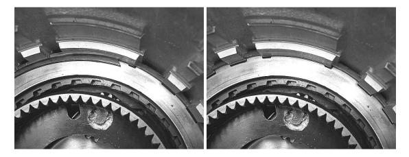
**CAUTION:** Be very careful not to scratch the top clutch surface of the reaction plate with the snap ring or ring installation tools.
