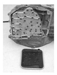
**Step 15:** Rotate the shift lever all the way **clockwise** when viewed from the outside end of the shaft. This will be one click *past* manual low, which is inaccessible when the vehicle shifter is connected to the lever. This locks the Park rod onto a bracket on the valve body, making it much easier to remove and install the valve body. Remove the valve body bolts, and carefully lift the valve body out of the case.
