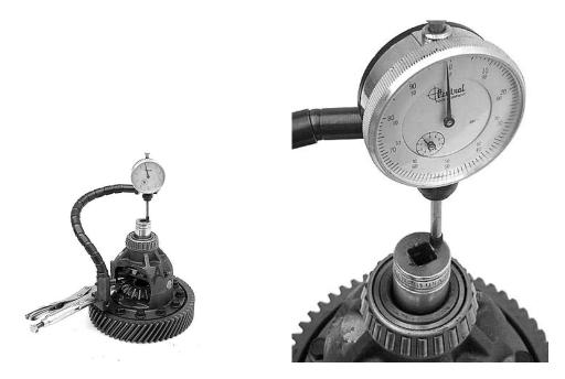
Side gear endplay should be between 0.001" and 0.013" (0.02 mm to 0.35 mm). Replace the selective side gear thrust washers to adjust the endplay.
