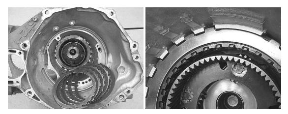
**Step 17:** Install the 2-4 return spring in the case, outside edge facing down against the last steel plate, inner edge fingers pointing up. Check the 2-4 clutch pack clearance by using either the 'feel' method, or mounting a dial indicator to the case and zeroing it on the top 2-4 steel plate or clutch tooth. While holding the return spring down against the case lugs with a hammer handle or something similar, pull up on the top 2-4 clutch and record the travel.
