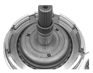
**Step 36:** Press down on the OD/reverse pressure plate and install the flat snap ring into the OD/reverse piston to secure it.
