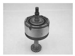
**NOTE-** The stand used to support the input drum in this section is not a 41TE component. It is a 4<sup>th</sup> clutch hub and shaft from a 4T60 (440T4).
