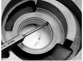
**Step 8.** Check the bushing to converter hub clearance with a feeler gauge. The clearance between the pump bushing and the converter hub should be less than 0.005". If there's too much clearance, look for wear on the converter hub.
