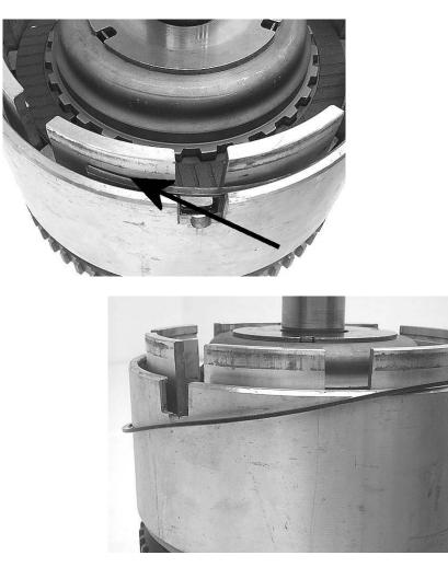
**Step 8:** Holding the solid underdrive clutch hub shaft, lift out both clutch hubs and the overdrive clutch pack. Be careful not to lose the #2 thrust bearing, which may either be on the input drum or the underside of the underdrive clutch hub. Remove the selective #4 thrust plate from the top of the OD clutch hub.
