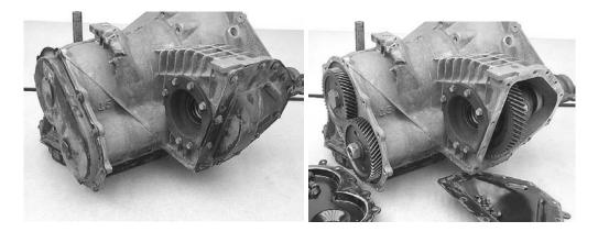
**NOTE:** This unit is prone to tip to the side while the differential assembly is in the case. Therefore, disassembly will be easier with the differential removed before disassembling any other area.
