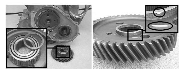
**Step 10:** Using a suitable prying tool, remove the transfer gear upper bearing race retainer.
