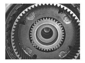
**Step 22:** Grease the #6 thrust bearing into place on the back of the front planetary carrier, then install the front planetary carrier into the case. You'll have to wiggle the planet to line up the clutches and gears.
