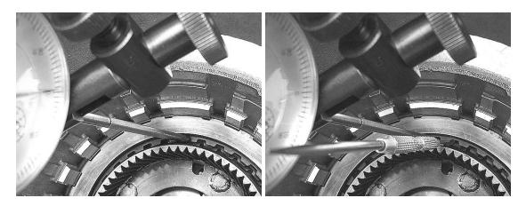
If the travel shown is out of the above range, you can adjust this clearance by changing the selective low/reverse-2/4 clutch pressure plate. The available pressure plate sizes are:
