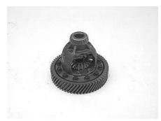
**Step 1:** Check the bearings and races for wear or damage, and replace as necessary. Always replace the bearing and race as an assembly.
