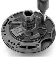
Step 4. Remove the pump gears from the pump body pocket.
