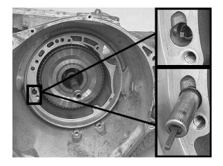
**Step 20:** Locate and remove the #1 thrust bearing, which is either inside the input drum seal ring bore, or stuck to the rear end of the stator support.
