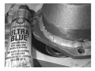
**Step 38:** Install the differential assembly into the case, and hold it in place. Install the differential bearing retainer, and thread the retaining bolts in by hand.
