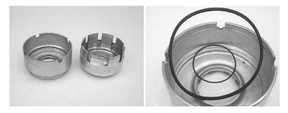
IMPORTANT- there is a small screened orifice pressed into the bottom ridge of the piston which has been known to blow out either in use or during service such as this. The unit will not work if this orifice is missing. Be certain that the orifice is in place. If not, replace the piston.
