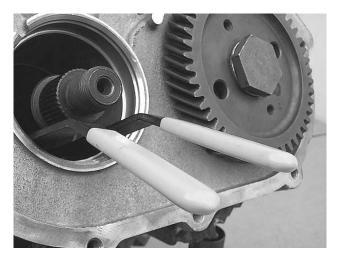
**Step 45:** Install the upper transfer bearing retainer into the case, with the tab on the retainer aligned with the slot in the case.
