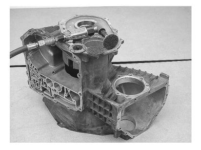
**WARNING-** Using this type of tool on valve body and pump mating surfaces almost guarantees a major failure of your work due to leaks caused by uneven surfaces. Keep powered abrasive tools away from this type of critical surface.
