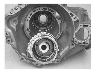
**Step 31:** Use an appropriate spring compressor to compress the low/reverse clutch return spring.
