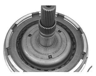
**Step 39:** Install the reverse clutch snap ring in the input drum, then pry up on the pressure plate to seat it against the snap ring.
