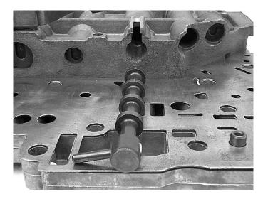
Step 3: Remove the 2-4 tower seal from the valve body.
