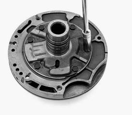
Step 12. Torque the pump bolts to 23 ft/lbs.
