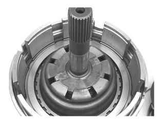
**Step 32:** Install the #3 thrust plate (3 locating tabs) onto the overdrive shaft assembly. Use assembly lube to hold the plate in place.
