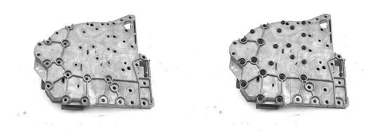
Step 15: Torque the valve body bolts to 40 in/lbs.
