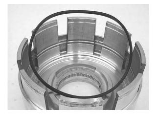
Step 23: Remove two lip seals and two o-rings from the input hub.
