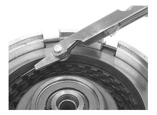
**Step 25:** Set the reverse clutch pack in the drum, and install the reverse pressure plate with the flat side facing down. Gently tap it down as far as it will go.
