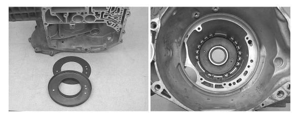
**Step 3:** Set the aftermarket retainer stiffener in place, which avoids leaks in the piston housing-to-case interface, and start the screws by hand. Torque the screws to 40 in-lbs..
