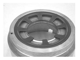
**Step 7:** Use a suitable press to compress the overdrive return spring. The OD clutch hub makes a great press adapter. Install the snap ring, and release the spring.
