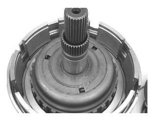
Step 34: Install the overdrive clutches into the input clutch drum.
