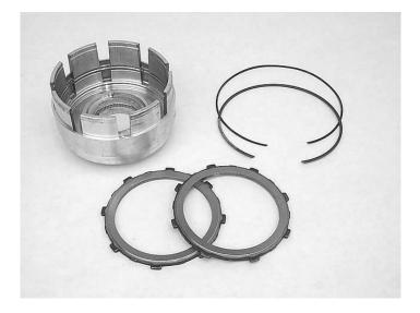
**Step 1:**Clean all of the input clutch assembly components, and inspect them for wear or damage. Pay particular attention to:
