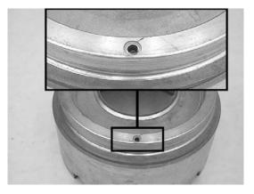
**Step 20:** Use an arbor or foot press to compress the OD/reverse return spring. The OD clutch hub makes an excellent press adapter for this purpose. Be careful: Just compress the spring enough to remove the retaining snap ring.
