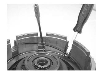
**Step 11:** Remove the overdrive/underdrive reaction plate, and the first underdrive clutch plate.
