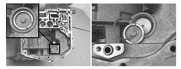
**Step 38:** Remove the low/reverse accumulator piston and spring from the case. If the piston appears stuck in the case bore, locate the bore vent hole inside the case in the low/reverse clutch case lugs. Cover the accumulator bore with a rag and send a blast of air pressure into the vent hole to blow the piston into the rag.
