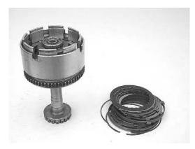
**Step 29:** Install the #2 thrust bearing on the input hub. Use assembly lube to hold the bearing in place.
