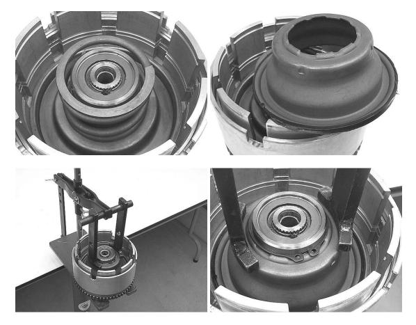
**Step 15:** Install the underdrive clutch stack in the clutch drum; leave out the top friction plate for now. This will include four thin steel plates and three thin friction plates.
