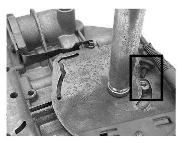
Step 2: Slide the manual valve out of the valve body.
