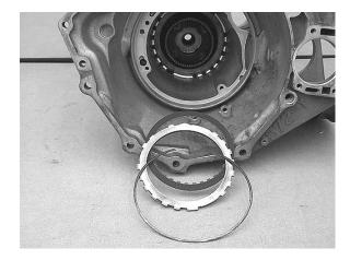
Step 29: Remove the low/reverse clutch reaction plate flat snap ring.
