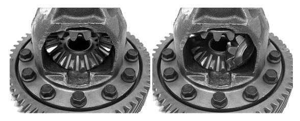
Step 5: Remove the side gears from the housing.
