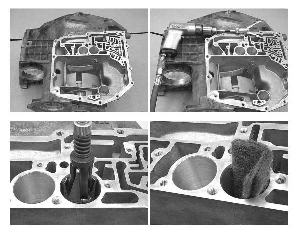
**Step 5:** Check for worn or damaged splines in the case. Slight notching (less than 1/16" deep) of the case lugs from steel plate motion is acceptable. Replace case if necessary.
