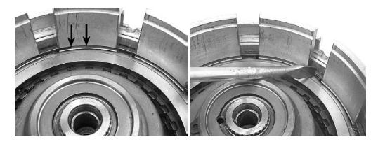
**Step 19:** Use a wire or spark plug gauge between the top friction plate and pressure plate to check the clutch clearance. Clearance should be between 0.035" and 0.060" (0.90 mm and 1.50 mm); for best results, keep the clutch clearance on the loose side. To adjust the clearance, replace the selective pressure plate. The drum kit described at the beginning of this section includes the two plates you may need.
