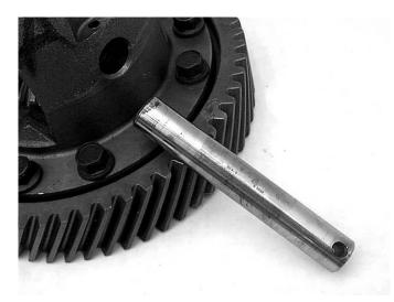
**Step 4:** Rotate the side gears to align the pinion gears with the openings in the housing, and remove the pinion gears.
