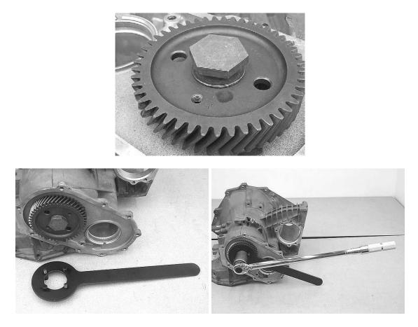
**CAUTION:** Never tighten the retaining bolt with your impact gun. As tempting as it may be, the hammering could easily damage the roller bearing races and cages.
