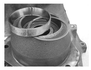
**Step 31:** Set the differential carrier into position in the case. Using no sealer, install the differential bearing retainer and the extension housing. Torque the retainer and housing bolts to 21 ft-lbs.
