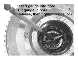
Swing gauge inside bore to compress probes to bore diameter.
