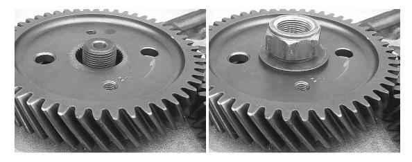
**Step 48:** Using the proper holding fixture for the transfer gear (use Miller\* special tool #6259), torque the transfer shaft gear retaining nut to 200 foot-pounds (270 Nm).
