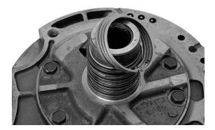
**Step 3.** Remove the body-to-support bolts being careful to support the pump body as you remove the last bolt.
