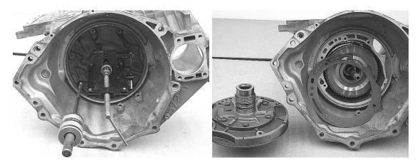
Step 19: Remove the cooler bypass valve, if so equipped.
