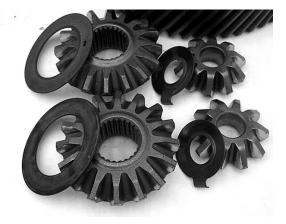
Step 6: Check the gears, pinion shaft and thrust washers for wear or damage.
