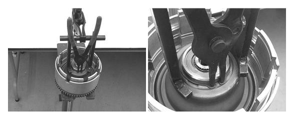
**Step 15:** Release the underdrive clutch return spring, and remove the return spring retainer and return spring from the input clutch assembly.
