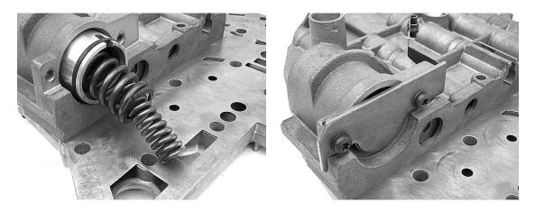
Step 17: Slide the manual valve into the valve body bore.
