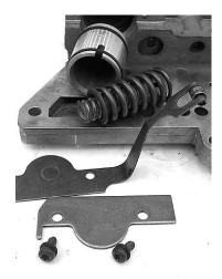
**Step 5:** Invert the valve body, and remove the valve body bolts. Hold the separator plate to the valve body transfer plate, and lift them off of the valve body as an assembly.
