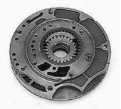
The 41TE uses a very straightforward, conventional crescent pump. There are no valve assemblies or intricate parts, other than screened checkball-controlled orifices in the stator support which are completely inaccessible.
