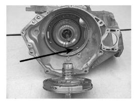
**Step 28:** Coat the stator support rear bore and the pump seal rings and lands with assembly lube. With no pump o-ring in the pump body groove, slide the pump into the case. Gently tap it all the way in, and start three of the pump bolts by hand, as shown in the above picture. Tighten these pump bolts with a speed handle or one hand on a ratchet wrench until good and snug.
