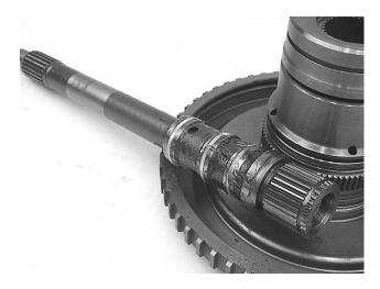
Step 3: Use a suitable press to press the input shaft into the input shaft hub.
