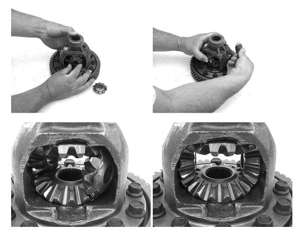
Step 9: Slide the pinion shaft into place.
