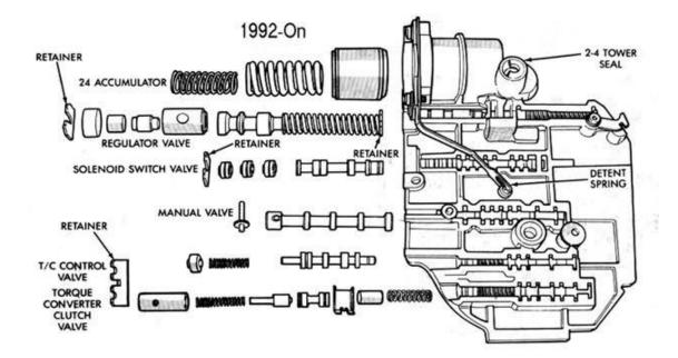
**Step 8:** Clean all components thoroughly. Check for signs of wear or damage, particularly at the pressure regulator valve and bore. Since cross-leaks are a real problem on this unit, flat-sand all machined valve body surfaces.
