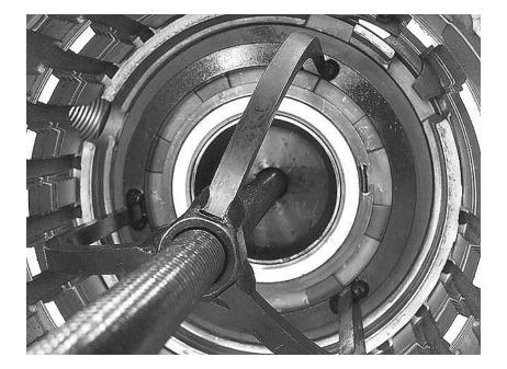
**Step 32:** Remove the return spring retaining snap ring, then release the compressor from the low/reverse clutch return spring.
