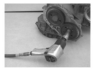
Step 8: Remove the output gear bolt from the output shaft.
