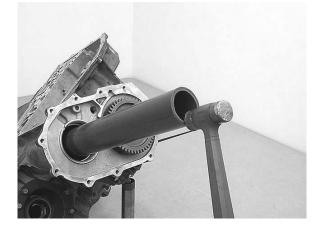
**Step 44:** Install the snap ring into the case using the special pliers designed for this purpose. If the snap ring doesn't want to pop into the ring groove on its own, you may want to help it a little bit by removing the special pliers and giving the ring a gentle pop or two with the PVC pipe and a modest sledgehammer. After the snap ring is in position, gently pry up on the bottom of the transfer gear through the differential area to push the lower bearing race against the snap ring.
