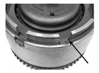
Step 37: Install the reverse clutches in the input clutch drum.
