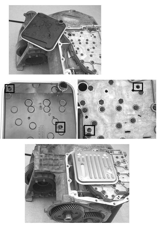
**Step 56:** Do not use any pan gaskets on this unit. Run a 1/8" bead of RTV all the way around the oil pan, rear cover and differential cover. Avoid gaps or narrow spots in the silicone bead that might not allow a complete seal. Make certain that the bottom pan magnet is cleaned and in the proper position, then lay the pans in place, and start the bolts. Torque the pan bolts to 14 ft-lbs.
