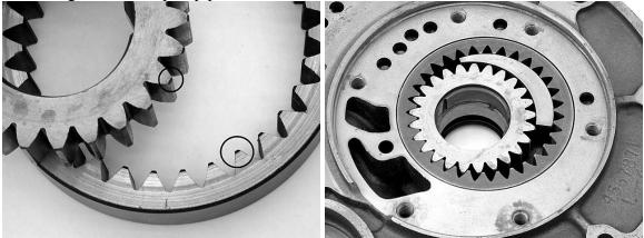
**Step 11.** Lower the stator support onto the pump body, properly aligning the passages and bolt holes. Hand tighten the six pump bolts.
