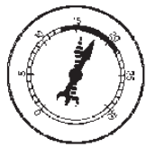
POOR VALVE SEATING AT IDLE
