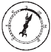
POOR VALVE SEATING AT IDLE
