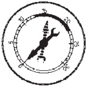
RESTRICTED EXHAUST (DROPS TOWARD ZERO AS ENGINE RPM INCREASES)
