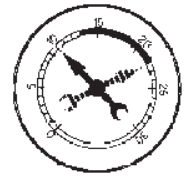
WORN VALVE SPRINGS (MORE PRONOUNCED AS ENGINE SPEED INCREASES)
