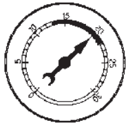
NORMAL READING RANGE AT IDLE
