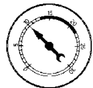
LATE VALVE TIMING, VACUUM LEAK AT IDLE
