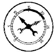
WORN VALVE SPRINGS (MORE PRONOUNCED AS ENGINE SPEED INCREASES)
