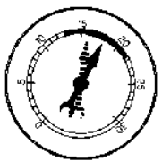
POOR VALVE SEATING AT IDLE
