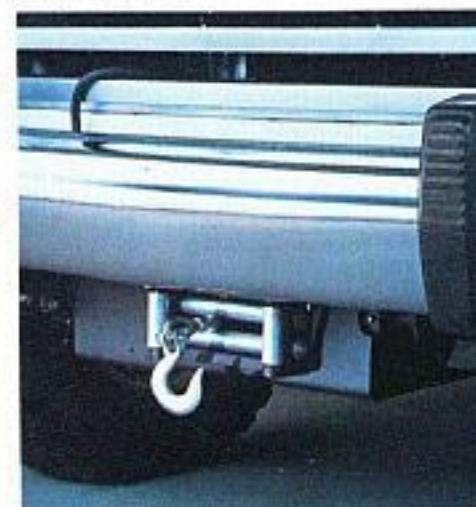
Hidden winch—dealer installed
