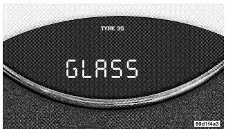
If any other active warnings including "door" or "LO-WASH" are present, they will be shown in the VF display and will also continue to cycle. If the vehicle is moving, two single chimes will occur if the rear glass is open or three single chimes will occur if the rear swing gate is open (one chime for each complete display cycle). After this, the VF display will continue to sequence only (no chimes).
