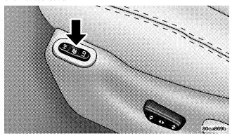
Once the heated seat switch is activated, depressing it a second time will de-activate it.
