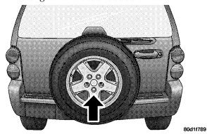
**NOTE:** If you have added aftermarket accessories to the spare tire mounted carrier, it cannot exceed a gross weight of 50 lbs (23 kg) including the weight of the spare
