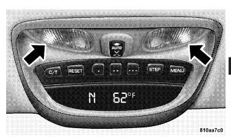
The dome/reading lights illuminate when a door or the swing gate is opened or when the interior lights are turned on by rotating the dimmer control located on the multi-function lever.
