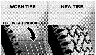
Overloading your vehicle, long trips in very hot weather, and driving on bad roads may result in greater wear.
