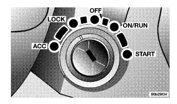
To remove the ignition key on models with an automatic transmission, place the gearshift lever in P (Park), turn the ignition key to LOCK and remove the key.
