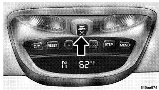
Press and hold the "V" button in the center of the sunroof switch to open the vent. The sunroof can be stopped at any position between closed and full vent. To close the sunroof from the vent position, press and hold the switch forward. Releasing the switch will stop the movement of the sunroof and the sunroof will remain in the partial vent position until the switch is pushed forward again.
