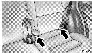
In addition, there are tether strap anchorages behind each rear seating position located on the back of the seat.
