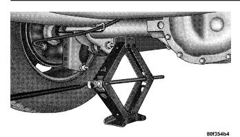
**Rear Scissor Jack Location** 5. Raise the vehicle by turning the jack handle clockwise until the tire clears the ground.
