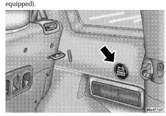
The rear power outlet is a direct feed from the battery so it receives power whether the ignition is in the ON or OFF position.
