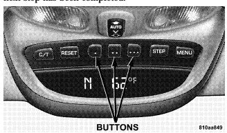
3. When the message TRAINED appears on the HomeLink display, release both the HomeLink and handheld transmitter buttons.
