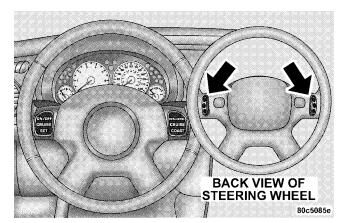
The right hand control is a rocker type switch with a push-button in the center and controls the volume and mode of the sound system. Pressing the top of the rocker switch will increase the volume and pressing the bottom of the rocker switch will decrease the volume.
