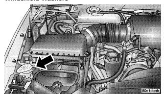
The fluid reservoir for the windshield washers and the rear window washer is shared. It is located in the front of the engine compartment on the passenger side and should be checked for fluid level at regular intervals. Fill the reservoir with windshield washer solvent (not radiator antifreeze) and operate the system for a few seconds to flush out the residual water.
