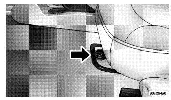
Using body pressure, move forward and rearward on the seat to be sure the seat adjusters have latched.
