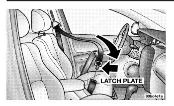
3. When the belt is long enough to fit, insert the latch plate into the buckle until you hear a "click."  $\,$
