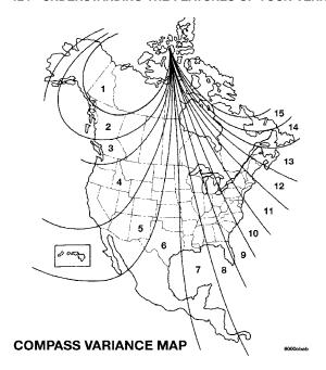
To set the variance: Turn the ignition ON and set the display to "Compass/Temperature." Press and hold the RESET button five seconds (no more than 10 seconds). The last variance zone number will be displayed. Press the STEP button to select the new variance zone and press the RESET button to resume normal operation.
