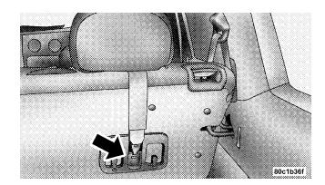
An incorrectly anchored tether strap could lead to increased head motion and possible injury to the child. Use only the anchor positions directly behind the child seat to secure a child restraint top tether strap.
