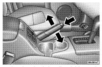
To release the parking brake, pull up slightly, press the center button, then lower the lever completely.
