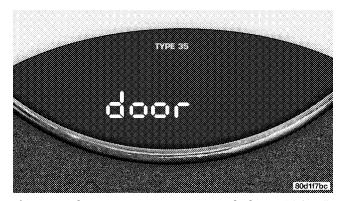
If any other active warnings including "GATE", "GLASS", or "LOWASH" are present, they will be shown in the VF display and will also continue to cycle. If the vehicle is moving, three single chimes will occur (One chime for each complete display cycle (three cycles total). After this, the display will continue to cycle only (no chimes).
