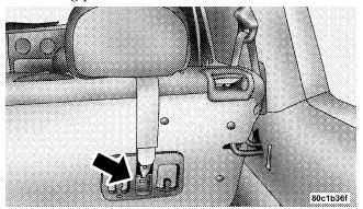
Many, but not all restraint systems will be equipped with separate straps on each side, with each having a hook or connector for attachment to the lower anchorage and a means of adjusting the tension in the strap. Forwardfacing toddler restraints and some rear-facing infant restraints will also be equipped with a tether strap, a hook for attachment to the tether strap anchorage and a means of adjusting the tension of the strap.
