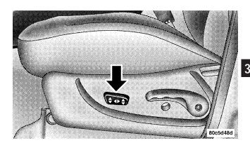
This seat also has a manual recline lever located just to the rear of the power seat switch. Pull up on the lever to recline the seat.
