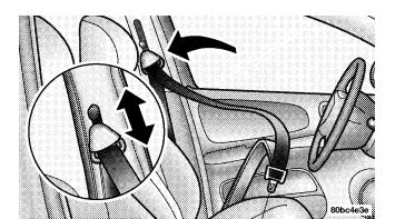
Position the shoulder belt height adjusters so that the belt rests across the middle of your shoulder. Failure to adjust the safety belt properly could reduce the effectiveness of the seat belt and increase the risk of injury in a collision.
