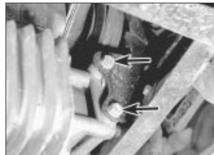
5.5 Left-hand mounting bracket attachment bolts (arrowed) on later manual transmission models
