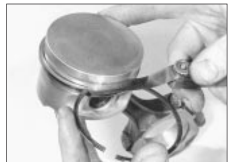
11.17 Measuring the piston ring-to-groove clearance
