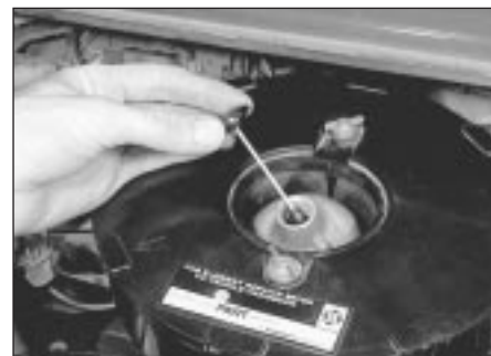
19.4 Top up the piston damper on carburettor models
