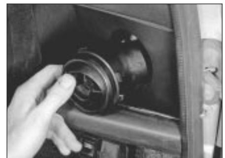
13.2 Turn the air vent anti-clockwise to remove
