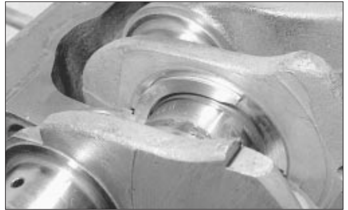
17.19 Refitting the crankshaft thrustwasher upper halves
