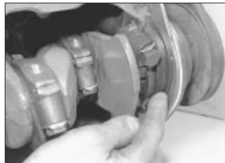
5.25 Fitting a new front oil seal . . .
