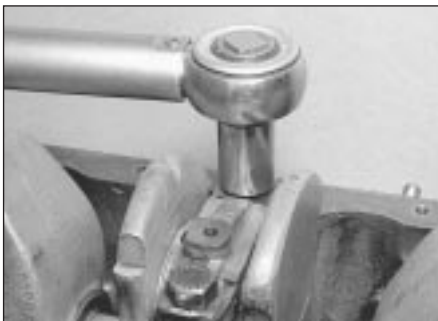
17.22 Tighten the main bearing cap bolts to the specified torque
