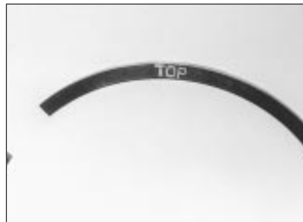
16.3 Piston ring identification markings
