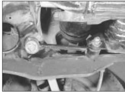
12.30 Lower engine tie-bar attachments
