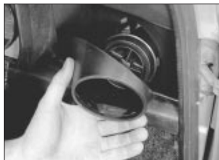
13.1b ... and lift away the binnacle
