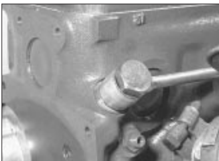
15.2a Oil feed pipe banjo union at the engine . . .
