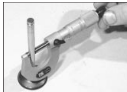
8.17 Measuring the valve stem diameter
