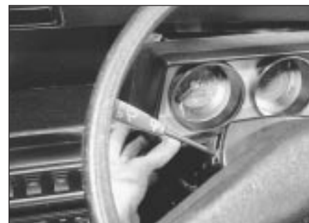
15.25 Remove the instrument cluster nacelle
