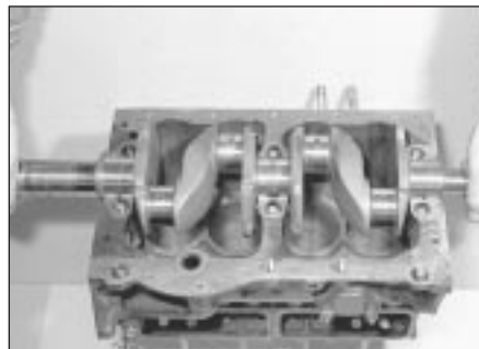
12.10 Carefully lift out the crankshaft
