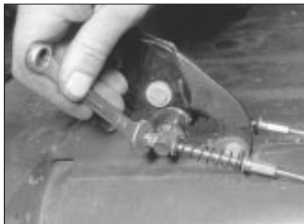
21.3 Remove the handbrake cable adjusting nuts
