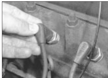
33.5 Pull the leads off the spark plugs by gripping the rubber boot
