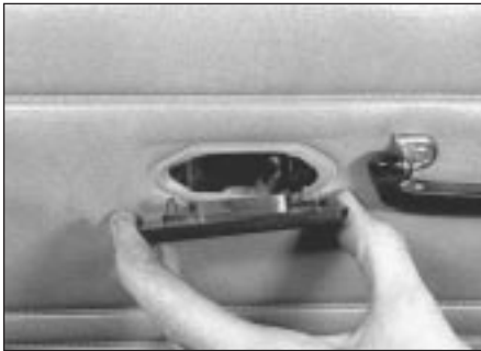
6.3 Ease off the interior lock control surround . . .
