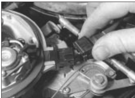
13.12 Disconnecting the injector housing wiring connector
