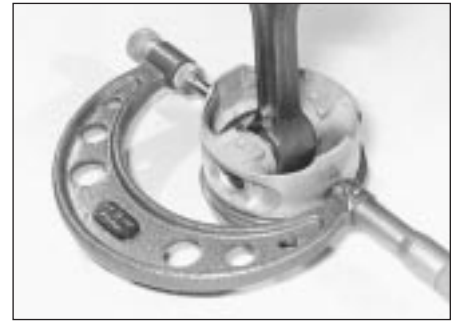
11.16 Measuring the piston diameter
