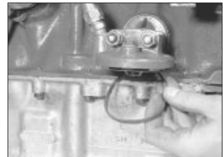
13.12 Fitting a new cartridge type oil filter sealing ring
