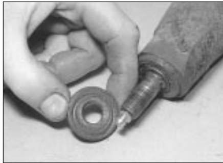
19.12b . . . and thrustwasher . . .
