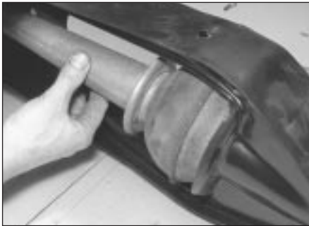
15.3 Remove the rear rubber cone spring strut . . .
