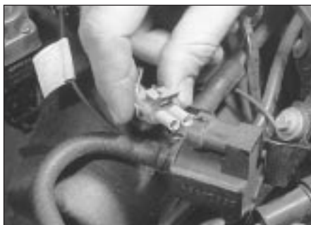
6.28 Disconnecting the purge valve wiring connector
