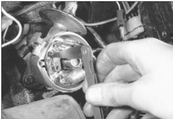
5.6d Using feeler blades to check the contact breaker points gap
