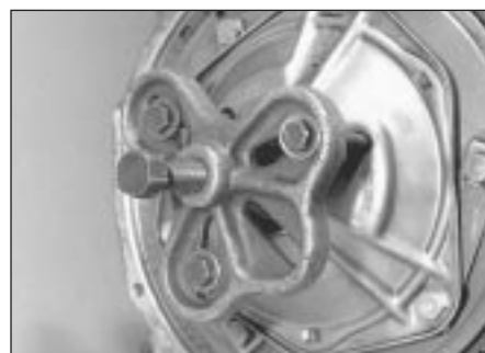
5.9 Using a commercially available puller to release the flywheel taper
