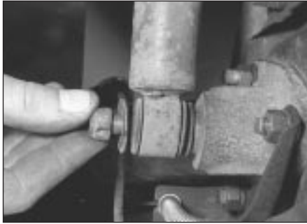
17.3 Remove the shock absorber lower . . .
