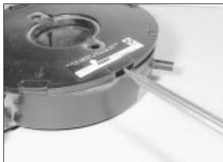
30.6a Prise off the later type air cleaner moulded plastic cover . . .
