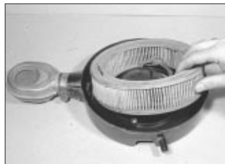
30.6b . . . and lift out the element
