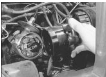
5.1 Removing the distributor cap
