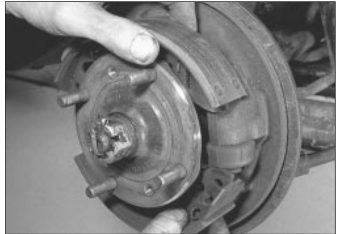
5.4b . . . and then from the piston end
