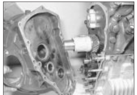
5.35 Refitting the flywheel housing
