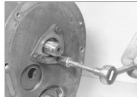
9.3 Undo the camshaft locating plate bolts and lift off the plate
