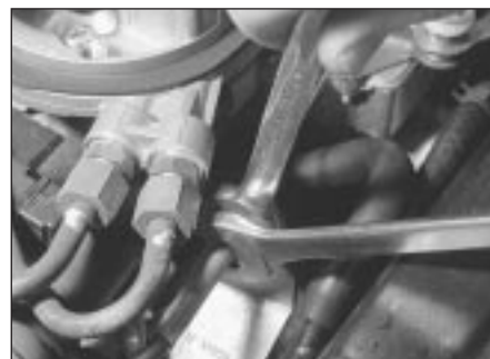
4.10 . . . then adjust the locknut and adjuster nut as described in text
