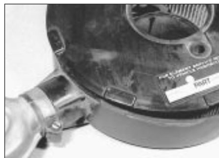
30.8 Make sure the alignment arrow is toward the lug on the air cleaner body
