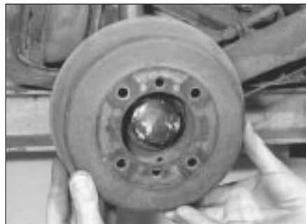
4.3 . . . and withdraw the drum
