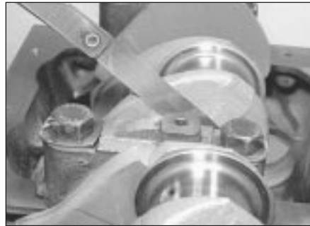
12.3 Checking crankshaft endfloat using feeler blades
