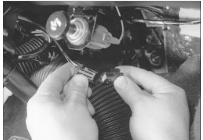
13.47 Disconnect the wiring connector . . .
