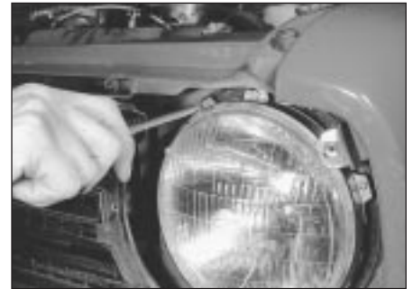
5.4a Unscrew the inner rim securing screws . . .
