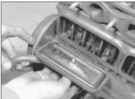
9.1 Removing the tappet side covers
