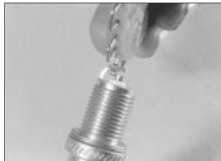
33.11 Adjusting a spark plug electrode gap
