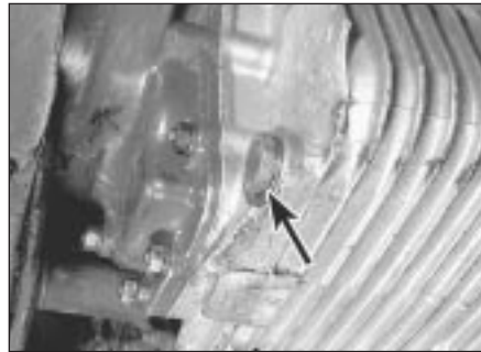
13.3 Engine/transmission oil drain plug (arrowed)
