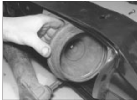
15.4 . . . and rubber cone spring
