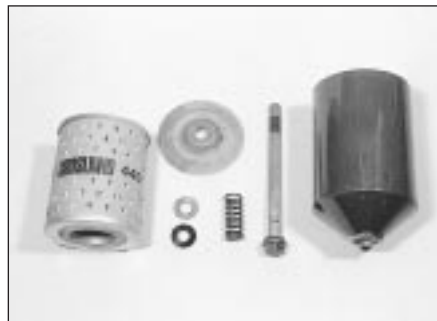
13.9 Components of the cartridge type oil filter
