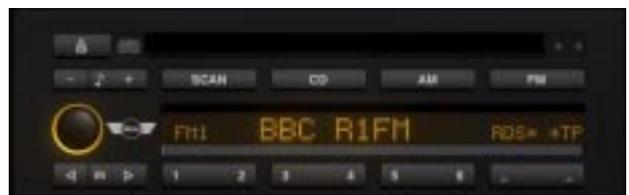
**NOTE:** If an incorrect code is entered three consecutive times, a delay period of 1 hour commences, during this delay period 'WAIT' appears in the display. **DO NOT** switch radio off (leave ignition switched to position 1), at the end of the delay period, 'CODE' reappears in the display and the correct code can be entered.
