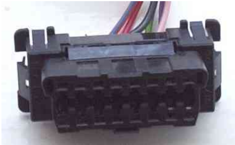
16-pin diagnostics socket
