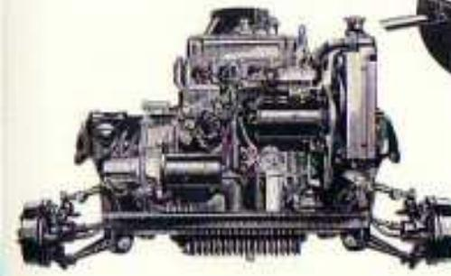
Almost all the mechanical parts of a Mini-Moke are embodied in the amazing unit shown left. Only 10 inches of the total length of the vehicle are taken up by engine, clutch, gears, differential,
