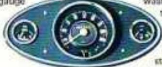
The two smaller dials show water temperature and engine oil pressure. There are warning lights for ignition, oil filter renewal and headlamp main beam. Windscreen washer is fitted and toggle switches control the lights. The key operates the starter.
