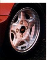
Giving an edge to that legendary bandling, the Cabriolet is fitted with 'Revolution' alloy wheels with 175/50 x 12 low profile tyres.
