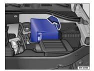
Fig. 164 In the engine compartment: Open the sleeve covering of the vehicle battery.
