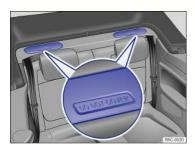
Fig. 42 Behind the rear bench seat backrest: Automatic Rollover Support System.
