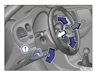
Fig. 49 Manual adjustment for the steering wheel position.
