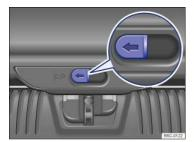
Fig. 175 Inside the luggage compartment: Opening the trunk lid.
