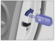
Fig. 171 On the edge of the passenger door: Manually locking the door with the vehicle key.
