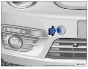
Fig. 197 In the right front bumper: Removing the cover.
