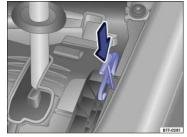
Fig. 179 Releasing the selector lever lock.
