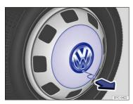
Fig. 187 Pulling the wheel cover off (Version 2).
