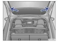
Fig. 103 On the trunk lid: Installing and removing the supporting cords.
