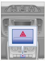
Fig. 169 In the center of the instrument panel: Button for the emergency flashers.
