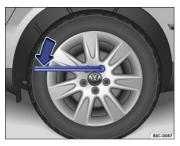
Fig. 188 Changing a wheel: Loosening the wheel bolts.
