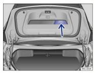
Fig. 34 Opened trunk lid: Recessed grip for closing (Beetle Convertible models).
