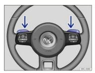
Fig. 135 Steering wheel with Tiptronic shift paddles (if equipped).
