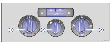
Fig. 153 In the center console: Manual air conditioning controls.
