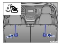
Fig. 80 Anchorages for the top tether strap on the back of the rear seat.
