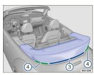
Fig. 41 With the convertible top open: Installing the rear of the convertible top cover (boot).
