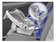
Fig. 75 Rearward-facing infant seat properly installed on the rear seat.
