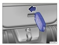
Fig. 172 Inside the luggage compartment: Opening the trunk lid.
