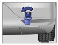
Fig. 200 In the right rear bumper: Installing the towing eye.
