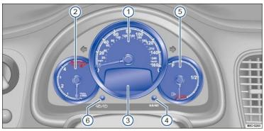
Fig. 12 Instrument cluster in the instrument panel.
