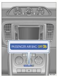
Fig. 66 In the instrument panel: PASSENGER AIR BAG light.
