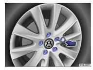
Fig. 185 Pulling cover caps off wheel bolts.
