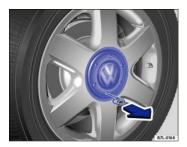
Fig. 183 Pulling the hubcap off.
