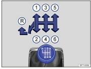
Fig. 132 Gearshift pattern of a 6-speed manual transmission.
