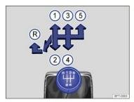
Fig. 131 Gearshift pattern of a 5-speed manual transmission.
