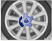
Fig. 184 Twisting the hubcap off.
