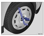
Fig. 186 Pulling the wheel cover off (Version 1).
