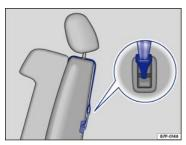
Fig. 79 Example of a mounted upper tether strap: The top tether strap reduces the forward movement of the child restraint in a crash, to help reduce the risk of head injury if the child hits the vehicle interior.
