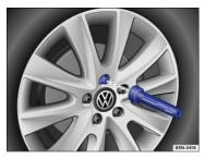
Fig. 191 Changing a wheel: Remove previously loosened wheel bolts using the screwdriver handle.
