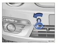
Fig. 198 In the right front bumper: Installing the towing eye.
