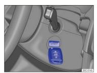
Fig. 128 Hold the remote control vehicle key to the right of the steering column: Emergency starting feature.
