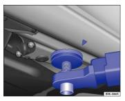
Fig. 168 Rear lift point for workshop hoist or floor jack.
