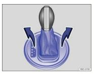
Fig. 178 Removing the selector gate cover.
