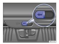
Fig. 66 Inside the luggage compartment: Opening the trunk lid.
