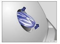
Fig. 60 Opening the trunk lid from the outside.
