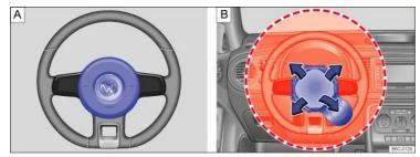
Fig. 33 Location and deployment zone of the driver front airbag.
