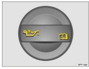
Fig. 170 In the engine compartment: Engine oil filler cap (cap design may vary depending on vehicle equipment).
