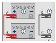
Fig. 161 Diagram for attaching the jumper cables: Dead battery ① and booster battery ②.
