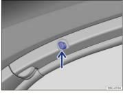
Fig. 136 On the sides of the convertible top frame: Coat hooks.
