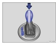
Fig. 110 Automatic transmission selector lever with shift lever release button (arrow).
