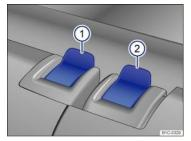
Fig. 81 Rear seat: release button right backrest ①, left backrest ②.
