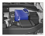
Fig. 174 In the engine compartment: Open the sleeve covering of the vehicle battery.
