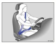
Fig. 29 Proper safety belt positioning for expectant mothers.
