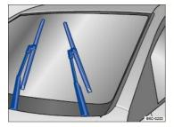
Fig. 155 Windshield wiper in service position.
