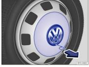
Fig. 185 Pulling the wheel cover off (Version 2).
