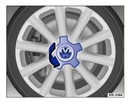
Fig. 182 Twisting the hubcap off.
