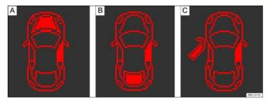
Fig. 14 In the instrument cluster display (examples): : Open engine hood, : Open trunk lid, : Open driver door.
