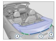
Fig. 74 With the convertible top open: Installing the rear of the convertible top cover (boot).
