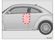
Fig. 35 Deployment zone of the side airbag.
