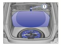
Fig. 152 In the luggage compartment: Floor covering raised and ① secured (Beetle Coupe models).
