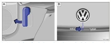
Fig. 166 : In the footwell on the driver side: Inside engine hood release lever. : Above the radiator grille: Outside engine hood release.
