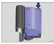
Fig. 158 In the engine compartment: Fuse box cover.
