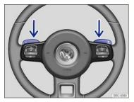
Fig. 112 Steering wheel with Tiptronic shift paddles (if equipped).
