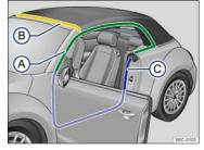
Fig. 151 Caring for rubber seals: Seals on the side windows (A), the roof seal (B), and door seals (C).
