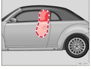
Fig. 38 Deployment zone of the side airbags.
