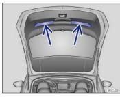
Fig. 61 Opened trunk lid: Recessed grips for closing (Beetle Coupe models).
