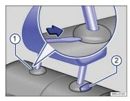
Fig. 86 Removing the rear head restraints.
