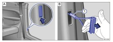
Fig. 64 In the bottom of the driver door pillar: Emergency release cover.
