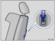
Fig. 48 Example of a mounted upper tether strap: The top tether strap reduces the forward movement of the child restraint in a crash, to help reduce the risk of head injury if the child hits the vehicle interior.
