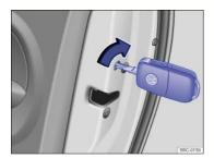
Fig. 58 On the edge of the passenger door: Manually locking the door with the vehicle key.
