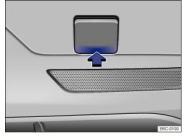
Fig. 164 In the right rear bumper: Removing the cover.
