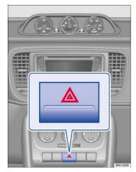
Fig. 50 In the center of the instrument panel: Button for the emergency flashers.
