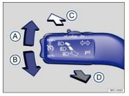
Fig. 89 On the left side of the steering column: Turn signal lever and high beam switch.
