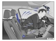
Fig. 23 The unbelted driver is thrown forward.
