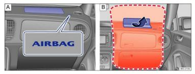
Fig. 34 Location and deployment zone of the front passenger front airbag.
