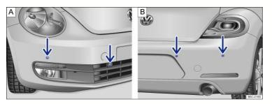
Fig. 122 In the front and rear bumpers: Park Distance Control system sensors.
