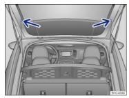
Fig. 145 On the trunk lid: Installing and removing the supporting cords.
