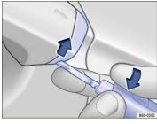
Fig. 57 Door handle on driver door: Removing the lock cylinder cover.
