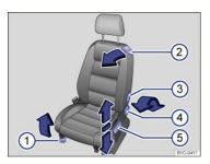
Fig. 80 Driver seat: Manual seat adjustment controls.
