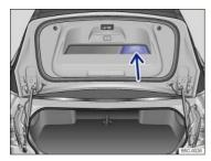
Fig. 62 Opened trunk lid: Recessed grip for closing (Beetle Convertible models).
