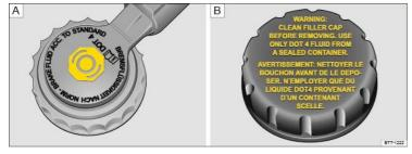
Fig. 173 In the engine compartment: Brake fluid reservoir cap (cap design may vary depending on vehicle equipment).
