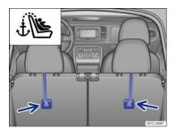
Fig. 47 Anchorages for the top tether strap on the back of the rear seat.
