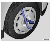
Fig. 184 Pulling the wheel cover off (Version 1).
