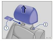
Fig. 85 Removing the front head restraints.
