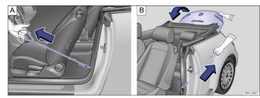
Fig. 65 In the bottom of the driver door pillar: Trunk lid emergency release.
