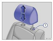
Fig. 84 Adjusting the head restraints.
