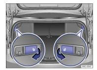
Fig. 83 In the luggage compartment: Release lever for the left and right sections of the rear seat backrest.
