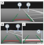
Fig. 128 On the screen: Orientation lines for the parking space behind the vehicle. : Searching for a parking space, : Backing into the parking space, : Maneuvering.
