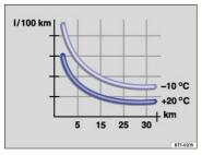
Fig. 106 Fuel consumption in I/100 km at 2 different outside air temperatures.
