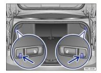
Fig. 148 In the luggage compartment: Shopping bag hooks (Beetle Convertible models).
