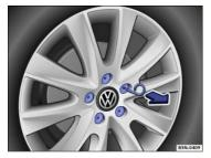
Fig. 183 Pulling cover caps off wheel bolts.
