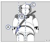
Fig. 31 Positioning of the safety belt extender.
