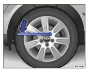
Fig. 186 Changing a wheel: Loosening the wheel bolts.
