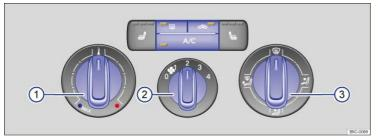
Fig. 101 In the center console: Manual air conditioning controls.
