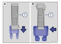
Fig. 160 Removing or installing a blade fuse with the plastic tweezers: : MINI. : ATO.
