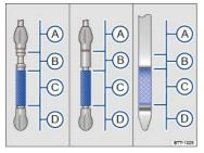
Fig. 169 Engine oil dipstick with oil level marks.
