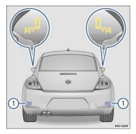
Fig. 116 In the outside mirrors: Indicator lights for the Blind Spot Monitor.
