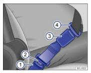
Fig. 30 A safety belt extender properly attached to the factory-installed safety belt.
