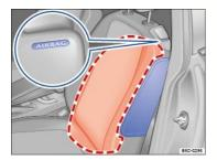
Fig. 36 In the padding on the outboard side of the front seat backrests (Beetle Coupe): Location and deployment zone of the side airbags.
