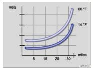
Fig. 105 Fuel consumption in miles per gallon (mpg) at 2 different outside air temperatures.
