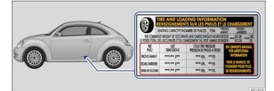
Fig. 177 On the driver door jamb: Location of the tire inflation pressure label.
