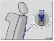
Fig. 46 Example of a mounted upper tether strap: The top tether strap reduces the forward movement of the child restraint in a crash, to help reduce the risk of head injury if the child hits the vehicle interior.
