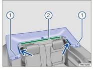
Fig. 73 With the convertible top open: Installing the front of the convertible top cover (boot).
