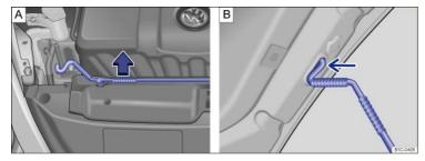
Fig. 167 : In the engine compartment: Bracket for hood support. : Hood propped open.
