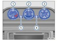
Fig. 13 Above the center console: Engine oil temperature gauge ①, stopwatch ②, and boost pressure gauge ③.
