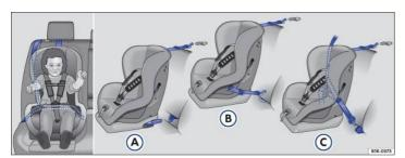
Fig. 43 Some child restraints have lower anchors and a top tether. Figures (A) and (B) show how to correctly install a LATCH/UCRA seat. Figure (C) shows the set up of a seat using the vehicle's safety belt system.
