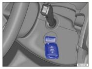
Fig. 109 Hold the remote control vehicle key to the right of the steering column: Emergency starting feature.
