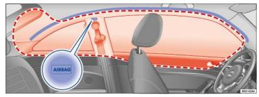
Fig. 39 On the left vehicle side: Installation location and deployment zone of the Side Curtain Protection airbag (Beetle Coupe only).
