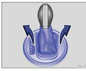
Fig. 113 Removing the selector gate cover.
