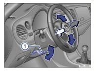
Fig. 78 Manual adjustment for the steering wheel position.
