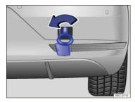
Fig. 165 In the right rear bumper: Installing the towing eye.
