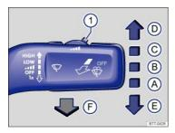
Fig. 93 Operating the front windshield wipers.
