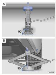
Fig. 190 Jack in position at the left rear lift point.
