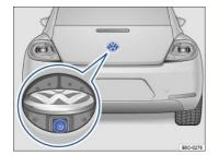
Fig. 126 In the trunk lid: Location of the camera.
