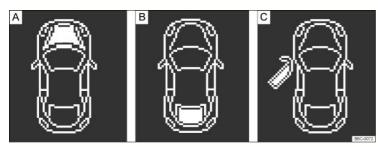
Fig. 15 In the instrument cluster display: : Open engine hood, : Open trunk lid, : Open driver door.
