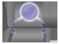
Fig. 45 Markings for the LATCH/UCRA lower universal anchorages on the seat.
