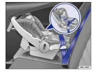
Fig. 42 Rearward-facing infant seat properly installed on the rear seat.
