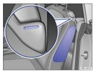
Fig. 37 In the padding on the outboard side of the front seat backrests (Beetle Convertible): Location of the side airbags.
