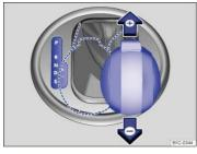
Fig. 111 Selector lever in Tiptronic position.
