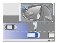
Fig. 117 Driving situation when passing with traffic behind your vehicle. Arrow: Blind Spot Monitor indicator light in the driver side mirror.
