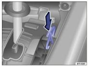
Fig. 114 Releasing the selector lever lock.
