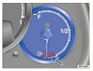
Fig. 16 In the instrument cluster: Fuel gauge.
