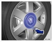
Fig. 181 Pulling the hubcap off.
