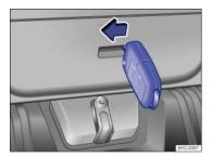
Fig. 63 Inside the luggage compartment: Opening the trunk lid.
