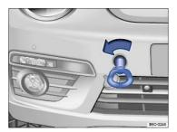
Fig. 151 In the front bumper on the right side: Installing the towing eye.
