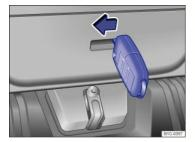
Fig. 58 Inside the luggage compartment: Opening the trunk lid.
