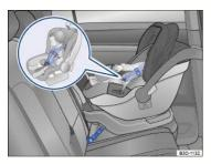
Fig. 37 Example of a rearward-facing infant seat properly installed on the rear seat.
