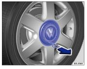
Fig. 169 Pulling the hubcap off.
