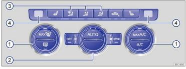
Fig. 96 In the center console: Climatronic controls.
