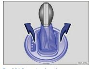
Fig. 106 Removing the selector gate cover.
