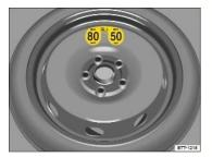
Fig. 167 In the luggage compartment: Compact spare wheel (label design may vary).
