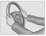
Fig. 74 Steering wheel: 9 o'clock and 3 o'clock positions.
