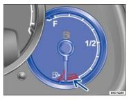
Fig. 14 In the instrument cluster: Fuel gauge.
