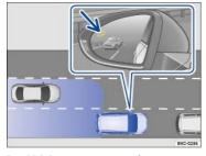
Fig. 110 Driving situation when passing with traffic behind your vehicle. Arrow: Blind Spot Monitor indicator light in the driver side mirror.
