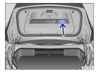
Fig. 57 Opened trunk lid: Recessed grip for closing (Beetle Convertible models).
