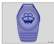
Fig. 156 In the engine compartment: Cap of the windshield washer fluid reservoir.
