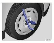
Fig. 172 Pulling the wheel cover off (Version 1).
