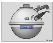
Fig. 159 Coolant expansion tank in the engine compartment.
