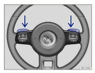
Fig. 105 Steering wheel with Tiptronic shift paddles (if equipped).
