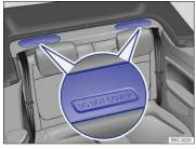
Fig. 70 Behind the rear bench seat backrest: Automatic Rollover Support System.
