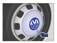
Fig. 173 Pulling the wheel cover off (Version 2).
