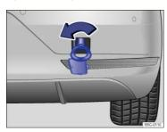
Fig. 153 In the right rear bumper: Installing the towing eye.
