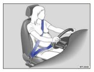
Fig. 26 Proper safety belt positioning for expectant mothers.
