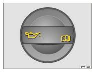
Fig. 158 In the engine compartment: Engine oil filler cap (cap design may vary depending on vehicle equipment).
