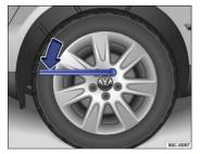
Fig. 174 Changing a wheel: Loosening the wheel bolts.
