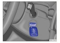
Fig. 102 Hold the remote control vehicle key to the right of the steering column: Emergency starting feature.
