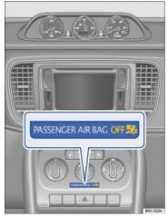
Fig. 27 In the instrument panel: PASSENGER AIR BAG light.
