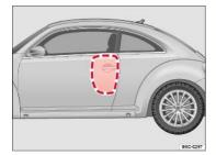
Fig. 30 Deployment zone of the side airbag.
