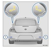
Fig. 109 In the outside mirrors: Indicator lights for the Blind Spot Monitor.
