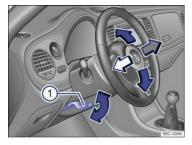
Fig. 73 Manual adjustment for the steering wheel position.
