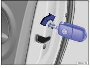
Fig. 53 On the edge of the passenger door: Manually locking the door with the vehicle key.
