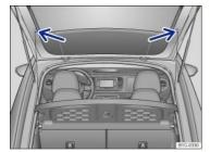
Fig. 133 On the trunk lid: Installing and removing the supporting cords.
