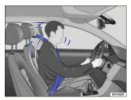
Fig. 22 Belted driver secured by the correctly worn safety belt in the event of a sudden braking maneuver.
