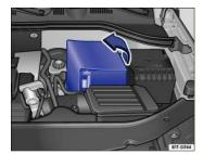
Fig. 162 In the engine compartment: Open the sleeve covering of the vehicle battery.
