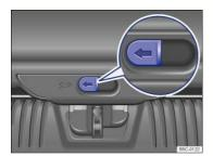
Fig. 61 Inside the luggage compartment: Opening the trunk lid.
