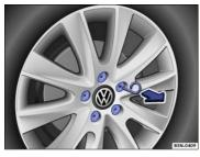
Fig. 171 Pulling cover caps off wheel bolts.
