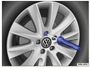
Fig. 179 Changing a wheel: Remove previously loosened wheel bolts using the screwdriver handle.
