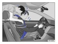
Fig. 21 Unbelted passengers in the rear seats are thrown forward on top of the belted driver.
