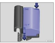
Fig. 146 In the engine compartment: Fuse box cover.
