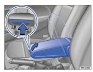
Fig. 124 In the front center armrest: Storage compartment (if equipped).
