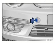
Fig. 150 In the front bumper on the right side: Removing the cover.
